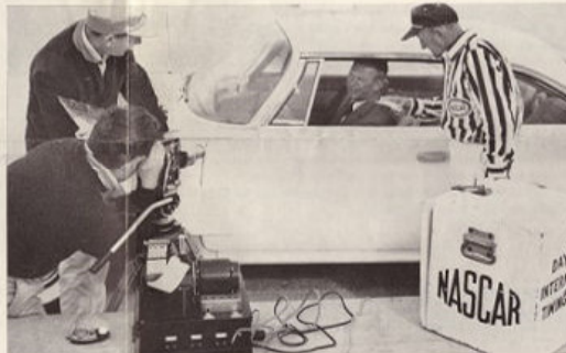
GETTING THE TIME—A NASCAR official heads Brewster Shaw the time for one of his acceleration runs while camera grinds away. Shaw made the unofficial test runs to see how the 300-F handles and performs.
