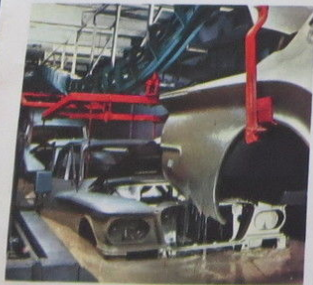
7-coat rust protection helps your car keep its good looks — and its high resale value. Car bodies are soaked seven times to protect the metal from rust inside and out.
