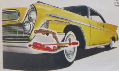
The principle of torsion bar suspension
