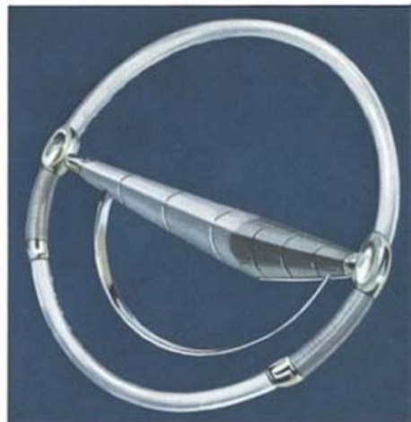
THE NEW SAFETY steering wheel features a deeply recessed spoke that is leather covered and heavily padded with sponge rubber. Convenient hand grips and chrome thumb rests are included.
