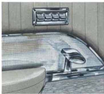
ILLUSTRATED ABOVE is a section of the left front door panel showing the new door handle, built-in arm rest, and the electric window lift control panel that operates all four windows.
