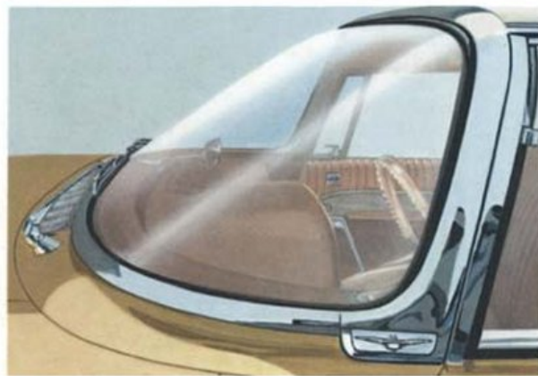
THE NEW "double wrap-around" windshield has 54% more glass area, which increases visibility in virtually all directions—a great safety feature.
