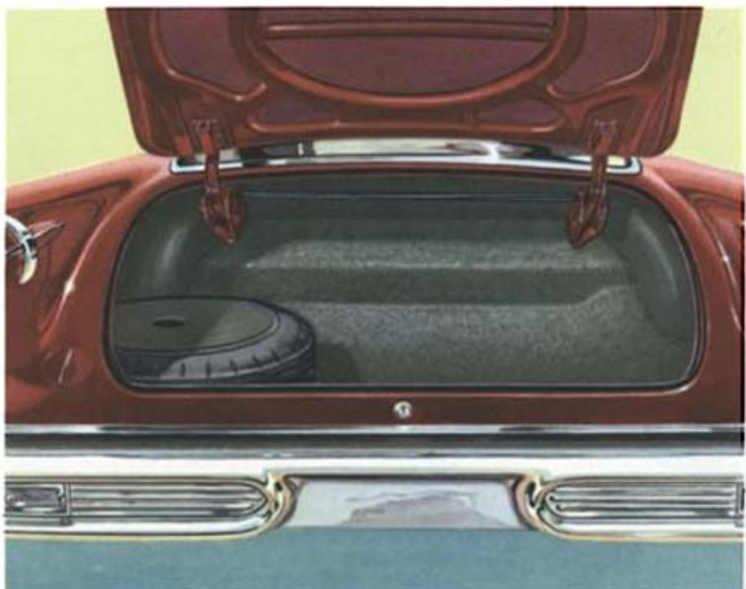
THE REAR DECK has large storage space. The spare tire is mounted flush with the floor and has a carpet cover to protect luggage. The floor has a rich gray carpeting. And the torsion bar hinges make opening and closing of the deck lid an easy matter. Compartment is automatically lighted when lid is opened.
