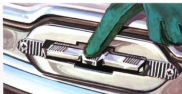
6-Way Electric Power Front Seat lets you choose your favorite position quick-as-a-wink and change it as often as you like. Just touch this control and your seat tilts for relaxing comfort — as well as adjusting up-down, forward-back.
