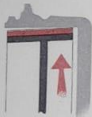
End view of ordinary off-center shoe twisting under braking pressure.
