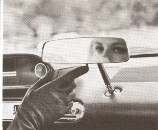
PRISMATIC REAR-VIEW MIRROR A flick of the base tab cuts the headlight glare from the cars behind to a minimum.
