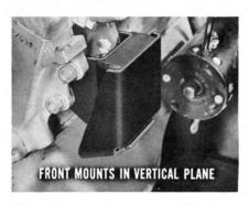
through the rubber in a direction parallel to the plates—in other words, in *shear*. In fact, they're called "shear-type" mountings. They're especially good at damping out engine low-speed vibration effects. They isolate from the frame and body the rocking motion induced in the engine by torque impulses, particularly while the engine is idling,
