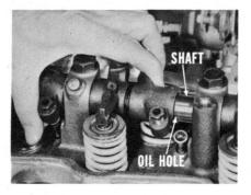
Oil is forced through the rocker arm shaft and through a small hole in the shaft to the clearance between the shaft and rocker arm. Oil that squeezes out at that point drains back to the crankcase through return holes drilled in the bottom corners of each cylinder head.
