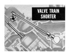
But on the new Plymouth engine, the valve train is 3" to 4" shorter in length. Valve stems and push rods are shorter. Besides that, there's a different size block, and an entirely new valve-train geometry.
