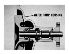
always coat the attaching screws with a good sealer that is not soluble in water. That's because these screws extend into the water passage. Two studs are used, in addition to the screws. It will seldom be necessary to remove these studs. However, if it should be necessary, be sure to seal the threads when installing the studs in the block.
