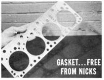
tightening sequence. First, snug down the bolts to about 40 foot-pounds in proper sequence. Then, go back and tighten the bolts in order to 85 foot-pounds. With the new steel gasket, a third check on cylinder head bolt torque after the engine has warmed ur won't be necessary.
