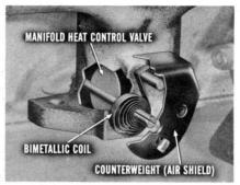
in the right exhaust manifold. A stuck heat control valve will affect the operation of the choke coil, and result in poor choke operation. In short, the manifold heat control valve has a direct effect on the operation of the choke valve. If you suspect the automatic choke of operating improperly,
