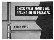
valve and what it does, keep in mind that it really works as a combination check and bypass valve. The check valve, in a vertical passage in the block, admits oil to a horizontal passage. It also acts as a *check* to retain oil in the passages, filter, and gallery when the engine isn't running.
