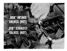
clearances on this new Hy-Fire V-8, 227 cubic-inch engine are .008" on the intake valves, and .018" on the exhaust valves.
