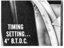
If an owner prefers using premium fuel in a two-barrel carburetor engine, however, you can advance the timing. But don't advance it more than 8° before top dead center! This engine is designed to give standard performance on regular fuel.
