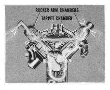
The valve rocker arm chambers and the valve tappet chamber are also ventilated along with the crankcase. So, more of the engine gets ventilated and the entire system keeps engine oil free from contamination caused by condensation and combustion fumes.
