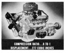
For example, the combustion chamber has been redesigned to
