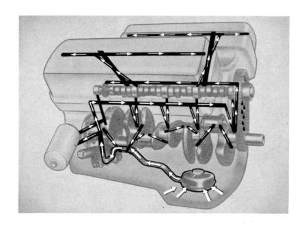
Improvements in engine lubrication are always made to protect engine life and to better the performance when possible. In the case
