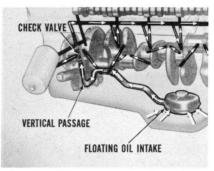
But suppose we trace the oil flow from the time the oil leaves the crankcase. For example, once the oil is drawn into the floating oil intake, it goes into a vertical passage in the block. A ball check valve at this point acts as an oil-flow traffic officer.
