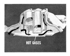
Now, after warm-up, and also during cold operation acceleration or high-speed driving, the heat valve opens. This cuts down exhaust gas flow to the hot spot. Consequently, you get better breathing and greater power output at higher speeds.
