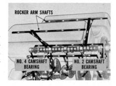
Oil comes up a passage from the #2 camshaft bearing, for instance.
