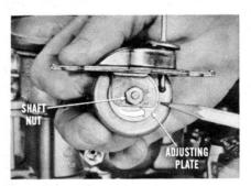
this adjustment, here's how simply it's done. First, loosen the holddown bolts and remove the choke from its pocket in the manifold. Next, loosen the shaft nut. Then, turn the adjusting plate toward "lean," or "rich." You'll find "L" and "R" stamped on the cover.
