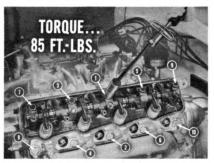
water leaks might show up. So torque the center bolt of the inner row first to 85 footpounds. Then, tighten the center bolt of the outer row. Alternate from the inner to the outer rows, working out to the ends. Remember . . . the *sequence* of tightening is very important!
