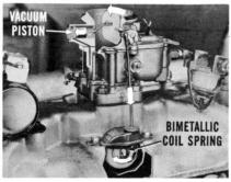
tered air from the carburetor air horn. Failure, due to dirt in the piston passage, is practically eliminated.
