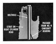
Oil from the #4 camshaft bearing also goes up the same kind of passage. This passage indexes with a cylinder head bolthole on the *right* cylinder head. The bolthole, in this case, is the one going through the rocker arm shaft bracket which is the second bracket from the rear of the engine.
