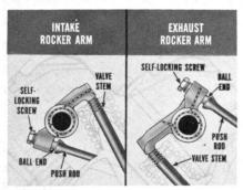
Oil lubricates the ball end of the self-locking screw that fits into the push rod. It also lubricates the valve stem from another passage in the arm. Incidentally, intake and exhaust valve rocker arms are drilled differently to perform both of these two lubricating jobs.
