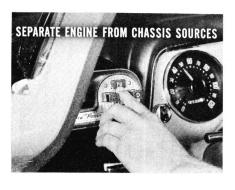
It also pays to see if you can bring in the same condition while the engine is running and car is *standing still*. Just remember to run the engine at the same r.p.m. as the tach showed when the vibration came in while the car was moving.
