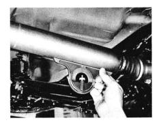
Next, place the protractor on top, or directly below the prop shaft and parallel to it. Adjust the spirit level to center the bubble and take your reading. Add the number of degrees the prop shaft is away from true horizontal, to the first reading. The total will give you the working angle.
