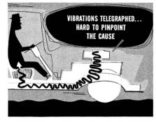
Sympathetic Vibrations. Occasionally there are sympathetic vibrations. This happens when one vibrating part causes another part
