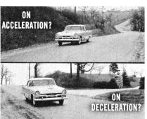
connection. As you road-test the car, get an answer to this question: "Is the condition present while the car is in motion?" At the same time, find out if the condition comes in at any particular car speed, or is present regardless of speed. Use the tachometer and speedometer to relate the condition to engine and car speed.
