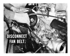
involved. If running with the belt removed didn't bring in the vibration, install a belt that drives only the generator to see if it is the source. A further test would be to remove the fan blades and leave the fan belt in place. If the vibration's gone, it means the fan blades were responsible.
