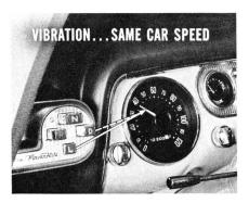
vibration comes in at the same car speed whether the transmission is in low or direct drive, you have a right to suspect the prop shaft. Overspray from undercoating can unbalance a prop shaft. Wrong angularity at the rear joint can make it vibrate, too. If angularity is at fault, it's an easy thing to correct.
