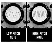
frequency. On an oscilloscope, 16 cycles per second would make a picture of a very low-pitched note. At the other end of the scale, some people can hear vibrations up to about 15,000 cycles per second. This is a very high-pitched note. The faster the frequency, the higher the note.
