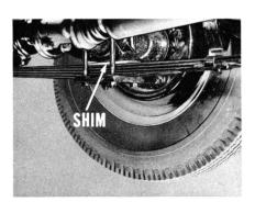
If the total angle exceeds 7°, install a shim between the rear spring and the spring saddle on the axle housing. Try to bring the angle as close to 6° as possible. Install the shim with the flat side to the spring, and the thick portion toward the front of the car to tilt the rear axle carrier upward. Be sure the shim surface is free from burrs.
