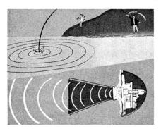
sound you can hear. All sounds, in fact, are the result of vibrations. Most of you know what happens when a pebble is tossed into a pond. Waves are set up. That's how sound acts, too. The vibrating diaphragm of an auto horn, for example, sets up sound waves and you can hear the horn.
