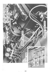
Next, remove the protective caps from both the discharge and suction service ports on the condenser and compressor. Install the 4' test hose from the 600-lb. (right-hand) gauge of the manifold gauge set to the discharge service valve port. Install the 4' hose from the 300-lb. (left-hand) gauge of the gauge set to the suction service valve port. Now, turn both service valve stems two turns clockwise.
