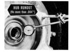
Usually, you'll heat a spot about ½" in diameter until it is a dull red. Next, quench the area quickly with wet rags to shrink the hub back into line. Recheck hub runout with the dial indicator when the converter returns to a uniform room temperature.
