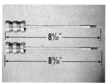
has been forced out of its groove at the upper end of the upper piston rod, chances are that the valve rod is too short. So, check the length of the rod. The short rod is 811/32"; the long rod is 815/32" long. If necessary, replace the piston valve and rod assembly to correct this condition.
