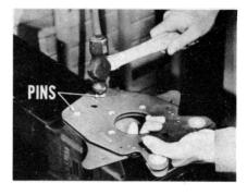
If the pins are loose, remove the support plate from the dust shield. Rest the pin on an anvil, and peen the end until the pin is tight. Be sure that both support plates are in good alignment.
