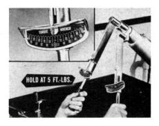
Then, retighten the adjusting nut *clockwise* to 5 *inch-pounds*. Finally, stake the nut to index with the slot in the worm shaft.
