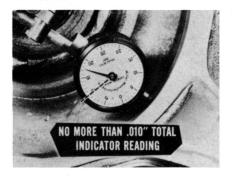
your readings. There should be no more than .010" total indicator reading. If it is more . . . say about .018" total reading, you'll have to shift the housing on the adapter plate in a direction opposite the point you noticed the maximum runout indication. Shifting the housing is done by first replacing the two steel dowels.
