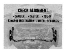
Front wheel alignment, naturally, has to be right. So, check camber, caster, toe-in, kingpin inclination, and front wheel bearing adjustment. Get all these points up to specifications for the car you're working on.
