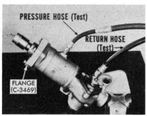
on the mating surface of the lower housing after the upper housing is removed. Next, you remove the worm connector assembly. Connect the test pressure and return hoses to the pump. With a cloth, wipe any traces of oil from the housing and upper piston rod.
