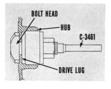
With a wrench, hold the flat end of the fixture bolt and tighten the nut. Then, mount the indicator on end of the bolt. Set the dial anvil so it bears on the transmission pilot bore of the converter housing. Then, turn the converter a full turn two or three times and take
