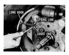
Put the long hook of the return spring in the shoe, and the shorter end in the spring link. Next, install the original brake shoe guide springs and retainers. Install the wheel and drum, and road-test the job.
