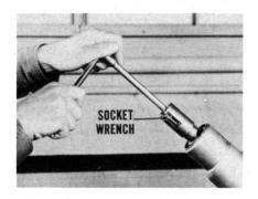
Check the steering worm coupling screw next. If it had worked loose, there would be too much backlash in the tube and coupling. In this case all you have to do is use a socket wrench and make sure the screw is snugged down good and tight.
