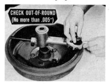
than .005". If they are, true them up on a lathe, and polish out any roughness. Always polish the drums if there's any roughness due to scoring, flat spots or a threading design. Use a piece of No. 60 or No. 80 grit emery cloth, and finish with a No. 200, or finer emery cloth.
