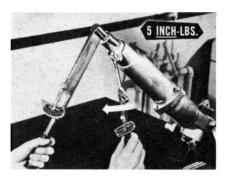
Worm Shaft End Play in Connector—If you find too much worm shaft end play in the connector assembly, replace the worm and connector as an assembly.
