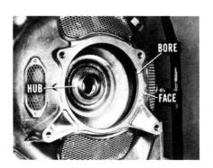
In other words, in addition to inspecting the surface of the hub, you'd want to check for excessive runout of the torque converter hub. Misalignment could result in excessive runout at the bore of the converter housing, or at the rear face of the housing.
