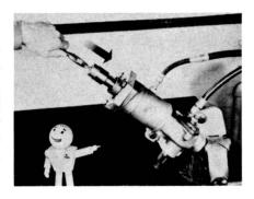
**CAUTION:** Don't leave the unit operating in this position any longer than necessary as high pressure may cause overheating and damage to the pump.
