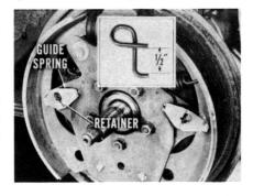
Replace any warped shoes or support plates. Finally . . . button up the brake assemblies and road-test the job.
