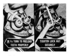
If you still find free play at the wheel, remove the power unit and mount it on the body holding bracket for further work at the bench.
