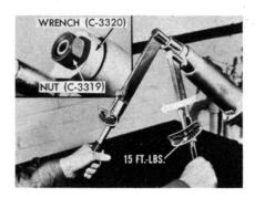
Then, using the special wrench (C-3320) and another torque wrench, tighten the adjusting nut *clockwise* to 15 foot-pounds. Turn the worm shaft several times, next, to seat the bearings. Then, loosen the adjusting nut.
