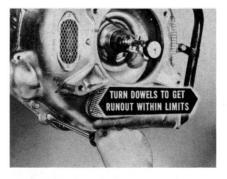
If necessary, loosen the housing screws. With a screw-driver, turn the dowels until they shift the housing to get runout within the limits. This may take some adjusting and readjusting. Again, tighten the housing screws 25 to 30 foot-pounds.
