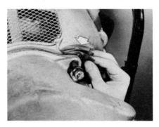
points because you'll be using shims there to square up the transmission. What you do is slip shims over the bolt between the housing and transmission case. The thickness of shims you pick depends on the runout reading. For the correct location and shim thickness to use, refer to the following table.
