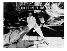
Check also for a bind or looseness at the idler arm. Besides that, look for loose or cocked tie rod ends . . . or loose steering knuckle arms. Tighten or replace any faulty parts.
