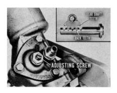
Check the Power Unit—Remember, more than 5/8" free play at the wheel, with the engine running and without moving the linkage, points to looseness in the power unit. There might be a loose gear shaft adjustment, for example.
