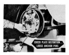
Next, inspect the support plates for distortion, and for loose anchor pins. Use a screwdriver between the plates while you press a finger against the end of the anchor pin to check looseness.
