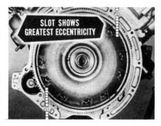
Make sure the mating surfaces of the plate and housing are free from nicks and dirt. Then, install the housing and torque the screws from 25 to 30 foot-pounds. Mount the indicator and check bore runout again.
