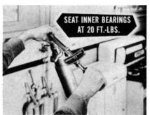
tapered roller bearings, it's wise to check the worm shaft bearing preload adjustment. To do this, you have to seat the inner bearings under a load of 20 foot-pounds. Hold the worm shaft against the bearing at 20 foot-pounds to seat the bearing races.
