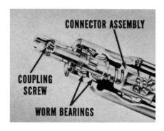
Besides that possibility, the steering worm coupling screw might be loose. In addition, there might be a loose worm bearing preload adjustment. Also, the worm shaft in the connector assembly might have too much end play.
