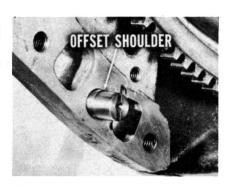
**CAUTION:** Remember to support the adapter plate when you install the *lower* dowel. Without support, you might damage the adapter plate.
