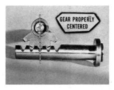
Before you make that adjustment, however, make sure the steering gear is properly centered to the over-all travel of the gear. You can center the gear by turning the steering wheel from one extreme to the other. Count the number of turns. Then, bring the wheel back to the half-way point.
