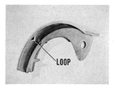
You'll notice that the new brake shoes have *loops* on their outside edges. The new, 5-coil return springs hook into those loops and provide the shoes with both a return force and side thrust.
