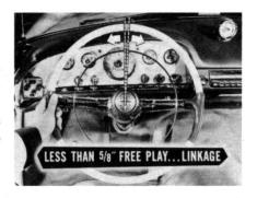
On the other hand, if free play at the steering wheel rim is more than 5%", without moving the linkage, the power unit is at fault.
