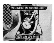
Check Face Runout — You'll have to mount the indicator differently to check runout on the face of the housing. Set the anvil so it bears on the rear face, ½" beyond the bore. Then, rotate the converter a full turn two or three times and check your readings.
