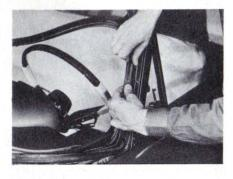
Installing the Glass. Insert the top edge of the glass first, making
