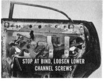
Next, run the glass up and down several times again. The nylon rollers will line themselves up for smooth operation. Last, tighten the lower channel screws.
