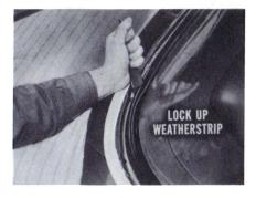
Brush some mild soap solution on the locking strip and use the butt end of the wedge to lock up the weatherstrip. Start across the bottom, up one side, go across the top, and down the other side.
