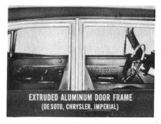
Removing the Front Door Glass. To remove a glass from the aluminum frame models, you take off the inside door hardware, garnish moldings, trim panel and rainshield. Next, you remove the six window
