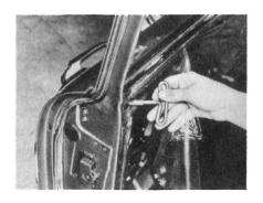
To remove the outside handle, first remove the garnish molding. Then, loosen the rear section of the trim panel. This lets you get at and remove the two handle attaching nuts.
