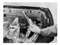
How to Remove the Door Glass. To remove the glass in case it's broken, remove the inside hardware, garnish moldings, trim panel and the rainshield. Be careful when you remove the rainshield, however, as you'll want to cement it back in place later.
