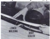
them back in reverse order from the way you removed them. For example, you install the lower molding first. Put body sealer at each bolthole in the cowl as insurance against water leaks. Start the nuts, but don't tighten them. Then, install the lower side moldings, and tighten all nuts.
