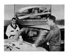
So, push out at either lower corner, then up the side. Once the glass is free, you and your helper can put it over on the bench. Always use a box and padding to support the glass on the bench. These precautions keep the glass edges from chipping.
