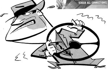
Hard, Jerky Steering at End of Turn. Occasionally, an owner may report hard or jerky steering at the end of a full left or right turn. A loose belt can cause this condition. So can dirt in the pressure relief valve. Dirt in the relief valve will also cause intermittent
