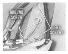
You'll also notice that the lamp sockets are grounded to the fender panel by a separate wire. To replace either the taillamp or back-up light bulbs, remove the two screws. One's at the top, and one's at the bottom of the lamp.
