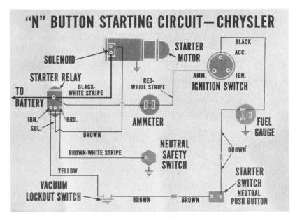
Now, if the car doesn't start when the "N" button is pushed in to the "start" position, you'll have to use a test light to check the starting circuit.
