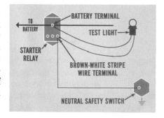
If the test light doesn't light, check the cable adjustment first. If this adjustment is okay, but the test light still doesn't light, replace the neutral switch on the transmission.
