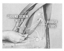
If you ever have to remove the rubber base, first remove the ground screw nut. Disconnect the ground wire and the bulb wires. Then, as you press out the rubber studs, pull the base away from the fender. To reinstall the base, just push the studs through the fender holes until they lock in place in their retaining grooves.
