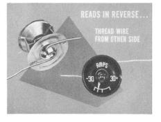
No indication at all means either the generator isn't charging, or the wire from the generator regulator to the starter relay is disconnected. In a case of this kind, you'd first make sure the regulator wire is connected. Then, get the tester and see if the generator is charging. If everything's okay, but the ammeter still doesn't register, replace the ammeter.
