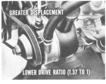
drive ratio of 1.37 to 1 is possible. This low ratio and resulting slower speed contribute to a quieter operating pump.
