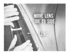
Then, very carefully, move the taillamp lens from side to side to release it from the base flanges. Remove the back-up lens in the same careful manner. Replace the bulbs and reinstall the lens.
