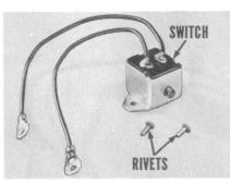
Replace Starter Switch. To do this, drill out the two rivets holding the switch on the flange. The Replacement Switch Package, Part No. 1779888, consists of a new switch and two soft tubular rivets. Install the new switch on the housing flange.
