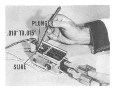
.015". Bend the flange on which the switch is mounted to get the .010" to .015" clearance. Then the switch plunger will have the right travel to close the switch. Test the circuit again, after making the clearance adjustment. If the switch closes, but the test light still doesn't light, then you'd have to replace the switch.
