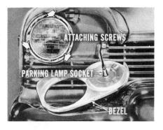
To replace the parking lamp bulb, remove the one long and two short screws that hold the lens to the bezel. Replace the bulb and button her up.
