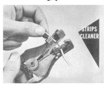
braid covering. You won't have to scrape off any black coating caused by sulphur used in making the rubber coating part of the old-type insulation. Cleaner stripping, incidentally, results in better electrical connections. Clean connections keep down voltage drop and current loss—another important advantage.
