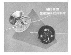
If the ammeter reads in reverse, or shows no indication, it's easy to correct. If you know the generator is charging, a reverse reading means the wire through the loop is reversed. So, remove it, and thread it back through from the other side.
