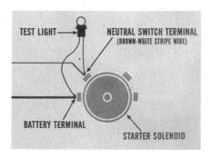
Connect the test light between the battery terminal of the solenoid and the neutral safety switch terminal. That's the terminal with the brown and white stripe wire. If the light lights, the switch is good.
