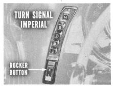
The automatic canceling switch is mounted on the steering column, and automatically cancels the signal when the steering wheel returns to the straight-ahead position.
