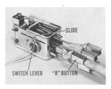
from the slide picks up the switch lever, turns it counter-clockwise and closes the circuit. If this switch ever needs replacement, remove the housing and use a long, narrow-blade screwdriver to straighten the four tabs that hold the switch. Remove the switch. Replace it. Bend the four tabs over, and put the housing back.
