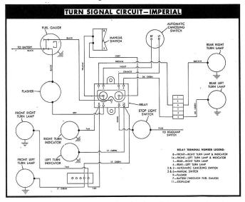
Test The Manual Switch. To check the right turn signal, push the manual switch for a right turn and connect the test lamp between the relay No. 5 terminal and ground. If the test light flashes but the right-turn lamps don't flash, it indicates the bulbs or wiring between the
