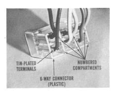
Plastic Connectors. Tin-plated terminals are used in new 6-way polarized connectors made of clear plastic. On the back of the connector, where the terminal enters, each compartment is numbered ("1" through "6") for terminal locations. This makes it easier to follow a wiring diagram.
