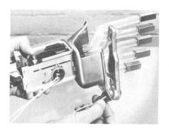
On the Imperial models, the bulb socket snaps into the rear of the housing. So, you'd just reach up behind the housing, pull the socket out and install a new bulb. Then, push the socket back in place.
