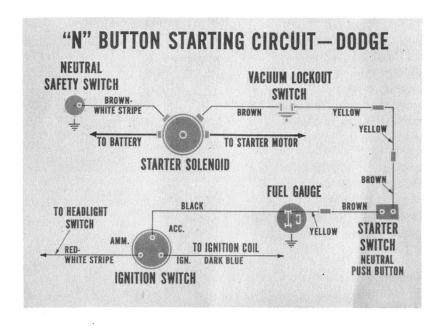
Neutral Safety Switch, Dodge Models. On Dodge, you'd follow the same test procedure you used on the Chrysler circuit—up to the testing of the neutral safety switch. Dodge, as you know, doesn't use a starter relay. So, your test light connection should be made at the starter solenoid.
