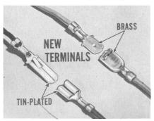
all but the ignition, generator, and starting circuits. There are two kinds, incidentally; brass and tin-plated terminals. The male part of the brass terminal is shaped like a small blade. The female section has curled sides that put pressure on the blade for a good, tight, electrical connection.
