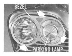
Plymouth Headlamps. On the new Plymouth headlamps, a large plate, called a bezel, serves as a door and support for the parking lamp. To replace the sealed-beam unit, you remove three screws from the bezel. One screw is below the sealed-beam unit. One's at the top. The third one is inboard of the parking lamp.
