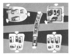
You'd replace the bulb in just about the same way on all but the Imperial models. The main difference is the number of screws that attach the plate, and the screw locations.
