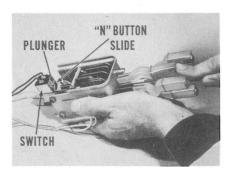
of the "N" button. In other words, after normal travel of the "N" button for a shift to neutral, the end of the slide contacts a spring-loaded plunger. This plunger bridges contacts in a switch to complete the starting circuit. De Soto and Plymouth engines are started with the ignition key, as before.
