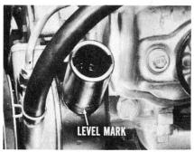
Pump Noise Condition. Now, if the power steering pump ever sounds off, it might be due to too low an oil level in the reservoir. So, see that the oil is right up to the level mark (and no higher) on the filler neck after the pump has been in operation for a few minutes.
