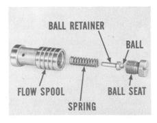
lack of assist. To clean the pressure relief valve, you have to drain the pump and reservoir. Remove a  $\frac{1}{4}$ " cap screw and remove the reservoir. Then remove the  $\frac{1}{8}$ " hex nut that holds the flow valve and spring in the pump body. Remove the flow valve spool. The pressure relief valve is inside the flow valve spool. Remove the screw in the end of the flow valve spool.
