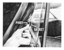
Cut a one-sixteenth-inch-thick rubber shim next. Place it between the gasket and pivot. Reinstall the screw. Press the vent glass forward and securely tighten the screw. This will increase compression at both sides—and at the top. Apply black semi-fluid sealer at the upper pivot on the door.
