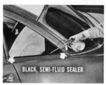
The first step in correcting this condition is to use a gun to apply black semi-fluid sealer between the weatherstrip lip and the reveal panels. Be particularly careful to add a little extra sealer at both lower corners.
