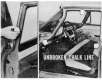
Instead of carpenter's chalk, —or some other fine dusting powder—between the weatherstrip and body all around the door, or deck lid. As in the case of a chalk-test, if the powder blown in leaves an unbroken line, it means the seal is good. But traces of powder found *inside* the line point out places that will need to be sealed.
