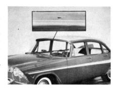
Sometimes there's a leak just outside the windshield opening that will look like a windshield leak. It comes from the three openings in the center of the windshield fence trough — at the bottom. Apply balls of sealer at these openings to keep the water out.
