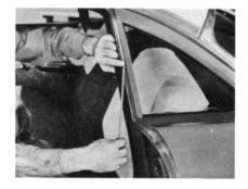
Then, lay a bead of sealer in the seam of the rear door lock-pillar reveal panel. Also at the top and bottom of that panel. The next step is to lay a bead of sealer above the curved reveal
