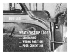
For example, if your watertest at the door shows that water runs down the trim, the weatherstrip may be loose at the dog-leg, or . . . there might be a low spot. Stretching the weatherstrip across the dog-leg or around corners, installing the weatherstrip in an improper position, or a poor cement job . . . all can cause the weatherstrip to come loose from the door.
