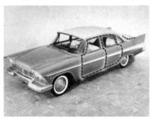
tion of the entire vehicle. Pay particular attention to the fit of the doors and deck lid. If there isn't a proper fit at these points, be sure to correct the fit *before* you do anything else. Sealers cannot be expected to compensate for incorrect mechanical adjustments.
