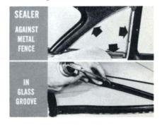
Next, install the quarter window and its sealed weatherstrip into the opening, and reinstall the inside garnish molding. Finally, run a bead of black semi-fluid sealer under the outer lip of the weatherstrip.
