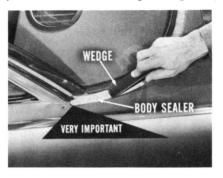
If water was detected as getting between the metal fence and upper part of the weatherstrip, put body sealer or cord-type sealer in the channel above the molding. Pack it in place with the wedge, or clothespin, and then paint it to match the finish.
