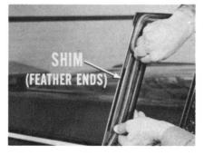
NOTE: For a good cementing job, put a thin coat of cement on both the weatherstrip and metal surfaces. Let each coat become almost dry and slightly tacky. Keep in mind that too little cement is better than too much. You'll get a more solid bond with a thin coat. Also, apply the weatherstrip on the door flange first, and then, to the door frame.
