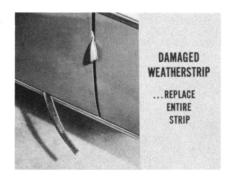
If you happen to find a low spot, you can shim it up with rubber shims cemented in place underneath the weatherstrip. Remember to featheredge the ends of the shim, however, to prevent any bulging of the strip.
