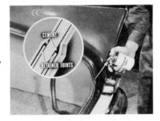
Now, if water gets between the weatherstrip retainer and body panel, body sealer will make an effective seal. Pack it in between the retainer and the body.
