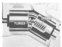
pushes both blocks out against the end cap and pump housing to form a seal, until pressure builds up. When that happens, fluid pressure in the space between the cylinder blocks forces the cylinders out to form a seal at the end cap and at the housing.
