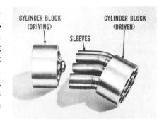
It's a lot easier to follow basic operation of the pump if you concentrate on what happens to one chamber during a complete cycle. For example, as one sleeve and both blocks turn one-half revolution, the chamber *increases* from its minimum to its maximum length. It goes from short to long.
