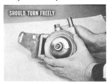
make sure it doesn't bind. Wrap a fan belt around the pulley to keep it from turning while you tighten the pulley cap screw to 20 foot-pounds. Finish assembling the pump. Install the pump in the car. Be sure that no dirt gets inside the pump assembly during any stage of installation on the car.
