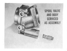
If you come across a rare case where any of the valve parts are badly scored, remember that the spool valve and pump body are serviced as an assembly.
