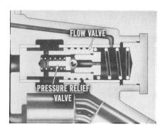
If the flow valve—or the pressure relief valve inside it—sticks open because of dirt, the pump may not provide steering assistance. More often than not, you'll find that checking the flow valve or pressure relief valve first will save you time and effort.
