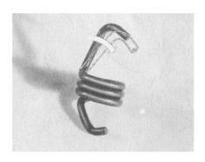
If that doesn't work, then install *new* return springs. Front brakes on Plymouth and Dodge take 3-coil springs. Other models take 4-coil springs. Rear brakes on Plymouth and Dodge use 6-coil springs. Other models use 5-coil springs.
