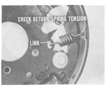
Check to see if there is proper return spring tension. Even a new spring won't return the shoe correctly if the link it hooks up with hangs up on the brake shield. You see, the link affects spring action. What's more, it automatically adjusts return spring tension whenever brake shoes are adjusted.
