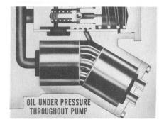
In fact, there's oil under pressure throughout the sleeve-type pump. As a result of small clearances, a tiny amount of oil finds its way between the sleeves and cylinder blocks into the center section, or knee, of the pump. So each internal part works smoothly on a film of oil.
