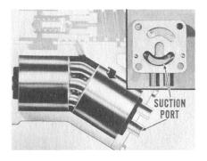
As the chamber gets longer, it draws oil in from a suction port in the end cap. This action is similar to what happens when a suction gun is used to draw oil out of a container.
