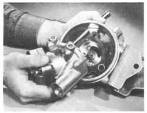
Then, assemble the pump body to the housing, making sure you use a new body gasket and a new flow valve seal ring.
