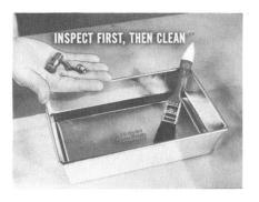
Inspect the parts in an attempt to find the cause of the condition before cleaning them. Occasionally, parts are dumped into solvent first, which removes the guilty particle of foreign matter, and the technician never quite knows what may have been causing improper pump operation.
