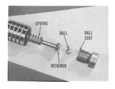
The pressure relief valve is inside the spool. So, remove the screw in the end of the spool. This screw is the pressure relief valve ball seat. Also, remove the ball, the ball retainer and spring.
