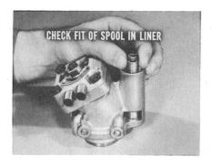
Check the fit of the spool in the liner. It should slide through the liner by means of its own weight. If it sticks at any point, find the nick or burr responsible and polish it out. Recheck spool movement in the liner.
