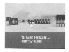
To raise pump pressure, you can insert a  $\frac{1}{32}$ " washer (Part No. 1733017) between the spring and ball retainer, and then reassemble the valve. Install the pump and recheck the pressure.
