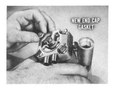
Remove the parts from the fixture next. Install the end cap, using a new gasket. Tighten the cap screws finger-tight to keep the driven block in place.
