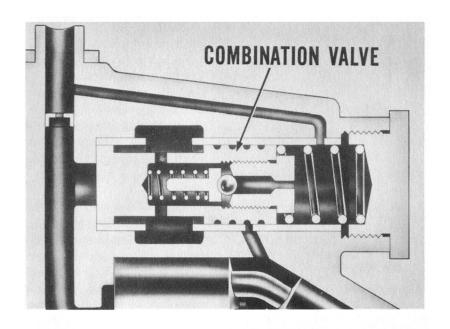
All of the oil displaced by the pump is discharged through a combination flow and pressure relief valve. This combination valve maintains a constant flow level, regardless of pump speed and pressure, and directs the oil to the steering gear.
