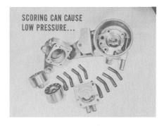
And if each sleeve has a smooth, slip fit in the bores, and some suction develops when you hold both ends closed as you withdraw the sleeve, the sleeve fit is probably all right.
