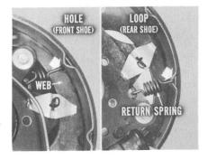
So, by hooking the return spring on the rear brake shoe off dead center, the shoe is pulled slightly sidewise and bears against the support plates. This helps damp out vibration.
