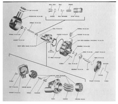
On 1957 Chrysler, Imperial and Plymouth cars, the power steering pump is of new design: it is known as a sleeve-type, positive displacement pump. Let's take a look at how it works.
