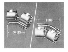
During the remaining half revolution, the chamber decreases in length. It goes from long to short. This change in chamber length provides positive displacement pumping action.
