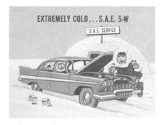
where there's a lot of belowzero temperature, S.A.E. 5-W may be used. Type "A" fluid is so viscous at extremely low temperatures, it could cause quite a drag on the starting motor. As soon as the cold weather period is past, however, drain the pump and use type "A" fluid, or mineral
