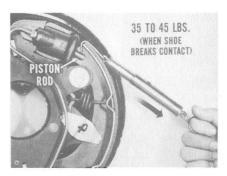
To check return spring tension, use a spring scale and pull the end of the shoe away from the wheel cylinder in the direction of piston travel. You should read 35 to 45 pounds when the shoe breaks contact with the piston rod.
