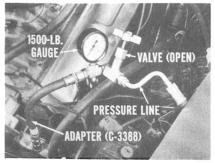
So, with the aid of a special adapter hose (C-3388), install a 1500-lb. pressure gauge (C-3309-B) in the pressure line between the pump and the gear. Make sure the gauge line valve is open so oil flow to the gear won't be restricted. Also, connect a tachometer as your guide to engine speed.
