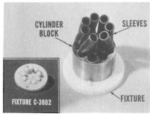
Use of the new assembly fixture (C-3602) is a must—it is next to impossible to assemble this pump without it. Place the driven block, the one without splines, on the fixture. Then, oil and insert the plunger spring, plunger and seven of the nine sleeves next.
