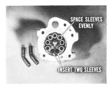
Place the splined block over the sleeves. Sight through the bores and lower the block until it engages the two sleeves in the forward position. Again, use the probe to align the next two sleeves while you push the driving block gently downward.
