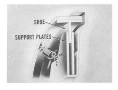
**Brake Noise.** Now, if you ever check into a case of brake noise, make sure the contact loops ride against the brake shield properly. Use a light and check from the anchor end of the shoe.
