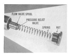
How to Inspect the Flow Valve. First step in examining the pump will be to remove it from the car and then drain it. Remove the reservoir. Next, unscrew the large hex nut that holds the flow valve and spring in the pump body. Remove the flow valve spool.
