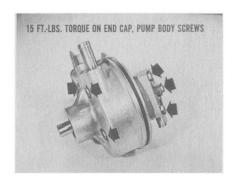
If these cap screws are tight, belt tension and fluid level are correct, you would suspect some internal damage to the pump as being the cause of low pressure.
