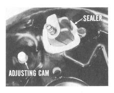
To correct this condition, clean the shoes and drums thoroughly. Use heavy body sealer outside the shield to seal off any openings. Always make sure the seal at each adjusting cam is in place, and in good condition, also.
