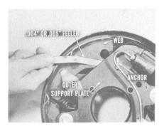
Slide a .004" or .005" feeler blade between the shoe web and outer support plate at the anchor end. If you can do it, there's no bind at that point, and the shoe is lined up okay.
