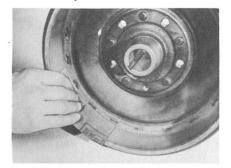
drums. This, in turn, may leave a glazed deposit on the drums. This deposit, as you know, causes brake squeal, and reduces effective brake action. In a case like this, clean the drums and lining surface with number 200 or 300 emery paper.
