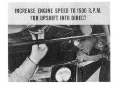
Now, when that upshift takes place, there should be a 26 to 32 psi compensated throttle pressure reading on the gauge. But, don't stop at this point.
