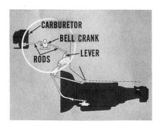
The other linkage setup uses an intermediate bell crank mounted on the intake manifold. It also uses two rods: one from the carburetor to the bell crank; the other from bell crank to the accelerator shaft lever on the dash panel.
