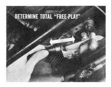
Now determine the total "free-play" of the cable. Push the cable into the housing. Mark it. Then *gently* pull it out. Measure the total amount of cable travel.
