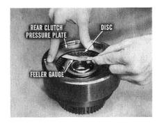
You check that clearance by temporarily installing a *rear* clutch pressure plate, Part No. 1732114, on top of the clutch pack. Hold this rear pressure plate firmly in place by hand, and insert a feeler gauge between it and the top disc in the assembly.
