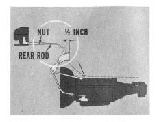
Next, push the rear rod backward to get about ½" clearance between the dash panel and the accelerator shaft lever. Hold the rods in that position, and tighten the clamp stud nut.
