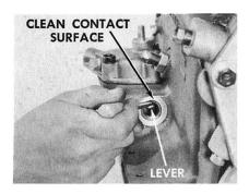
If necessary, use a screwdriver to bend the lever as required to get it properly lined up. In addition, clean the switch contact surface on the transmission so the switch will have a good ground. Install the mounting washer on the switch so the concave face is away from the switch. Place the rubber "O" ring on the switch and install the switch in the case.
