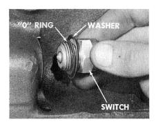
Turn the switch in until the washer contacts the case. Then, tighten the switch an extra ½-to ½-turn. Connect the wire and recheck switch operation.
