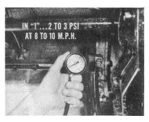
Next, start the engine. Push in the "1" button. You should read no more than 2 or 3 psi at 8 to 10 miles per hour. More than 3 psi means that the governor valve is open, probably because the governor weight is stuck.
