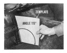
If you ever have to change the accelerator pedal angle, remove the pedal end of the accelerator shaft-to-pedal rod at the pedal lever.
