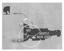
Then, push the throttle valve lever on the transmission forward to its closed position. Pull the forward half of the rod back just enough to remove the slack, and tighten the clamp stud nut.
