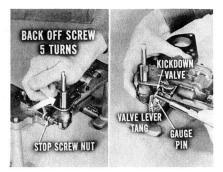
from the transmission, mount it in the stand, loosen the throttle valve stop screw nut, and back off the screw about five turns. Insert the gauge pin between the valve lever tang and the end of the kickdown valve. Keep the pin in line with the valve.
