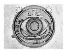
brake and not the transmission. Check this by pulling the parking brake lever out one to two notches. Drive the car. Then let it coast. If there is now no rattle with the brake pulled out, it means that the brake shoes are making a partial contact with the drum when the brake is in fully released position.
