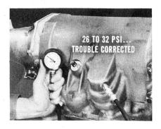
But if you don't get the correct readings, the only thing left to do is reset throttle pressure. And that's where the new pin gauge comes in. Here's how that's done. You first remove the valve body assembly
