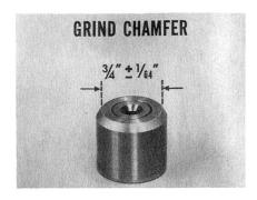
Hold a 34" diameter on the face of the weight, plus or minus 1/64". Then you'll end up with a chamfer that will adequately clear the chamfer on the output shaft ramp.
