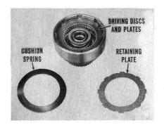
On top of that, you install a driving disc, and then a plate. Keep this up until four discs and three plates are installed. Don't install the cushion spring or the retaining plate just yet.
