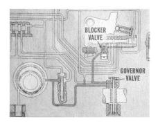
As you probably know, an open governor valve admits pressure to the reverse blocker valve. This, in turn, keeps the transmission from shifting into Reverse. As a result, you'll have to remove the governor for cleaning and inspection.
