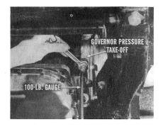
In a case like that, you'd check governor pressure first. So, raise the car up on the hoist with the wheels free to turn. On the *left* side of the output shaft support, remove the tap plug from the governor pressure take-off hole. Connect a 100-lb. Pressure Gauge (C-3292).
