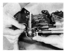
bottoming the valve completely inside the body. As you do that, tighten the throttle valve screw finger-tight (do not use a wrench), so all free-play of the lever is removed. Be sure the adjustment is made with the spring fully compressed and the gauge pin held in line with the kickdown valve.
