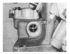
In a case like this, the neutral starter switch may need attention. So, remove the switch and see that the neutral starter switch lever in the transmission is located in the center of the hole where it can make positive contact with the switch.
