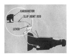
Correct throttle linkage adjustment is one of the most important items in proper transmission performance. On the Torque-Flite unit, two basic types of linkages are used. One of them uses a two-piece slipjoint rod between the carburetor and accelerator shaft lever on the dash panel.
