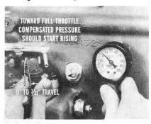
throttle. Compensated throttle pressure should start rising when there's 0 to  $\frac{7}{32}$ " travel at the outer end of the lever. If pressure was above 32 psi with the lever against the stop, and if the pressure increased immediately when the lever was moved, you'll have to adjust throttle pressure.
