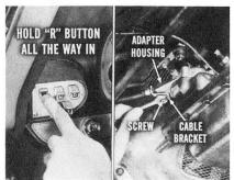
To make this adjustment properly, have someone hold the "R" button all the way in. That removes the slack from the linkage. Loosen the screw holding the control cable adjustable bracket to the adapter housing.
