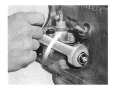
You can also use a test light to check the neutral switch operation.
