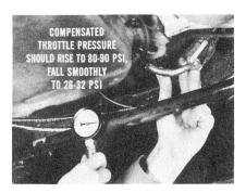
32 psi at closed throttle. If you don't get the 80 to 90 psi throttle pressure, it points to faulty throttle compensator valve or throttle valve operation. That, in turn, will call for draining the transmission, dropping the oil pan, and removing the valve body for cleaning and inspection.
