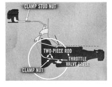
Now, with the linkage loose, and the transmission in Neutral, adjust engine idle at 475 to 500 r.p.m.
