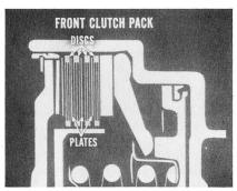
A front clutch pack with the wrong build-up of discs and plates does not have enough clearance and won't let the clutch release properly when the transmission is in Neutral, or when shifted to Reverse. Your best bet in this case is to remove the transmission and disassemble the clutch.
