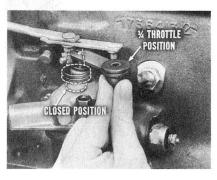
Before you do this, there's one more check you should make while the engine's running at 1500 r.p.m. Suppose you read the 26 to 32 psi, but pressure failed to rise after you moved the lever  $\frac{7}{32}$ ". Advance the lever slowly to about  $\frac{3}{4}$  throttle position, and return it to closed position.
