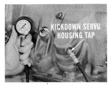
To reset throttle pressure, first hook up a tachometer to the engine. Also, install a 100-lb. Pressure Gauge (C-3292) in the kickdown servo housing *upper* tap.
