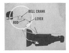
Follow the same general procedure on the linkage type that uses the two rods and intermediate bell crank with just one difference. The upper adjustment is made at the rod from the bell crank to the accelerator shaft lever instead of at the slip-joint of the two-piece rod.
