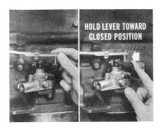
As you hold the lever there, slowly pull down on the accelerator pedal lever to increase engine speed to about 1500 r.p.m. This will make the transmission upshift into Direct.
