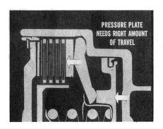
Now, remember that the front clutch pressure plate has to have the right amount of travel when pressure is applied. This means that the proper amount of disc clearance has to be maintained. Not enough disc clearance will cause the clutch to drag. Too much clearance will cause a delayed clutch engagement.
