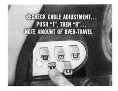
The amount of over-travel will be about the same for each button when you have the control cable properly adjusted. If either the "1" or the "R" button has no over-travel, you'll have to repeat the cable adjustment.
