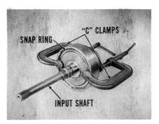
Complete your assembly of the input shaft and snap ring by using two large C-clamps, or an arbor press. That's the story on the front clutch build-up.
