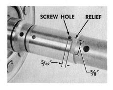
tire relief should be about 58" long. After grinding, smooth off any burrs and use crocus cloth on the governor body bore if it needs to be smoothed out. Clean the shaft and governor parts as before.
