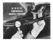
Keep advancing the transmission throttle valve lever toward full
