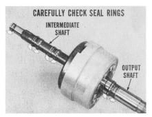
transmission apart, it's wise to inspect the seals, too. For instance, carefully check the interlocking seal rings on the intermediate and output shafts without removing them. There should be no worn or broken interlocks... and they should turn freely in their grooves.
