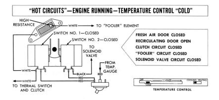
By referring to the diagram above, and to the illustration of the control unit arrangement, you will note what happens with the temperature control lever on "COLD". The Bowden wire still won't be moved far enough to open the water valve. Microswitch #1 will be closed, completing the circuit from the *red* wire input to the two *white* wires leading from the switch.
