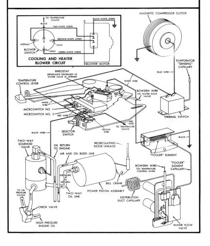
Another glance at the diagram will show you that the temperature control lever operates a Bowden wire connected to a water flow valve. It also controls opening and closing of microswitches #1 and #2.
