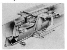
Moving the unit under the hood, of course, made more trunk space available. It also improved the distribution of cold air, delivering it at the front of the car instead of against the back of the passengers' necks.
