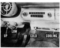
After making sure your controls operate properly, turn your attention to the refrigeration part of the system. To do this, set the air control on "UP", the blower on "LOW", the temperature control lever on "COLD", and the selector switch on "COOLING". Close all car windows.
