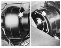
Normally you wouldn't think an air leak through the seam in the blower housing, or between the blower housing and the blower motor would be worth considering. But it is! So, use body sealer to seal these points thoroughly.
