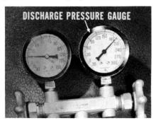
testing outfit (C-3354), designed mainly for Freon 22, had a 300-psi range on the left-hand gauge and a 600-psi range on the right-hand gauge. This would not lend itself to accurate readings on the new air-conditioning units which use Freon 12.
