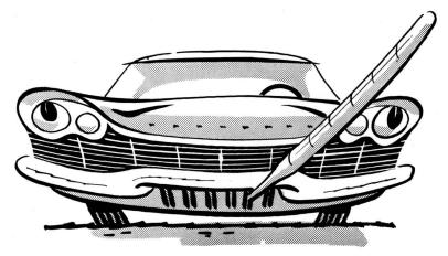
Direct all air "UP". Set the blower control on "HIGH". Then, suspend a thermometer in one of the open outlet grilles. Have it face so that you can read the outlet air temperature from outside the car.
