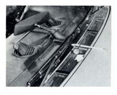
Place a second thermometer near the center of the cowl vent. Rest it across a pencil to keep the thermometer bulb from touching the metal of the grille. Close all car doors and windows. Recheck your tachometer to see that engine speed is still 1200 r.p.m. while the compressor clutch is engaged.
