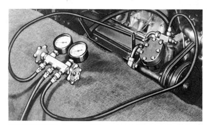
Make sure that both manifold gauge set hand valves are fully closed. Next, connect the hose from the left-hand gauge to the suction port, and the hose from the right-hand gauge to the discharge port.
