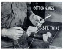
a two-foot length of twine to the upper end of the thermometer. Now, wet the bandage in water that's at room temperature. Using the string as a sling, swing the thermometer in a circle for several minutes to speed up evaporation at the bulb.
