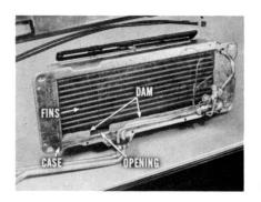
stead of through the cooling coils, cooling efficiency suffers. To prevent this type of leak, use sealing compound to build a dam across the bottom of the evaporator case. That will keep air from sneaking in between the fins and case. Leave about a 2" opening so water can flow out to the external evaporator drain.
