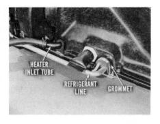
Then, check to make sure the evaporator and housing seal well against the dash panel. If any of the attaching bolts are loose, tighten them to 30 inch-pounds, but take it easy! There's a new palm-grip ratchet wrench (C-3616) with an extension (C-3622) that is a real
