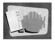
The blower, on the engine compartment side, acts quite a bit like a vacuum cleaner. Just a small leak on the suction side of the blower can draw in enough hot air to raise the temperature of the air entering the car, and make a noticeable difference in cooling. In short, the refrigeration part of the unit can be perfectly okay, but hot-air leaks can nullify the results. Leak possibilities, therefore, have to be checked out very carefully.
