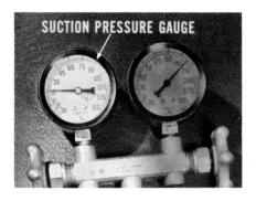
Notice the combination gauge that gives vacuum readings down to 30 inches of mercury and pressure readings up to 150 psi. This is the left-hand, or "suction pressure" gauge.
