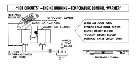
When the temperature control lever is in the "WARMER" range, the Bowden wire opens the water control valve. The more you move the lever to the right, the more hot water flows through the valve to the heater core.
