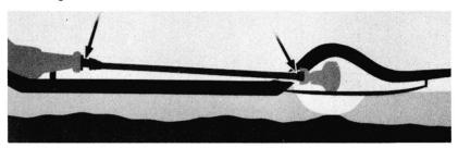
In addition to the changing angle-of-drive, there's also a slight change in *distance* between the output and pinion shafts. The universal joints, therefore, must do more than provide a connection throughout various angles. They also have to allow for slight variations in distance between the transmission and rear axle.
