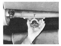
Following out our example, we have a  $1^{\circ}$  angle of the front shaft; subtracted from the  $2^{\circ}$  angle of the rear shaft, this gives an answer of  $1^{\circ}$  for the working angle of the center joint. This is within limits, so no further work is required.
