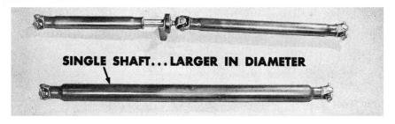
But when you go to too large a diameter, you're very apt to introduce more vibrations. There's more mass to rotate, for one thing. Also, it's very difficult to *balance* a longer, thicker shaft.
