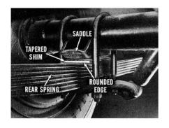
Always keep the flat side of the shim with the rounded edge toward the spring, and see that the thick end points forward. After installing the shim, recheck the rear flange angle. This is mighty important because you'll want to know that the angle is within limits.
