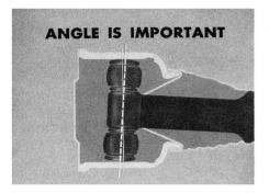
Importance of Working Angle. Since the universal joints must transmit torque through an angle, the degree of angle is mighty important to the maximum life of the parts.
