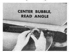
Next, disconnect the universal joint at the pinion shaft. Put the spirit level against the front face of the companion flange. Hold the level so that its long dimension is vertical, and center the bubble. At this point, let's assume the pinion shaft slopes down about  $2\frac{1}{2}$ °.
