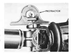
To check the center joint yoke alignment, remove the bearing lock plate from the center yoke. Turn the yoke so the bores are vertical. Adjust the protractor scale to zero and put the protractor on the yoke at a  $90^{\circ}$  angle to the frame centerline. Rotate the yoke to center the bubble.
