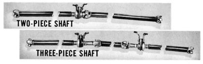
As on the Imperial, a center bearing bracket supports the rear of the front shaft. On three-piece shafts, you'll find a bearing bracket at the rear of the front and center shafts.
