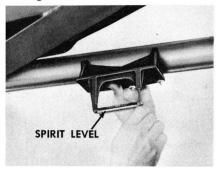
But, if the leading edge of the bubble is ahead of the third graduation, you'll have to put a 2° tapered shim between the spring and its saddle to correct the angle. As before, shim the struts, too, so they're free and unloaded and will let the pinion shaft assume the proper working angularity.
