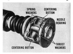
The cross-type joint has a yoke, a cross, two roller-bearing-and-bushing assemblies, two roller-bearing-and-block assemblies, dust seals and retainers.
