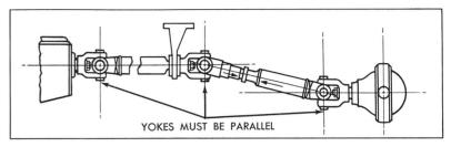
Now, to line up the yokes properly, you must use bearing brackets of the correct length, and the proper rear axle spring seats. Brackets on different models vary in length from about 23/8" to 415/16". Using the wrong length bracket can cause too great a working angle and its resulting vibration. A chart that lists the brackets and spring seats to use for the corresponding model is given on the next page.
