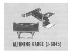
You'll notice that this new tool consists of an index gauge and an adapter. The gauge has an adjustable spirit level and provides direct readings of the angles at the pinion shaft and rear propeller shaft. You use the adapter to apply the gauge to the front propeller shaft where space is limited by the X-frame member on hardtop models.
