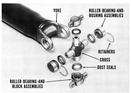
A sliding spline connection between the prop shaft and the joint compensates for variations in distance between the output shaft and the pinion shaft. On all cars but the Imperials, you'll find a one-piece shaft that uses a ball-and-trunnion joint at the front, and a cross-type joint at the rear.
