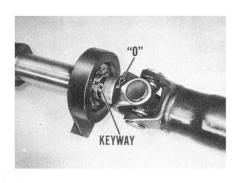
Checking Two-Piece Shaft. You're now ready to check phasing of the center universal joint. See that the letter "O" on the front face of the yoke lines up perfectly with the keyway in the rear end of the front shaft. To get a clear look at the keyway, back off the oil seal cap about ½".
