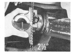
Now, add your two readings  $(2^{\circ} + 2\frac{1}{2}^{\circ})$  and you'll get the working angle of the rear joint,  $4\frac{1}{2}^{\circ}$ , in our example. Don't forget that specifications call for an angle not over  $3^{\circ}$ . So, in this instance, you'll have to correct the angle by reducing it until it falls within the  $1^{\circ}$  and  $3^{\circ}$  limits.
