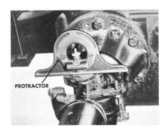
Next, swing the protractor  $90^{\circ}$  so it will be parallel to the frame centerline. Again, adjust the level to center the bubble. Read the scale opposite the zero indication mark. This angle should be the same as the engine angle, within  $1^{\circ}$ .
