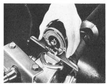
centering the bubble in the sight glass. Read and record the degree of engine declination, which is the vertical angle of the yoke. Then, remove the joint yoke bearing lock plate from the axle pinion shaft yoke, and turn the yoke to put the bores in a vertical position.
