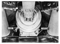
Check for the presence of undercoating overspray on the propeller shaft or parking brake drum. Overspray alone is enough to cause an out-of-balance condition. Once you've checked these points, you're ready to check the working angle.
