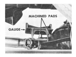
Place the gauge squarely on the underside of the rear shaft, spirit level on the left. If the bubble's leading edge is centered, or within
