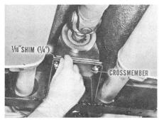
easily done. You simply add or remove  $\frac{1}{16}$ " shims between the center support insulator and crossmember. One  $\frac{1}{16}$ " shim will change the center angle about  $\frac{1}{4}$ °. If the angle is too low, you'd add shims to increase it. If the angle is too great, you remove shims to cut it down.
