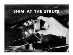
When you install a shim at the spring saddle, you'll probably have to do some shimming at the struts. Just loosen the attaching bolts and add shims until the struts are free and unloaded. This releases the load on the rear axle housing and permits it to assume the proper angle.
