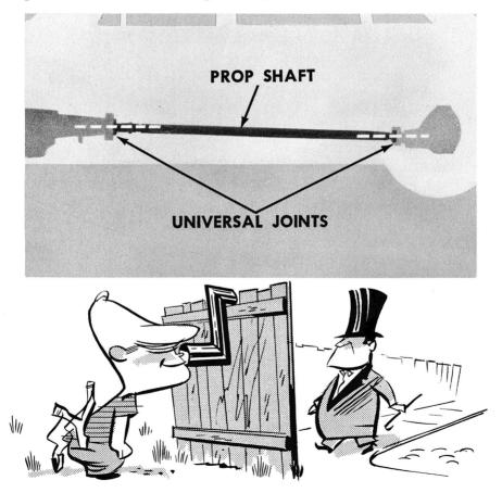
One important point to keep in mind is that the transmission is attached to the frame crossmember. As a result, the transmission output shaft won't change in relation to the frame. On the other hand, the pinion shaft does change in relation to the frame and, consequently, to the output shaft. This happens each time the rear axle moves up or down because of travel over uneven road surfaces.
