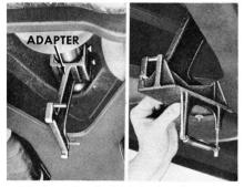
adapter pins pointing left. Tighten the thumb screws to secure the adapter to the shaft. Then, index the gauge on the adapter so the level is at the left. Make sure the locating pins index squarely on machined pads on both the adapter and gauge.
