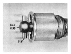
The ball head for the trunnion pin is a built-in part of the prop shaft. The pin is a press fit in the ball head and is accurately centered so that each end extends the same distance. If the pin is off center by as little as .003" it can cause the shaft to run out of balance, setting up a vibration.
