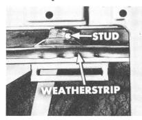
arm studs when the glass starts down, use a fiber wedge to work it past the studs. And, once you get the weatherstrip past those studs, you can pull the glass down the rest of the way. But take it easy! If you're not careful, those studs can scratch the glass.
