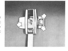
If the studs on the model you're working on aren't marked, use a late model handle as reference to make a paper template to locate the stud centers. In case you don't have a late-production handle
