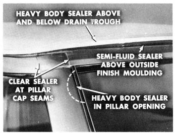
**Drain Trough.** A seam between the drain trough and roof rail at the rear of the roof panel may have small pin holes. Water getting through will come out under upper garnish moldings or rear body pillar garnish moldings. If you suspect this type of leakage, lay a bead of rope-type body sealer along the lip of the drain trough. Use a clothespin to press it firmly under the lip of the drain trough. Remove excess sealer for neat appearance.
