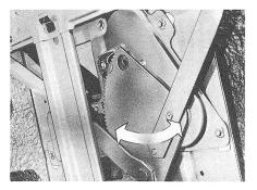
Scribe the lower edge of the regulator base and loosen the attaching screws. Rotate, or shift the regulator to even up the glass, and tighten the screws. Recheck the glass travel again and see if you've evened it up properly.
