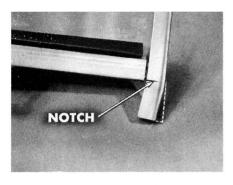
torting, or flaring, the sides of the frame. You can also use heavy pliers to pinch the sides slightly. Then, file down the edges so there will be no burrs or sharp corners. On current models, the lower ends of the frame have been revamped to avoid any interference in the channels.
