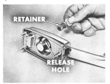
release hole. If you don't do that, the lock won't work properly. You see, you can install the lock cylinder upside down. It'll go in all right. But it will lock in place. The result? You won't be able to get it out at all.
