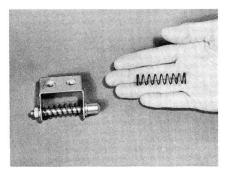
Once you have that assembly out, you'll notice that there's probably only one spring on the sliding bolt. So, add a second spring to increase the bolt pressure.
