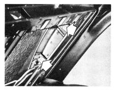
Check glass operation once more. Run the glass up and down to see how easily it works. Be extra sure that the top edge of the glass enters the weatherstrip evenly as you crank it up into fully closed position. If you find that the glass rises evenly, and without any binding, you're all done. So tighten the regulator handle nuts and that will finish the job.
