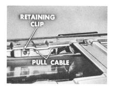
Next, install the garnish molding and the latch operating handle. See that the latch pull cables or rods run through the retaining clips just under the molding. That will keep those cables tucked out of the way so they won't snag themselves on the regulator arms.
