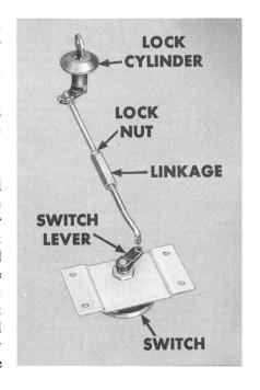
**Limit Switch.** In the BROWN wire circuit, this series switch opens the circuit when the gate is opened, preventing accidental raising of the glass.
