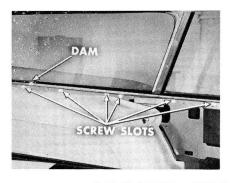
Now, once you have that construction completed, build a dam of body sealer at the rear end of the lower run channel. Also, seal the garnish molding screw slots. Then you can install the glass, the upper run channel, and the moldings.
