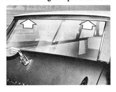
Level the Glass. If the glass doesn't rise evenly, notice which side lags as you crank it up. Lower the glass, open the gate, and crank out the glass so you can reach the regulator attaching screws.
