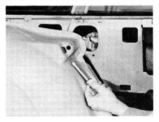
seat-back will fly forward when the suburban makes an emergency stop. If you find this condition, remove the garnish molding and the trim panel. Remove the two screws holding the latch, and reach through the access hole to remove the bolt assembly.
