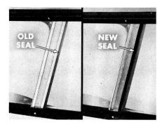
To install this seal, remove the upper, lower, and both end garnish moldings. Slide the window rearward, and remove the upper run
