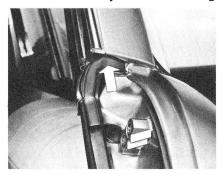
end at the top should fit into the opening at the lower end of the body pillar. It should be positioned to extend about ½ inch below the lower end of the pillar. It seals against dust and exhaust fumes funneling up into the car through the pillar opening. If the weatherstrip has been stretched, and has been recemented
