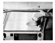
Before you reinstall the glass and the trim, there's another leak possibility that deserves your attention. Any water getting into the sliding glass lower run channel can follow back, spill out, pass under the garnish molding behind the quarter panel trim and onto the floor. Or, it might leak out the garnish screw slots and run over the trim on the inside.
