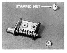
In addition to those tips, take a rat-tail file and enlarge the bolt hole in the wheelhouse. That'll make sure the bolt will enter the hole easily without hanging up. Install the catch, the trim and molding, and you're all set.
