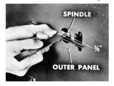
If you should find there's less than 3/8" operating clearance, all you have to do is install shims between the regulator and its mounting bracket at each attaching screw.
