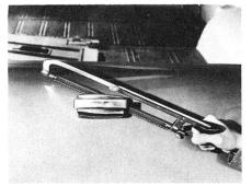
careful not to saw through the lock cylinder which extends into the boss. Also, before you saw through the right side, open the handle so that you don't saw through it. Once you saw about two-thirds of the way around, break off the boss and remove the handle.
