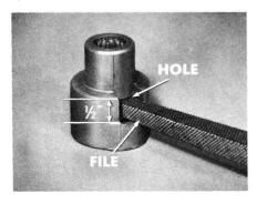
If you do run across a case like this, it's fairly easy to repair. Just turn the lock to its locked position and remove the housing from the handle assembly. Use a small file to elongate the bolt slot until it is about ½" long.
