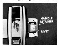
Remove and Install Lock Cylinder. Now, here's something else. If you ever have to remove a lock cylinder, turn the key a quarter turn, so it is horizontally positioned in the cylinder. Then push a paper
