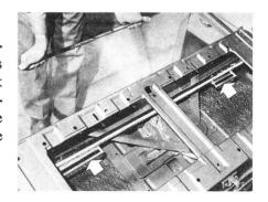
Inspect the glass frame. Take a close look at the lower ends of the frame especially. If those ends are sharp, they'll gouge and bind in the run channels. You can correct sharp ends very easily. Just make a saw cut or notch in the side channel right below the lower window frame member. Then you can bend the channel inward without dis-
