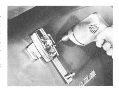
Some handles have three countersunk spots which mark the exact centers of the attaching studs, so you know just where to drill.
