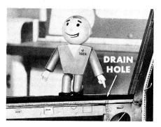
A small drain hole at the forward end helps to carry water away. But, when the suburban is on an upgrade, water will run away from this small drain. Fitting the sliding glass more tightly isn't the right answer because owners prefer an easily operating glass.
