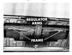
Don't install the handle until after you install the glass. If you install the glass first it may be positioned so the handle will not fold into its retainer when the glass is fully raised. When you install the handle, leave the attaching nuts finger-tight temporarily. Then, if you have to reposition the regulator to adjust the glass, the handle will shift with the regulator spindle.
