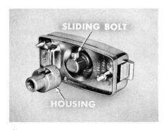
Repair the Handle. Once you remove a handle, disassemble it to find out what may have caused the difficulty. You may find the sliding bolt doesn't engage the housing. In other words, the handle may have just been "free-wheeling" when the owner tried to crank down the tailgate glass.
