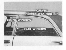
Move the window forward, if necessary, to line it up with the edge of the front window. Next, tighten the fore-and-aft window roller track upper bracket screws. Lower the rear window and shift the lower end of the roller track into contact with the frame. Then, tighten the window roller track lower screws.
