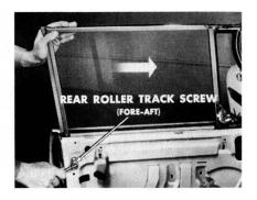
Lower the window next. Hold the roller track against the frame
