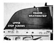
While the rear window is all the way up, adjust the upper stop screws. Be sure, also, that there's no interference at the header weatherstrips, or the door will be too hard to open. Last, lower the window until it is flush with the top of the door and adjust the lower stop.
