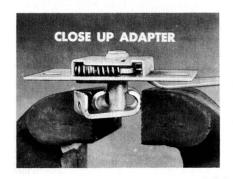
In a case like that, remove the remote control, and close up the adapter in a vise. When you reinstall the set screw, tighten it just enough to hold the handle securely. Here's another condition to check. If a throttle-type handle won't return to its released position, it may be binding in the armrest guide slot. Slotted shims installed behind the remote control base will center the handle in its slot and eliminate the bind.
