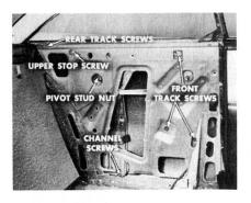
Here's how you'd go about adjusting the quarter window. First loosen the roller track bracket screws and the pivot stud nut. Loosen the two center channel support bracket screws, and the upper and lower stop screws.
