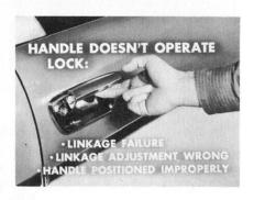
Knowing how the linkage looks and works will help you check its adjustment whenever the lock appears to need attention. For instance, the linkage consists of two flat steel links, with serrated sur-
