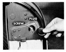
Just reach in, loosen the screw and shorten the linkage. If the adjustment doesn't hold, then you'd remove the trim panel to get inside and check the linkage more thoroughly. On Imperials, you must remove the trim panel to check and adjust the linkage as there is no access hole in the rear face of the door.
