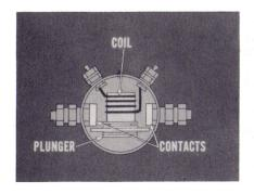
amperes, solenoid construction differs from that of a relay. The solenoid has a coil, a plunger, and a set of heavy duty contacts. Turning the ignition switch to Start completes the solenoid coil circuit and the coil becomes a powerful electro-magnet.
