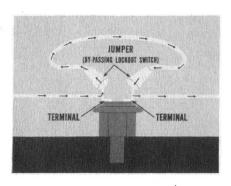
minals to take it out of the circuit by bypassing it. Then, if the starter operates when the Neutral button is pushed, the trouble is in the lockout switch. But, if the starter is still dead, and the starter solenoid and starter relay are okay, the trouble is in the Neutral push-button starter switch.
