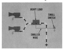
carry the heavy load required by the horn. When a relay carries the heavy load, a small switch can be used in the control circuit without any danger of burning the switch points. Also, smaller wire can be used in the horn control circuit.
