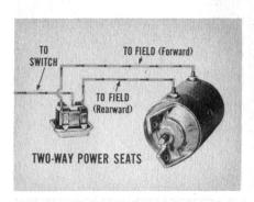
Power seats, power windows and convertible tops are operated by reversible electric motors which have two sets of field windings. When one field is energized, the motor runs clockwise. When the other field is energized, the motor runs counterclockwise. A two-way switch controls the direction of rotation.
