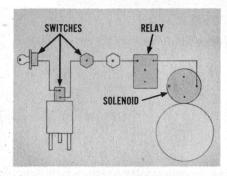
On Plymouth, Dodge, and De Soto Firesweep models, the starter sciencid acts like a heavy-duty relay. It is a magnetically operated switch. But because the starter sometimes draws more than 100
