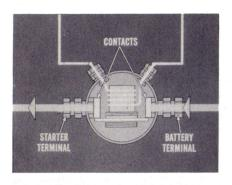
Right away, the plunger is pulled toward the center of the magnetic field set up by the coil. A contact plate on the end of the plunger bridges the contacts. This completes the circuit from the battery terminal to the starter terminal of the solenoid.
