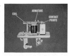
Pushing the horn ring completes the circuit through the coil. The coil, in turn, produces a strong magnetic field which pulls the armature down, closing the contact points. That completes the circuit from the battery to the horn.
