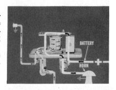
Checking the Horn Circuit. Now, if the horn won't blow, and there is a relay in the circuit, use a jumper to check whether trouble is in
