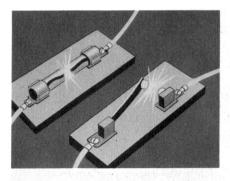
Now, *shorts* aren't too hard to locate. The wire heats up and insulation begins to burn on the shorted wire or unit. But before there's any serious damage, a fuse . . . or circuit breaker . . . disconnects the shorted-out section of the circuit from the source of supply to protect the entire system.
