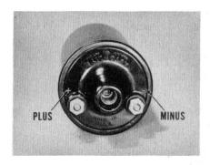
Coil Polarity Is Important! In case you've ever wondered, reversing the coil primary leads does affect the strength of the spark at the plugs. So, always connect the coil primary wires according to the plus and minus marks on the coil. Reversing the wires may cause ignition trouble.
