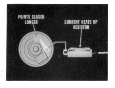
Now, if the ballast resistor ever fails, it will break the primary circuit to the coil. You can check for this failure possibility by connecting a jumper across the two resistor terminals to bypass the resistor. If the engine starts, then you'll know the resistor should be replaced.
