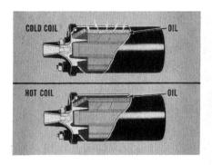
the engine might not start when cold. But with the ignition "on" and the distributor points closed, the oil can heat up and expand. That can fill up the air space, correct the internal short, and the engine will then start.
