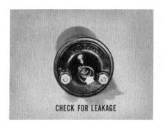
If you ever get a case where intermittent cold starting is reported, check for oil leakage at the tower terminal. If you find oil at that point, replace the coil.
