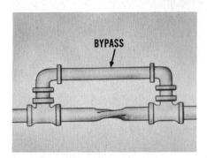
Just remember that you use a jumper to *bypass* parts of the circuit so you can close in on the section that may be at fault. It's a lot like using a pipe bypass in a water system.
