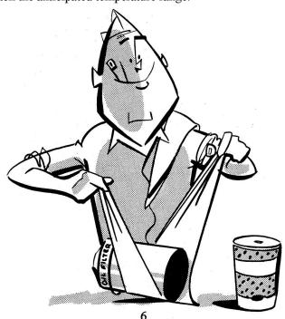
To replace the filter, unscrew it from the base. If the filter has taken a set on its mounting, it may be necessary to use Oil Filter
