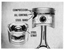
hole in the connecting rod is from .0007 in. to 0012 in. under the pin diameter. This method of fitting the piston pins prevents them from floating horizontally, even when hot, and eliminates the need for lock rings in the piston.
