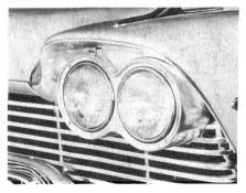
lamps on each side have only single filaments and operate only on the high beam. The outboard lamps on each side have two filaments and work on both high and low beams. These outboard lamps serve as the passing lamp and also supply the fill-in or supplementary light for high-beam operation.
