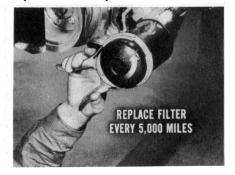
There may be instances where the oil filter may have to be replaced before the 5,000-mile change period. When the engine oil and filter are clean, the oil pressure gauge reading will be fairly high. However, if unusual operating conditions cause the filter to become clogged, oil pressure will gradually show lower readings. This can be used as an indication the oil and filter require changing.
