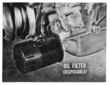
The oil filter is entirely new. It is a full-flow filter of the disposable type, and is mounted on the front face of the oil pump base. Engine oil capacity is four U.S. quarts. When the filter is changed, on extra quart of oil is required.
