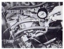
Start the engine and let it run until both it and the power steering fluid are at normal operating temperature. Fluid temperature should be about 175° F. Set engine idle at 475 to 500 r.p.m.
