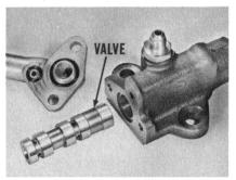
sure control valve end of the body so you don't have to remove the body end plug. Just unscrew the two pressure control valve housing screws, and separate the body and housing. The steering valve will slide easily out of the body, so don't drop it or the valve lands might get nicked.
