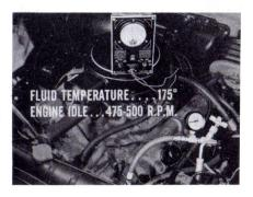
Now, gradually close the gauge valve. Pressure should rise to between 800 and 950 psi. Open the valve after making this test. If pressure is less than 800 psi, pump output is too low, and the trouble isn't in the gear. It's either in the flow valve, relief valve, or there's internal leakage in the pump.
