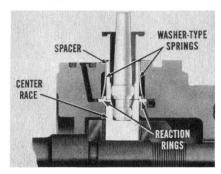
Two reaction rings keep the center race lined up with the spacer. These rings bear against the center race and spacer, and are mechanically loaded by two washer-type springs. Besides that mechanical force, there's hydraulic pressure in the picture.
