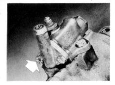
When you adjust the steering valve properly, returnability will be the same in both directions. Then, tighten the body attaching screws to 15 ft.-lbs., and you're done.
