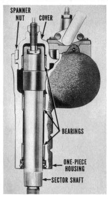
The sector shaft adjusting screw threads through a seal in the cover. A second seal between the cover and housing guards against any possible leakage. A seal and retainer are installed at the lower end of the sector shaft. They're held in by a snap ring.
