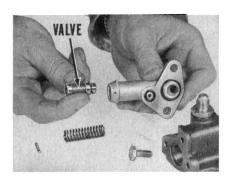
Pressure Control Valve. To remove the pressure control valve for cleaning and inspection, push the retaining pin from the housing. The spring and valve will slide out. If the valve doesn't slide out freely, check for burrs on the inside of the housing bore where the retaining pin enters. If you find any burrs, remove them
