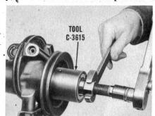
NOTE: When you assemble the puller to the pulley hub, see that the tapered ends of the two half collars fully engage the hub before you turn the puller screw.
