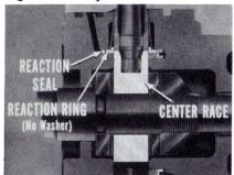
slightly different than with a left turn. On the lower side of the center race, for instance, there's a reaction seal and ring – but there's no compensation washer. As a result, there is more hydraulic pressure to resist center race movement on a left turn than there is on a right turn.
