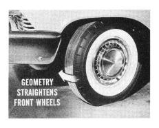
**Gear Resists Road Shock.** One good point in favor of power steering is that it's got a lot of built-in safety features. For example, if the wheel hits a chuckhole, or if a tire blows out, the shock of the wheel trying to change direction will be transmitted to the wormshaft.
