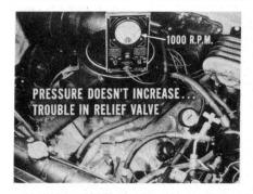
If your tests show that pressure is only slightly below standard, make this further test. Close the gauge valve and increase engine speed to about 1000 r.p.m. If the pump pressure doesn't increase noticeably, the trouble is in the relief valve.
