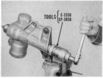
Install the new seal with its lip toward the roller bearings in the housing. Start the seal into the housing. Then, place the Adapter
