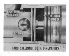
Poor Returnability. If a car has poor returnability in both directions, chances are it is caused by either incorrect front end alignment, low
