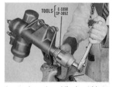
Steering Valve. You can service the steering valve while the unit's on the car. Disconnect the two hoses from the valve. Cap the ends to
