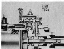
upper port wider. The lower port is closed off from the incoming fluid. Pressure increases in the pressure chamber *below* the piston flange, and the lower port becomes a return flow port to relieve pressure *above* the piston flange.
