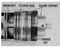
The wormshaft extends through the cylinder head, and through the steering column support at the upper end of the gear housing. A spanner nut holds the column support to the housing.
