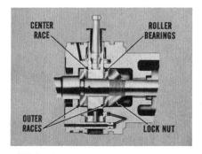
Think of that center race as being a part of a *thrust bearing*. The thrust bearing has two outer races, two sets of roller bearings, the center race and a lock nut holding the entire assembly on the wormshaft.
