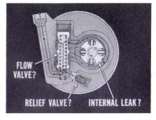
If your test shows *almost no pressure*, you'll have to repair or replace the pump, depending on the type of pump.
