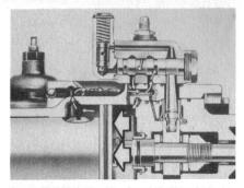
That movement, in turn, moves the steering valve. Pressure immediately goes to one side of the piston to prevent the front wheel from changing course. In support, power quickly comes to the rescue whenever there's a case of severe front wheel shock.
