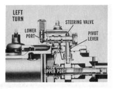
upper port to pressurized fluid coming in around the valve. Fluid through the *lower* port pours into the pump chamber *above* the piston flange. The *upper* port becomes a return flow port to relieve pressure in the chamber *below* the piston flange.
