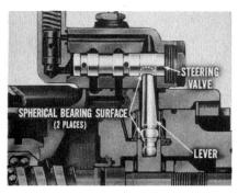
ment of the center race is used to control movement of the steering valve. This action will be explained later. The lower end of the steering valve pivot lever has a spherical bearing surface that rides in, and moves with, the center race.
