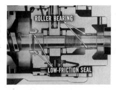
For instance, the shaft journal is fitted with a cast-iron seal ring.
