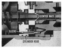
see, there is spring pressure, plus hydraulic pressure, resisting movement of the center race. It is this resistance that provides the "feel-of-the-road" characteristic.
