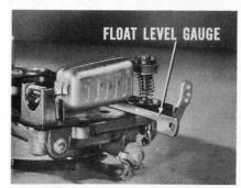
seated, check the float level. This is measured with the gauge (or a  $\frac{7}{32}$ " drill) placed between the outer end of the float and the gasket. If an adjustment has to be made, bend the float lever, close to the float. (Note: The float level for the front carburetor of a dual four-barrel installation is  $\frac{9}{32}$ ".)
