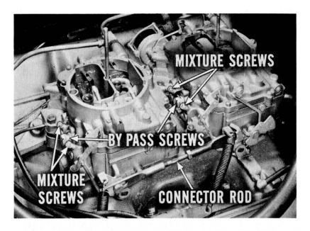
are properly synchronized. Next, you'll have to adjust the air bypass screws and idle mixture screws to get an engine idle speed of 600 r.p.m. and the smoothest possible idle operation. Here's how you go about it.
