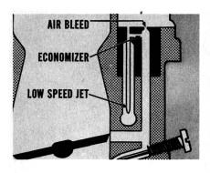
buretor, the low speed system functions in the primary barrels. Low speed jets are pressed into the primary venturi assemblies. Bypass air passages, an economizer and an idle air bleed built into the assembly function to break up liquid fuel and mix in the air before the mixture gets to the idle and low speed ports.
