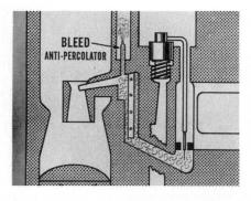
The high speed air bleed also serves as an anti-percolator vent. When a hot engine idles, or stops, vapor pressure in the idle well escapes through this vent. Otherwise, vapor pressure would build up in the idle tube and push fuel out of the nozzle and into the intake manifold, causing flooding.
