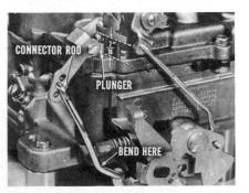
hole of the operating lever. This is the position for normal driving. There should be 7/16" from the air horn to the top of the plunger. Bend the connector rod at its lower angle, if needed. The outer hole provides a short pump stroke for summer driving. The inner hole provides a long pump stroke for winter driving.
