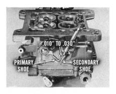
Adjust Secondary Throttle Valve Lock-Out. A secondary throttle valve lock-out, controlled by the choke rod, locks the secondary
