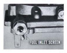
Make a visual inspection for presence of dirt in the float bowls. Then run your finger across the bottom of the float chamber and feel for dirt or foreign particles. If you see or feel any, remove the fuel inlet screen and inspect it for dirt. Inspect the float needle valves and seats, too. If the needles
