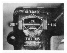
Inspect the clearance between the float lever tabs and the air horn lugs. The float should move freely on the pivot pin, but should not have excessive side movement that would permit it to rub on the sides of the bowl. This side clearance can be controlled by bending the float lever tabs.
