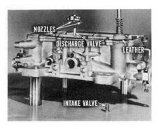
If service is needed, here are the main pump system points to keep in mind: leather in good condition, clean discharge nozzles, and no leakage at intake and discharge check valves. If dirt was found anywhere else, the intake and discharge check valves should be cleaned thoroughly.
