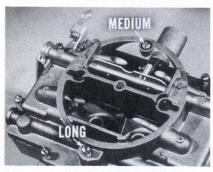
Ten screws secure the air horn to the main body. Eight are of the same length, one is slightly longer, and another is still longer. The mediumlength screw is in the counterbore, and the longer one is on the opposite side. Lift the air horn straight up so you will not damage the floats.
