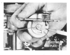
Adjust Fast Idle Cam Linkage. Hold the choke valve closed, and also see that the lugs on the inner and outer choke levers are in contact with each other. With these parts held as described, the end of the
