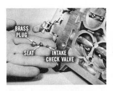
To do that, remove the brass plug, the intake check valve and seat from the bottom. The discharge check valve is under the pump discharge nozzles, which are removable. Clean up the checks and use a new gasket under the nozzles before you reinstall the parts.
