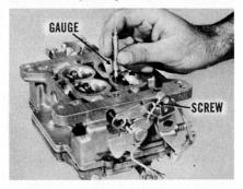
as described in the preceding paragraph. Then, turn the adjusting screw in or out until a .012" wire gauge will pass between the inner edge of the primary throttle valve and the bore of the barrel. With this clearance set at .012", the engine fast idle speed will be 1400 r.p.m.
