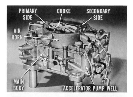
The carburetor functions as two two-barrel carburetors. There are two float systems, for example, each float serving one primary and one secondary barrel; two low speed systems (one for each primary barrel, since the secondary barrels do not function in the low speed range); two high speed systems—primary and secondary. The accelerator pump system takes care of both primary barrels, and the choke system applies to the primary barrels only.
