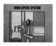
High Speed System. The high speed system supplies fuel for part and full throttle operation. The two front barrels contain the primary high speed system, and the two rear barrels contain the secondary high speed system. The flow of fuel to the main nozzles of the primary system is controlled by vacuum-operated step-up rods.
