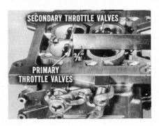
ondary throttle valves should just start to open when the primary throttle valves are open 3/8", measured between the edge of the valve and the bore. (On dual carburetor models 2652S and 2653S, primary throttle valve opening should be  $^{23}_{64}$ ".) If necessary, bend the connecting link to obtain this setting.
