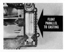
If the float is not parallel to the edge of the air horn you'll have to bend the float lever. Support the lever with your thumb to relieve the strain on the pivot pin, and use your forefinger to bend the float lever.
