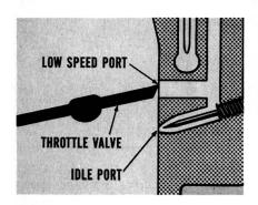
The low speed port is the slotted port just above the idle speed port. As the throttle valve opens it uncovers more of the port, allowing a greater quantity of the mixture to enter the barrels.
