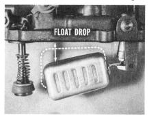
Remove and Install Baffles. Baffles in the float system help to maintain a stable fuel supply for the primary and secondary jets. If the baffles are removed when cleaning the carburetor, it is important that
