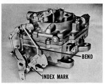
fast idle adjusting screw should be centered on the index mark on the fast idle cam. If it isn't, bend the lower end of the connector rod until it is centered on the mark. Then, in order to get the correct engine r.p.m. for fast idle operation, the fast idle adjusting screw setting will have to be checked.
