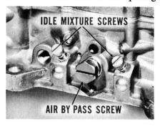
**Final Adjustments On Car.** Handling the final adjustment of dual AFB carburetors is simple enough if you follow the various steps in the proper order. The first thing you'll have to do is to adjust the throttle connector rod so that the throttles of the two carburetors
