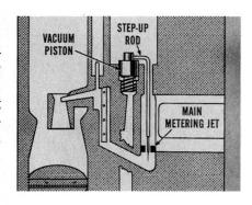
During part-throttle operation manifold vacuum is high. It pulls the step-up piston and rod down against a spring. This places the large diameter area of the rod in the metering jet, resulting in a reduced flow of fuel through the jet.
