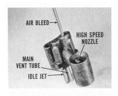
Remove the two screws which hold the primary venturi to the main body and lift out the venturi assembly. Inspect it carefully for presence of dirt, and clean it thoroughly so all passages and jets are free. Discard the gasket, because a new gasket should be used whenever the venturi is installed.
