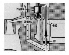
During wide-open throttle operation manifold vacuum is low. The piston spring overcomes the vacuum pull on the piston, and forces the piston up. The rod moves up until the small diameter area is in the jet. This permits an increase in the flow of fuel through the jet.
