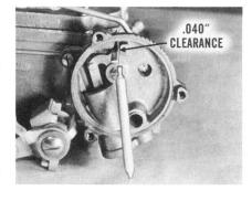
Adjust Crossover-type Choke. Remove the two bolts which hold the choke in its pocket in the manifold. Loosen the shaft nut, and turn the adjusting plate toward "lean" or "rich". You'll find "L" and "R" stamped on the cover. Reinstall the choke in the manifold, and tighten the retaining bolts.
