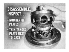
If you happen to find *more* than .020" total clearance, remove the eight case bolts and disassemble the unit. Note the number of clutch plates. There should be five. See if the thin,  $\frac{1}{16}$ ", tanged plate was stacked next to the differential case.
