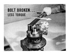
Now, tightening the bolt took effort because the bolt resisted your effort to turn it. But, if the bolt were broken suddenly so that the wrench began to *spin*, you'd be exerting *less torque*.
