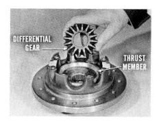
**Operation.** Under normal conditions, the Sure-Grip differential works a lot like the conventional unit. But when the rear wheels turn at different speeds, here's what takes place. Instead of dividing torque equally between the two wheels, the Sure-Grip differential sends the greater share of torque to the slower moving wheel.
