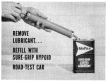
First, remove the lubricant and refill with the right amount of Sure-Grip Hypoid lubricant. Road-test the car to see if proper lubrication corrects the reported condition. Frequently, this is all that's needed.
