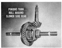
case. This, in turn, makes the pinions turn on their own shaft. They roll around the slower moving side gear. So the rotating pinions, in this differential action, allow the rear wheels to turn at different speeds while still keeping torque evenly divided between the two wheels.
