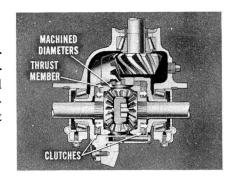
Both clutches, by the way, engage at the same time. In fact, any time there is torque applied to the Sure-Grip differential, the clutches are engaged to some degree. Differential action in itself doesn't actuate the clutches.
