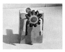
One important point to keep in mind is that each pinion is like a *balance* pivoted about its center. In other words, if you put one weight on one tooth, and another weight on an opposite tooth on the other side, the pinion would balance the weights like a small scale.
