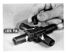
The axle shaft thrust spacer, which connects the two pinion shafts, is a two-piece part. It's fastened with a split, hollow lock pin forming a spool-like connection so a slight sidewise movement of the pinion shaft is permitted.
