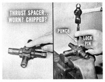
Carefully inspect the ramps in the differential case and on the pinion shafts. Replace both halves of the case if they are excessively worn. Replace the pinion shafts, too, if they appear to have bad surfaces where they contact the case ramps.
