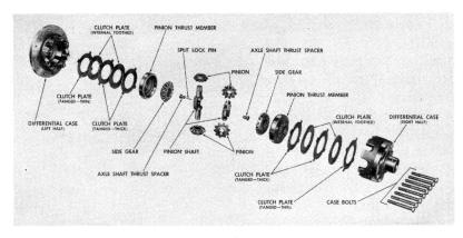
Now, before you go any farther, make a note of the index marks on case sections . . . and on the ends of the pinion shafts and their
