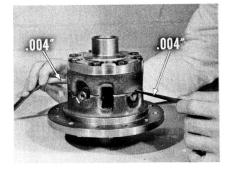
Then, increase the blade thickness until you get total clearance on one side. Invert the unit and check the clearance of the other pinion shaft ends in the same way. In addition to checking the total clearance, be sure there isn't more than .005" variation in clearance from one pinion shaft to the other.
