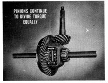
So the wheel standing on dry pavement can't get any more torque than the spinning wheel because of the equal torque division. Result? The car doesn't move.
