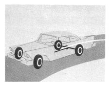
That wouldn't work out for an automobile. A single rear axle shaft would compel one rear wheel to slide—instead of roll—on curves or while traveling over uneven places in the road surface.
