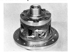
Once you remove the bolts and take off one half-section, you immediately see one of two packs of five clutch plates. Another clutch pack is on the bottom of this assembly.
