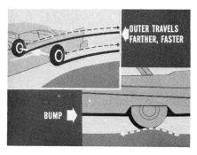
That's because the outer wheel, on a curve, travels farther and faster than the inner wheel. On a bump, or dip, one rear wheel acts the same way when it's compared with the wheel that rolls over a level surface. Even differences in tire air pressure will cause rear wheels to turn at different speeds.
