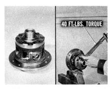
Before you reinstall the differential in the carrier, recheck total clutch plate clearance. This is always a good practice whenever the differential's been disassembled. If clearance is under .020", install the assembly in the axle housing. Fill the unit with Sure-Grip Hypoid Lubricant. Then, finally, road-test the car to be sure the condition has been satisfactorily corrected.
