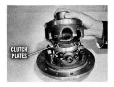
External tangs on three of the clutch plates fit into slots in the differential case. The other two clutch plates have internal teeth which engage external splines in the pinion thrust member. The clutching is done between the pinion thrust member and the differential case.
