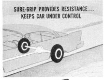
But if one wheel on that turn should hit loose gravel, or ice, and *try* to spin, Sure-Grip won't let it. Instead, Sure-Grip quickly provides resistance to prevent excessive one-wheel speed-up, and keeps the car under control.
