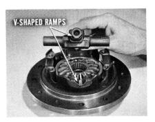
Both ends of each pinion shaft have two flat surfaces, or V-shaped ramps. These mate with identical ramps in the two differential case sections. One reason for marking the pinion shaft ends is to get them back on the same ramps during reassembly.
