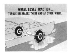
Something a lot like that happens when a rear wheel loses traction. Torque decreases at that wheel, and also at the other wheel because of the equal torque division provided by the differential. Speed of the spinning wheel increases, but not the torque.
