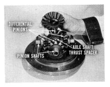
Right under the pinion thrust member is a differential side gear, like the side gear in a conventional unit. And when you lift the differential gear, you see four differential pinions. These pinions are on two pinion shafts that are loosely connected at right angles to each other by means of an axle shaft thrust spacer.
