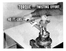
Definition of Torque. Torque, as you probably know, is a force—a "twisting effort". As an example, you'll remember putting a torque wrench on a bolt and tightening it until you get a certain reading—let's say the indicator points to 40. Said another way, you've tightened the bolt to 40 footpounds.
