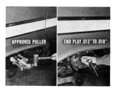
But if proper lubrication isn't the remedy, then use an approved puller (never a knockoff type, as it may cause damage) to pull the wheels. Check axle shaft end-play. It should be .013" to .018". Readjust end-play, if needed, and again road-test the car.
