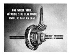
The side gear on the spinning axle turns faster because the pinions are turning on their shaft. The extra *speed* of the pinions is added to the side gear, in addition to the *speed* of the case. So, the free axle of the wheel with no traction turns exactly twice as fast as it would when both wheels have the same traction.
