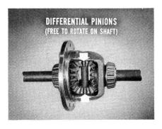
Surrounding those side gears is a cast housing, called the differential case. Pressed into this case is a small differential pinion shaft. Mounted on this pinion shaft are two smaller gears called differential pinions. These pinions are free to rotate on the pinion shaft which is held stationary in the differential case.
