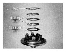
Follow the thin plate with an internal-tooth plate. Alternate for five plates in all—three with tangs, two with internal teeth—and be sure the thin plate remains as the outer plate to go next to the case.
