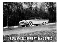
Now, when engine torque drives the axle drive gear around, the case turns with it and carries the pinions around. But, since both rear wheels turn at the same speed, the gears and pinions inside the case don't turn on each other. In other words, the pinions don't turn on their own shaft. Instead, they're in balance!
