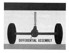
the single rear axle shaft was replaced by two short shafts. Then, the conventional differential assembly was developed and placed between the two axle shafts. What this differential does, and how it does it will help you understand Sure-Grip operation. So let's take a look at how the conventional differential operates.
