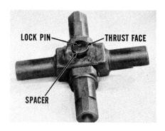
Now, when you assemble the pinion shafts, drive in the lock pin until it shows at, but not beyond the thrust face. The thrust spacer should be a loose fit so it will let the shafts separate to actuate the clutches.
