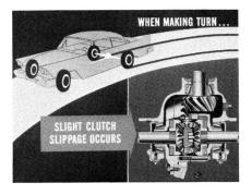
Operation—Car on Turn. Now, when a car equipped with the Sure-Grip unit is making a turn, a slight amount of clutch slippage occurs. This limited slippage is equal in each pack. In this way, differential action is allowed to take place to let the outer wheel on the turn travel a greater distance at a faster rate of speed.
