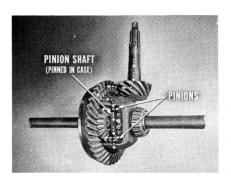
Now, the axle drive gear is bolted securely to the differential case. So, the gear torque passes directly to the case. Since the differential pinion shaft is pinned in the case, the torque is taken by the pinion shaft and applied to the bores of the differential pinions as a force.
