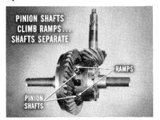
one wheel on ice and the other wheel on dry pavement. When an attempt is made to drive the car, drive gear torque in the differential case will cause the pinion shafts to climb the case ramps. The pinion shafts will separate, as allowed by the axle shaft thrust spacer.
