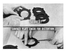
Scored or galled surfaces, of course, mean plates are damaged. A surface plate check will show up any distortion. Discard any damaged or distorted plates.
