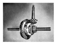
They act as balance wheels, pivoted about the center, and apply equal force to the side gears. As a result, the side gears turn at the same speed as the case. In fact, the whole nest of gears turns as if it were one solid unit. It goes through the same motion that would take place if there were a solid rear axle.
