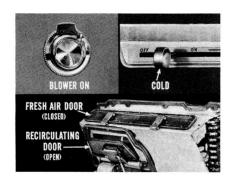
Check the Controls. Make a brief check of the controls next. Turn the blower on. See if it delivers plenty of air. Then, start the engine. Put the temperature control lever in "COLD" position. The freshair door should be closed, the recirculating door open.
