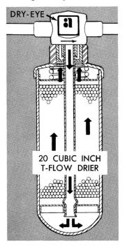
Here's another way to dry the system and leave the factory-installed drier attached. Purge the system of refrigerant. Remove the sight glass and install a super dry-eye, which is a combination dry-eye and sight glass. Also, install a 20 cubic-inch T-flow drier, making sure the arrow on the dry-eye points toward the direction of refrigerant flow. Tighten the drier into the dry-eye only 8 to 12 foot-pounds torque! Any more torque than that might crack the gasket. Evacuate and recharge the system.
