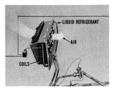
Evaporator. The evaporator works like a radiator in reverse. It has a lot of coils through which liquid refrigerant flows. Air is directed over the coils. Liquid refrigerant flowing inside the coils absorbs heat from the air that is circulated over the coils. As this heat is absorbed, the liquid changes to a gas.
