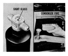
While the unit runs, inspect the sight glass. Bubbles mean a low refrigerant supply. Take a look at the condenser fins, too. If they're cluttered up with bugs, brush them off so air flow won't be restricted.
