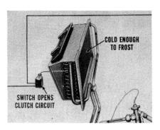
pressor, which stops the flow of refrigerant. As the evaporator warms up, the thermal switch closes the circuit and engages the clutch. The compressor starts running, and the system begins to function again. Knowing that will help you understand why the thermal switch occasionally requires testing.
