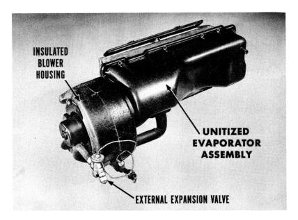
This new construction provides improved sealing and insulation for both the evaporator assembly and blower housing. It minimizes hot air leak possibilities, which means an increase in cooling. Only one joint remains to be sealed. It's the seam between the flange of the unitized assembly and the dash panel.
