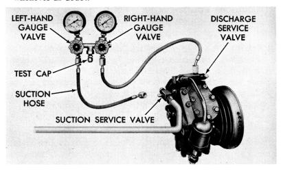
Disconnect the suction hose from its service port. Slowly close the left-hand gauge and watch discharge pressures and tachometer. At exactly 500 r.p.m. pressure should build up slowly to the figures listed in the following table. Open and close the left-hand valve several times to allow pressure to drop and build up, and recheck your readings.
