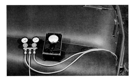
Operate the engine at 1200 r.p.m. with the *hood down* to keep hot engine compartment air from entering the cowl vent opening. Set the temperature control lever to COLD and the selector switch to COOLING.
