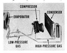
the evaporator, compresses it, and sends hot, highly pressurized gas to the condenser. The compressor, then, must have the ability to deliver adequate volume and pressure under all operating conditions. Knowing how to make an accurate compressor capacity test, therefore, is important.
