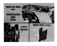
Checking what happens with the temperature control on "COLD" and 3/8" to right of COLD will tell you whether they are doing their job. It's not a complete check, of course, but you'll know the controls are doing what they should to provide maximum fresh and recirculated air cooling.
