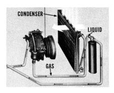
Condenser. At the condenser, heat from the compressed refrigerant gas is transferred to outside air flowing through the condenser fins. In this process, the refrigerant is condensed. It changes from a gas to a liquid. Unrestricted air flow around the fins is vital if the condenser is to do its job.
