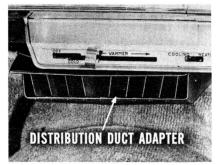
blower has been increased about 15%. This means more cool air is delivered inside the car. Besides the boost in blower output, a distribution duct adapter is used for more effective air distribution. It's an addition to the air duct. It directs cool air better, especially to the rear compartment.
