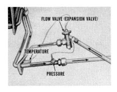
When you test a valve on a 1955 or 1956 system, the normally open hot gas solenoid by-pass valve must be energized. This will prevent flow of gas from the discharge to the suction side. Run a hot lead from the battery to the solenoid terminal to energize the valve.
