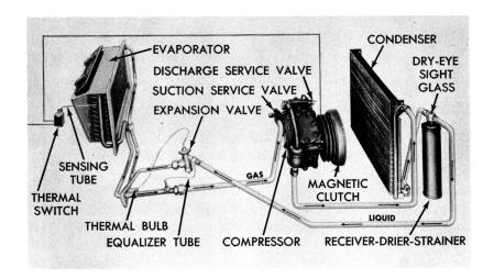
Compressor. Take the compressor, for instance. It pumps refrigerant through the system. It pulls refrigerant gas under low pressure from
