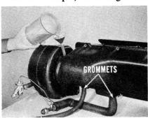
remove the blower rubber coupling. Pour in about a pint of water, and watch for leaks at the grommets along the bottom. A stream of water means there are leaks. Use heavy body sealer at the grommets and around the entire outside edge of the housing to correct any leaks you may discover.
