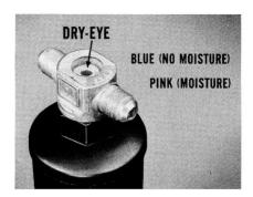
**Dry-Eye.** On models that use a combination "dry-eye" and sight glass, a *blue* element means no moisture is in the system. But a *pink* element means there is excessive moisture in the system, and you'll have to correct this condition before you go to other tests.
