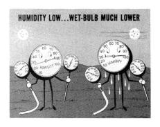
When humidity is low, the wet-bulb reading will be much lower than the dry-bulb reading. If humidity is high, wet-bulb and dry-bulb temperatures will be closer together. In fact, when wet-bulb and dry-bulb temperatures are exactly the same, you'll know relative humidity is 100%.
