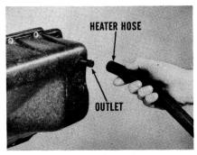
**NOTE:** If the engine's hot, and the cooling system is under pressure, coolant may pour out of the hose and surprise you. So, make the water valve closing test with the radiator cap off, and *before* the engine gets hot.
