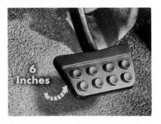
If the pedal doesn't have proper travel, check for interference between the clutch pedal and the clutch pedal rod—the perpendicular
