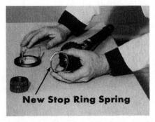
When assembling the synchronizer, use the new thinner, lighter load stop ring spring, part number 1823916. This new spring improves shifting into second, and will prolong the life of the synchronizer.
