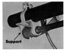
Just loosen the lower support (two clamp bolts on early models, a single clamp bolt on later models) and tap the support up or down. When the proper clearance has been obtained, tighten the clamp bolts. If you are working on a "K" Series manual steering job,
