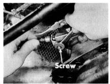
**Checking Fluid Pressure.** Conditions due to incorrect hydraulic pressure will not be confused with mechanical conditions if pressures are checked first, before disassembly is attempted. It's a lot easier to check pressure than to drain the transmission and remove the valve body or perform other mechanical operations which may not be necessary.
