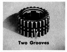
two grooves instead of the single groove of the former gear. This new gear can be used for replacement in any transmission using the pin-type synchronizer. If you install the gear only, be sure to use the new, lighter-load synchronizer stop ring spring, part number 1823916.
