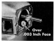
shift the dial indicator farther out on the arbor so the dial contact arm rests on the face of the housing. Again, rotate the flywheel and read the total runout of the face of the housing. A total runout of .003 inch is the limit—more than that calls for a correction.
