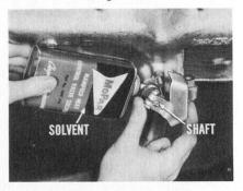
**NOTE:** If the shaft is stuck tightly, tap the ends of the shaft *lightly* with a hammer to break it loose (after solvent has been applied). Then rotate further to free it up.
