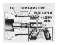
letters following (alphabetically). You can't install this new boot on earlier units because there's not enough space between the support and jacket. But if you replace the housing or power unit with later production parts, the new boot and ground strap can be used.
