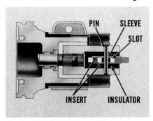
coupling and remove the tube. Enlarge the slot to 3/8" and round the upper and lower corners. Secure a piece of rubber tubing 3/8" O.D., 3/16" I.D. Cut a 1/4" section for use as a sleeve. Put the sleeve in the slot. Assemble the two plastic inserts and rubber tube insulator in the coupling. Then, install the pin.
