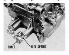
strong enough to overcome any slight sticking or resistance on the part of the throttle valve assembly. You can check this by removing the air cleaner and observing throttle opening. If valves are positioned properly, and the shaft doesn't bind, install a new, stronger flex spring (Carter No. 61-623).
