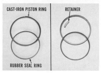
New Piston Ring Package. There are two cast-iron piston ring packages available for service, under Part No. 1879745. One package has the cast-iron ring and a synthetic rubber seal ring; the other contains the piston ring and seal ring, plus a retainer which fits on the piston ring to protect the seal ring.
