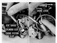
enters the slot in the cylinder. (A .026" step-up wire used on BBD carburetor can take the place of the gauge if one is not available.) Push the choke lever clockwise to trap the gauge between the piston and cylinder slots, leaving the choke linkage free.
