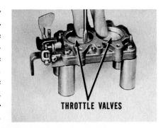
Fast-Idle Adjustment. This adjustment has to be high enough to keep the engine from stalling during warm-up. To check it, remove the air cleaner. Partially open the throttle valves to release the fast-idle cam. Close the choke by hand. Hold it closed, and release the throttle valves.
