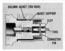
too high on the jacket support of the power unit. When that happens, the slot in the lower end of the steering tube bottoms on the tube connector pin. This pin must be located in the slot so it will allow a slight up-and-down movement of the wormshaft. This is the movement that controls valve operation.
