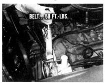
be free from oil and grease. And on the current Plymouth model, for example, the belt should be tightened to 50 footpounds torque. All belts, by the way, should be tightened at the regular inspection period — 1,000- or 2,000-mile — depending on the model.
