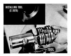
Use the installing tool C-3676 to install the new rings on the piston. Lubricate them with type "A" automatic transmission fluid. Then, install the piston and wormshaft assembly into the housing carefully so the rings won't be damaged.
