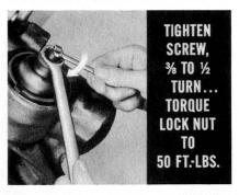
Finally, turn the adjusting screw in  $\frac{3}{8}$  to  $\frac{1}{2}$  turn. Torque the lock nut to 50 foot-pounds, and you're done.
