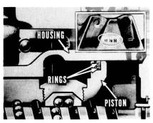
The most recent change in the power steering unit consists of a new housing, a new piston, cast-iron piston ring, and synthetic rubber seal ring. Units with these parts are identified by the letter "H", or letters following alphabetically, stamped between the mounting bolt holes.
