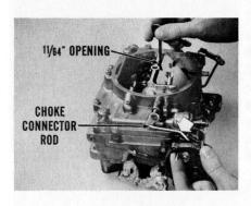
Bend the choke connector rod at the upper angle to provide an  $^{11}\!\!/_{\!64}$ " opening between the choke valve and the wall of the air horn. Check this with Unloader Gauge T-109-166. Finally, remove the gauges. Reassemble the choke. Set the thermostatic coil cap one notch rich, and reinstall the throttle return spring.
