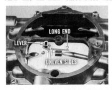
AX, you can remove the cotter pin from the choke lever. Take a ½16" diameter wire about 1¾" long. Put one end through the two holes in the lever so it sticks out about ½8" on the short end. Bend the long end of the wire around the bottom of the lever to form a "U" with uneven sides. Remove the wire.
