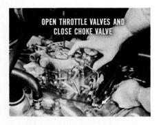
That should move the fast-idle cam to the position giving the cor-
