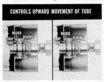
assembled *under* the jacket bearing, or if the washer is missing. The washer, which is assembled between the snapring and lower end of the jacket bearing, controls upward movement of the tube. It also maintains proper clearance between the steering wheel hub and top of the column.
