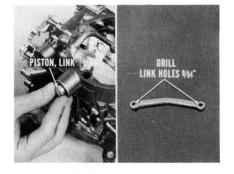
**NOTE:** Remember, installing the wire applies *only* to crossover chokes with AX identification on the cover. Enlarging the holes can be done on either AX or AU chokes.
