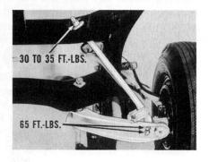
Occasionally, front shock absorbers make a noise similar to chuckle when they're cold. This condition is normal, and is easy to identify because the noise disappears as soon as the shock absorbers warm up.
