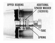
Lack of "Feel-of-the-Road". This can happen if the reaction area parts are installed in the wrong sequence when the power unit has been disassembled for service. So, if you get a report of this condition,
