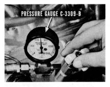
If belt tension is up to specifications, and is free from oil or grease, install Pressure Gauge C-3309-B. See if pump maximum pressure is up to specifications. As these pressures vary for different models, consult the table below.
