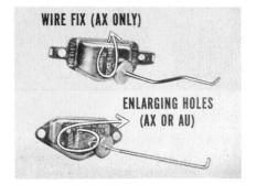
On the integral type choke, remove the retainer ring, cap, and thermostatic coil. Remove the throttle return spring, and set the throttle ¼-open. Let the choke valve go wide open.
