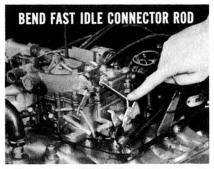
To make such an adjustment, get the fast-idle cam in the proper position first. You may have to bend the connector rod at the angle until the index mark lines up with the screw. Then, you'd adjust the screw to get the correct fastidle speed.
