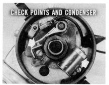
Why Ignition Points Burn. If points are set too close, they'll burn. The condenser won't be able to do its job of soaking up enough of the current to prevent arcing. Oil or grease on the points can also make them burn. So can a defective condenser cause burned points.
