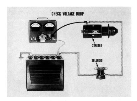
Starter Cable and Switch Tests. Use a voltmeter to check voltage drop in the starting circuit. But first ground the ignition primary circuit to keep the engine from starting. Connect the ground jumper on the distributor side of the ignition coil.
