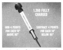
Remember that specific gravity of the electrolyte will vary 4 points (.004) with every 10°F. change in temperature. Subtract 4 points for each 10° below, add 4 points for each 10° above 80°F. Correct your readings to 80°F. before making a final interpretation.
