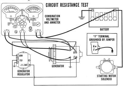
Reconnect the battery and start the engine. Slowly increase speed until 10 amperes register on the ammeter. You shouldn't read more than .5 volt on the voltmeter. If voltage reads higher, check for either a bad connection between the voltmeter leads, or for burned relay points. A higher reading, by the way, shows a need for making a point-to-point voltage drop test.
