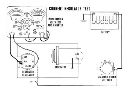
Start the engine and increase its speed to 2000 r.p.m. Adjust the rheostat (variable load) until the current regulator settles at a steady ampere output. This should meet the following specifications within plus or minus 2 amperes. Temperature should be taken 2" from regulator cover.
