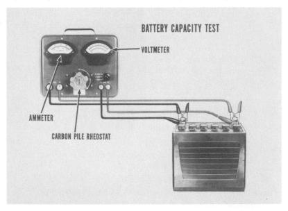
Adjust the rheostat control knob until the ammeter shows 200 amperes. This puts a good load on the battery. Let the battery discharge at this rate for about 15 seconds. Then, with the battery discharging at 200 amperes, read the battery voltage. If it's 9.5 volts or more, battery capacity is okay.
