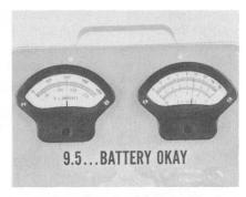
If a battery doesn't pass the capacity test, you'll have to slow-charge and retest it to find out if it can be saved. Another thing, if a battery tests less than 1.225 or is cold—below 70°F.—don't make a capacity test because the results would be meaningless. In either case, install a good battery in the car before making any further tests.
