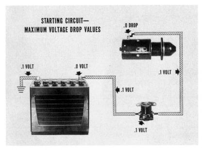
Maximum voltage drop across each part of the circuit should not exceed .1 volt for each cable, .1 volt for the switch, and there should be .0 volt (no drop) at the terminals and connections.
