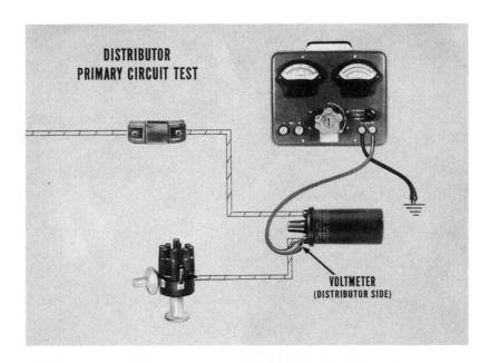
With the ignition turned on, and the breaker points closed, read the voltmeter. Voltage drop should not be more than .1 volt. If you see more than .1 volt, you'll know that something's not up to snuff in the distributor. There may be burned points or a loose connection. Since you have made sure the trouble is in the distributor, it should be removed for bench tests and inspection.
