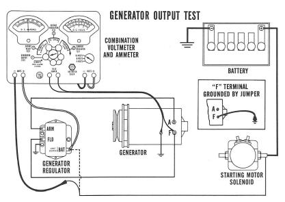
Start the engine and gradually increase engine speed. The standard equipment generator should produce the rated output at 1500 to
