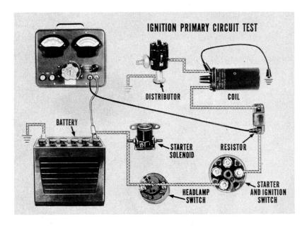
To check voltage drop, set the voltmeter selector switch at the 4-volt position. Connect the positive voltmeter lead to the positive battery post. Connect the negative voltmeter lead to the ignition switch side of the ballast resistor.
