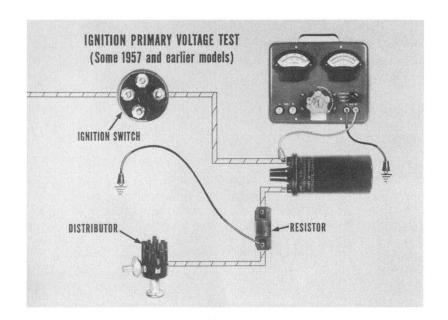
If you connected the jumper to the coil side of the resistor, current would be too high. That's because the resistor wouldn't cut down the current, which would really "French-fry" the ignition wiring.
