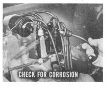
Besides that, you'd check for a burned rotor, or arcing at the terminals inside the cap. If you find those points okay, you'd check the wires and spark plugs . . . burnt electrodes, wrong gap, etc.
