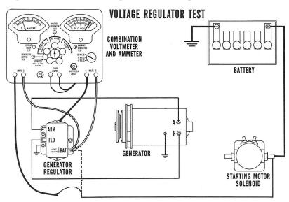
Start the engine and let it run at 1500 r.p.m. Take temperature readings with the regulator cover in place. Hold an accurate thermometer 2" from the cover and see if the voltage readings follow those listed in the following table:
