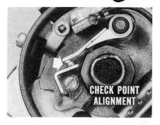
Also, if the points aren't lined up properly, they'll burn on one edge because the reduced contact area won't be able to dissipate heat properly.
