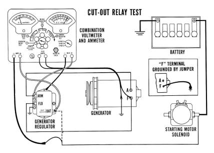
If this test immediately follows the voltage and current regulator tests, you won't have to normalize regulator temperature. But if the regulator's cold, you'd better normalize it.
