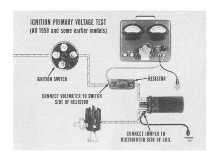
On 1958 models, along with some 1957 and earlier cars, the ballast resistor is between the ignition switch and coil. As a result, you must connect the positive voltmeter lead to the switch side of the resistor. If you connected the voltmeter to the coil side, the resistor would drop the voltage. That would give you a low-voltage reading that would be misleading. So, whenever the resistor lies between the switch and coil, put the positive lead on the switch side of the resistor.
