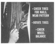
inspect the tire wear pattern; it's a good clue to a need for front-end alignment. Before lowering the car, rotate the tires, check tire inflation and then check wheel balance. If you noticed any tendency of the car to wander while out on the road, it could have been due to low tire pressures.
