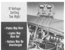
nition points may burn, lights may burn out, and the battery may become overcharged and require water too frequently. If the regulator setting is too low the battery will run down. In other words, proper generator regulator operation is necessary to keep the battery in a good state of charge.
