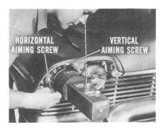
To aim the headlamps vertically, turn the vertical adjusting screw counterclockwise to bring the bubble on the spirit level to the car side of center. Then, turn the screw clockwise to center the bubble and eliminate backlash. Recheck each lamp. Readjust, if necessary, and remove the aimers.
