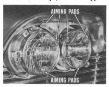
into the lens at the top. Each outboard lamp has two filaments—one for low, the other for the upper beam. It's the low beam that you'll be aiming. The upper beam is an "off-focus" filament which provides body light for illuminating the side of the road, ditches, and signs, and sort of fills in the low beam.
