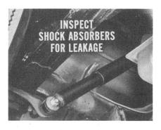
Inspection. While you're under the car, inspect the shock absorbers for fluid leakage. A slight amount of wetness is okay. But if it looks as though the shocks are leaking, it means that seals at the top and lower sections of the unit are worn, and the shock absorbers must be replaced. Badly leaking units cannot be repaired.
