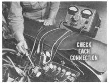
use the voltmeter to test for circuit resistance. Check each connection for looseness or corrosion, especially the battery and starter cables. Also, inspect connections at the solenoid. There should be no more than .1 voltage drop per cable or switch, and zero drop at the battery and starter terminals.
