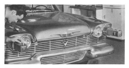
Checking Headlamp Aim. If the headlamps are merely to be checked for aim, you don't have to remove the headlamp doors. Just clean the lenses and attach the aimers to both outboard lamps. See that the side sight openings on each aimer point toward each other, as shown. Turn the right-left aim knob until the split image is in alignment. If the *horizontal* check exceeds the values listed below (representing inches at 25 feet), you'll have to aim the lamps.
