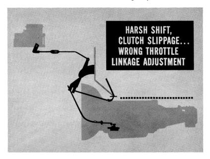
The amount of engine torque transmitted through the converter and into the transmission is directly related to throttle opening. The throttle linkage acts on the throttle valve in the transmission valve body, so that throttle pressure increases in proportion to engine torque. So, shift *timing* and shift *quality* are affected by throttle opening.
