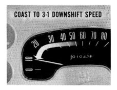
Let the car coast down until you find the speed at which the 3-1 downshift is made. Do this again. But just before the unit makes the downshift, accelerate rapidly with ¾-throttle. If the engine races because engine speed increases faster than car speed, the rear clutch is slipping.
