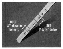
10 miles and the fluid is thoroughly warmed up, the level should be at the FULL mark—or ½" below. **NOTE:** If the car's been driven over a *long* distance at high speeds, and the level is checked as soon as the car stops, the level might rise to about ¼" above the FULL mark.
