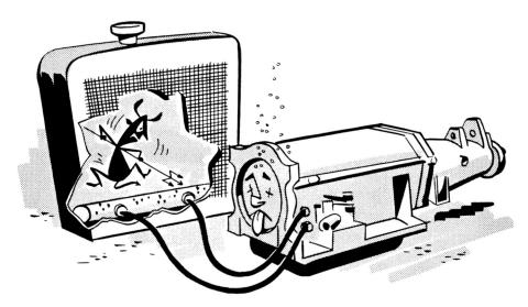
Antifreeze in Transmission Fluid. If you find antifreeze in the transmission fluid, check for a leak in the cooler at the bottom radiator tank. Disconnect the cooler lines and use air pressure (no more than 50 pounds) to test for cooler leaks. If you find a leak, remove the cooler for repair.
