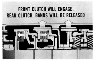
Now, accelerate with 3/4-throttle. If car speed responds quickly, without engine runaway, you'll know the front clutch is okay.
