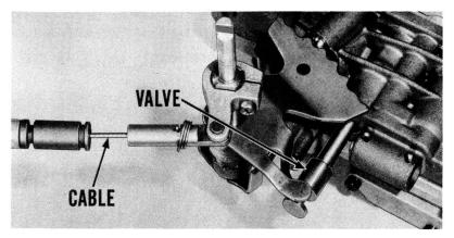
The manual valve, remember, is positioned by the push-button cable. So if the manual valve is improperly positioned, flow of fluid through the valve will be reduced. In short, when the flow to the apply pistons is reduced, the transmission won't perform as it should. That's why the cable adjustment must be checked before even thinking about disassembly of the unit.
