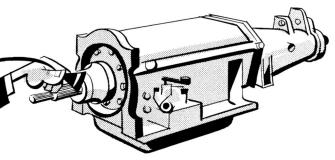
Front Clutch Test. With the engine idling, and the car standing still, engage the "D" button. The front clutch will engage. The rear clutch as well as both bands will be released. The transmission is in low gear or "breakaway" and any slippage experienced will be in the front clutch.
