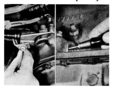
the "R" button all the way in to remove free-play at the button box. Next, loosen the screw holding the cable adjustable bracket to the adapter housing. Remove the neutral starter switch. Use a screwdriver to hold the manual valve lever in reverse detent position.
