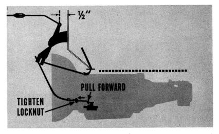
Then, with the bell-crank-lever-to-dash-panel clearance correct, adjust the length of the throttle rod so it can be connected to the carburetor throttle lever without moving the lever.
