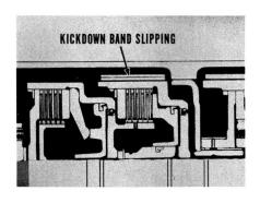
A kickdown band that's too tight can cause a harsh 2-3 upshift, and a harsh 3-2 kickdown. Check the 2-3 upshift at half-throttle. The upshift at half-throttle opening should be very smooth if the band and throttle linkage adjustments are correct. If, however, the upshift is noticeably harsh at half-throttle, the kickdown band is very likely too tight, and should be adjusted.
