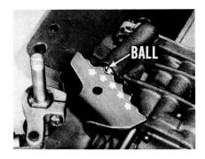
NOTE: If all pressures check out okay, but there still seems to be some slippage, double-check the push-button cable adjustment. You may have to remove the oil pan to make sure the ball seats properly in each detent!
