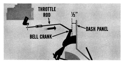
Next, move the throttle rod rearward to the limit of its travel. There should be ½-inch clearance between the rear edge of the bell crank and the dash panel. With the bell crank in that position, the end of the throttle rod should line up with the carburetor throttle lever without moving the lever from idle position.
