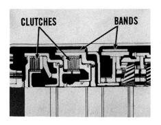
Inside the transmission, the flow of power is controlled by two multiple-disc clutches and two bands. When these clutches and bands do what they're designed to do, the transmission works beautifully. But if a band happens to slip—or grab—or if a clutch slips—operation won't be normal.
