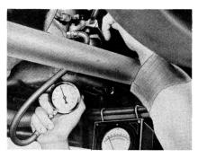
Line Pressure. Connect a tachometer to the engine. Remove the pipe plug from the line pressure take-off hole (on the left side of the transmission just below the push-button cable ferrule). Install a 300psi gauge (C-3293). Line pressure readings and pushbutton positions are in the table below:
