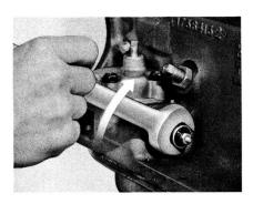
Turn the switch in until the washer contacts the case. Then, tighten the switch an extra ½-to ½-turn. Turning it in any farther will affect the cable adjustment. Finally, connect the wire and check neutral switch operation.
