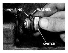
Next, clean the switch contact surface on the transmission so the switch will have a good ground. Install the mounting washer with the concave surface away from the switch. Place the rubber "O" ring next to the washer, and install the switch in the case.
