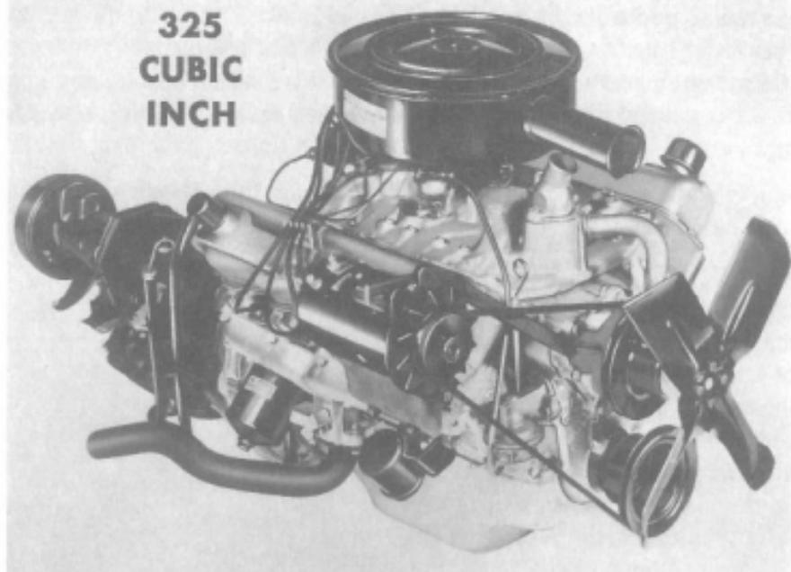
**Red Ram V-8.** This engine, found in Coronet models, is a new 325-cubic-inch engine. It uses hydraulic tappets. Some of the earlier production engines may have adjustable rocker arms, even though they have the hydraulic tappets. If you'll remember that, you won't be tempted to try adjusting the tappet clearances just because you find adjustable rocker arms.
