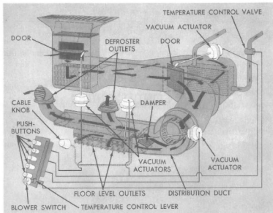
The air-conditioning unit is operated by push buttons located on the instrument panel. The buttons select the degree of air conditioning desired—Maximum Cooling, Fresh-Air Cooling, Defrosting, etc.—while a sliding lever in the same panel permits selection of the temperature desired. The lever operates the temperature control valve.
