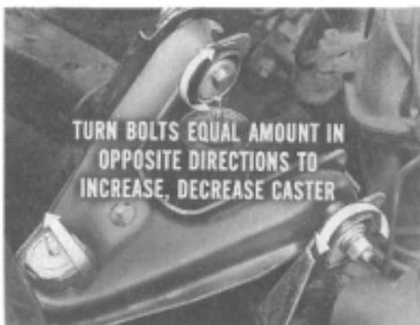
When the proper adjustment has been reached, hold the bolthead with one wrench while you tighten the nut to 65 ft.-lbs. torque. Recheck caster and camber before leaving the job.
