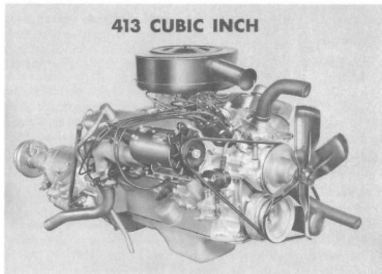
**Golden Lion 413.** This new V-8 engine, with a displacement of 413 cubic inches, is used with a four-barrel carburetor as standard equipment in the Chrysler New Yorker models. It has a bore of 4.188 inches, and a stroke of 3.750 inches. Compression ratio is 10 to 1, and ignition timing is set 10 degrees Before Top Center. Premium fuel is required.
