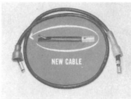
Because of the construction of these cables, care must be exercised in removing the terminals from the spark plugs or from the distributor cap towers. If you yank the cable in an attempt to remove it, you may stretch the cable and thereby increase the built-in resistance—or you may pull the cable out of its terminal. So, disconnect the cable by grasping the terminal boot—not the cable itself.
