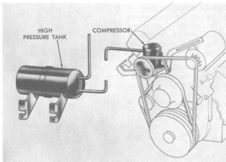
A belt-driven air compressor is mounted on the engine, and a high-pressure tank is mounted at the right front end of the frame.
