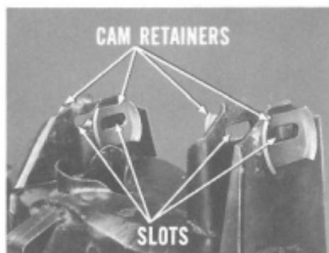
Welded to the outer face of each support bracket is a cam retainer. Horizontal slots are provided in the support brackets to allow for movement of the adjusting bolt.
