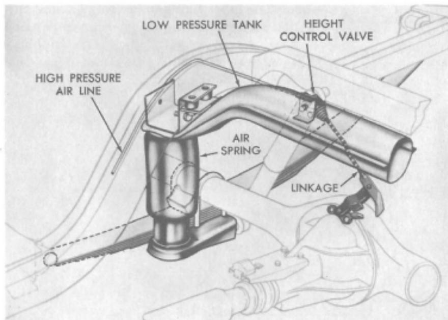
The high-pressure tank is connected to a low-pressure tank at the rear of the car. Also at the rear are two air springs, a height control valve, and the necessary linkage.
