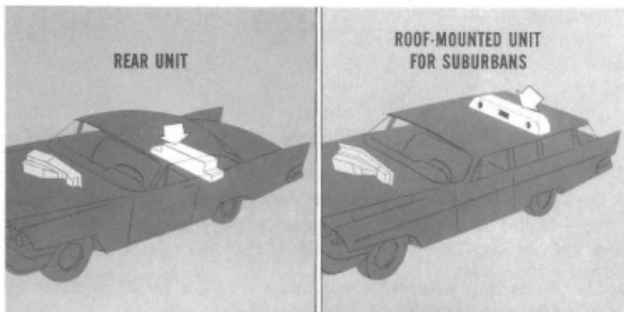
The front unit can be used to operate by itself, or in conjunction with the rear unit, or with the roof-mounted unit. The rear unit can be installed *instead* of the front unit, or *with* it, to supplement the operation of the front unit. The roof-mounted unit for suburban installa-
