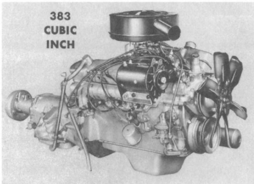
**Turboflash 383-cubic-inch V-8.** This is a new V-8 engine, and is used with a two-barrel carburetor as standard equipment on the Fire-dome models. It has a bore of 4.250 inches and a stroke of 3.375 inches. It has a 10 to 1 compression ratio, and ignition timing is set 10 degrees Before Top Center.
