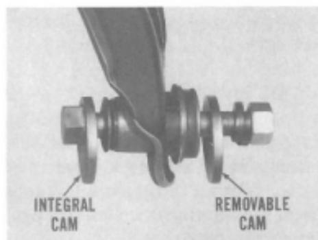
Integral cams are welded under the head of each bolt, and removable cams are installed over a flat section of the bolt at the threaded end. These cams operate in the cam retainers welded to the support brackets.
