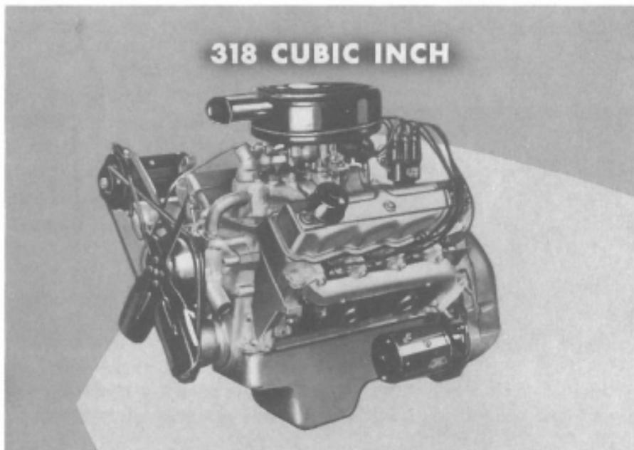
**Fury V-800.** While the displacement of this engine—318 cubic inches—remains the same as for the “L” Series, there are a number of improvements which will increase its performance. For instance, the high-performance camshaft used in the Super Pak job “L” Series is now standard in this engine. It holds the valves open for 244 degrees,
