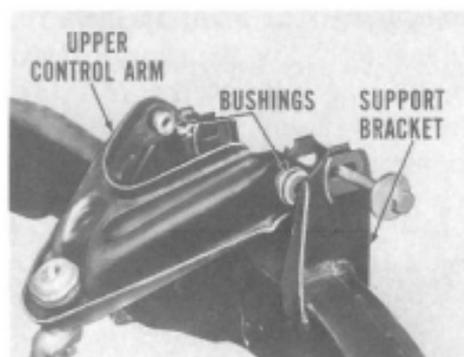
The upper control arm is new, and its inner ends are mounted in new supports welded to the frame.
