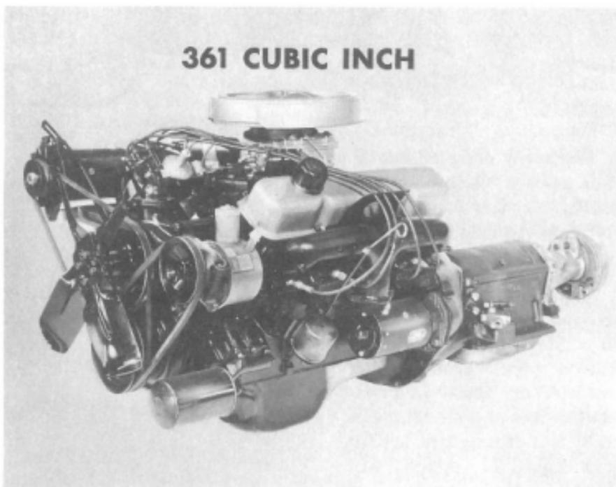
**Golden Commando.** The Golden Commando V-8 engine is larger than for the "L" Series. It has a displacement of 361 cubic inches, and a compression ratio of 10.1 to 1. The high-output camshaft holds
