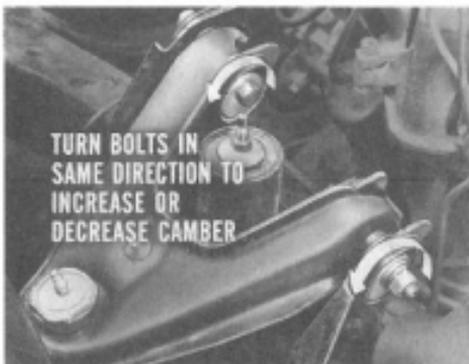
By turning the front and rear bolts an equal amount, but in *opposite* directions, the ball-joint end of the arm is moved toward the front or rear of the car, thereby changing caster. Since bolts are turned an equal amount, there is little or no change in the camber setting.
