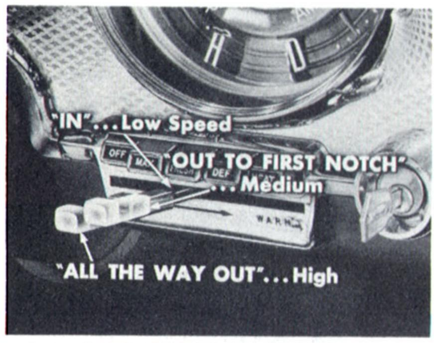
The three-speed switch provides low speed when the lever's pushed in; pulled out to the first notch is medium speed. All the way out is high speed.
