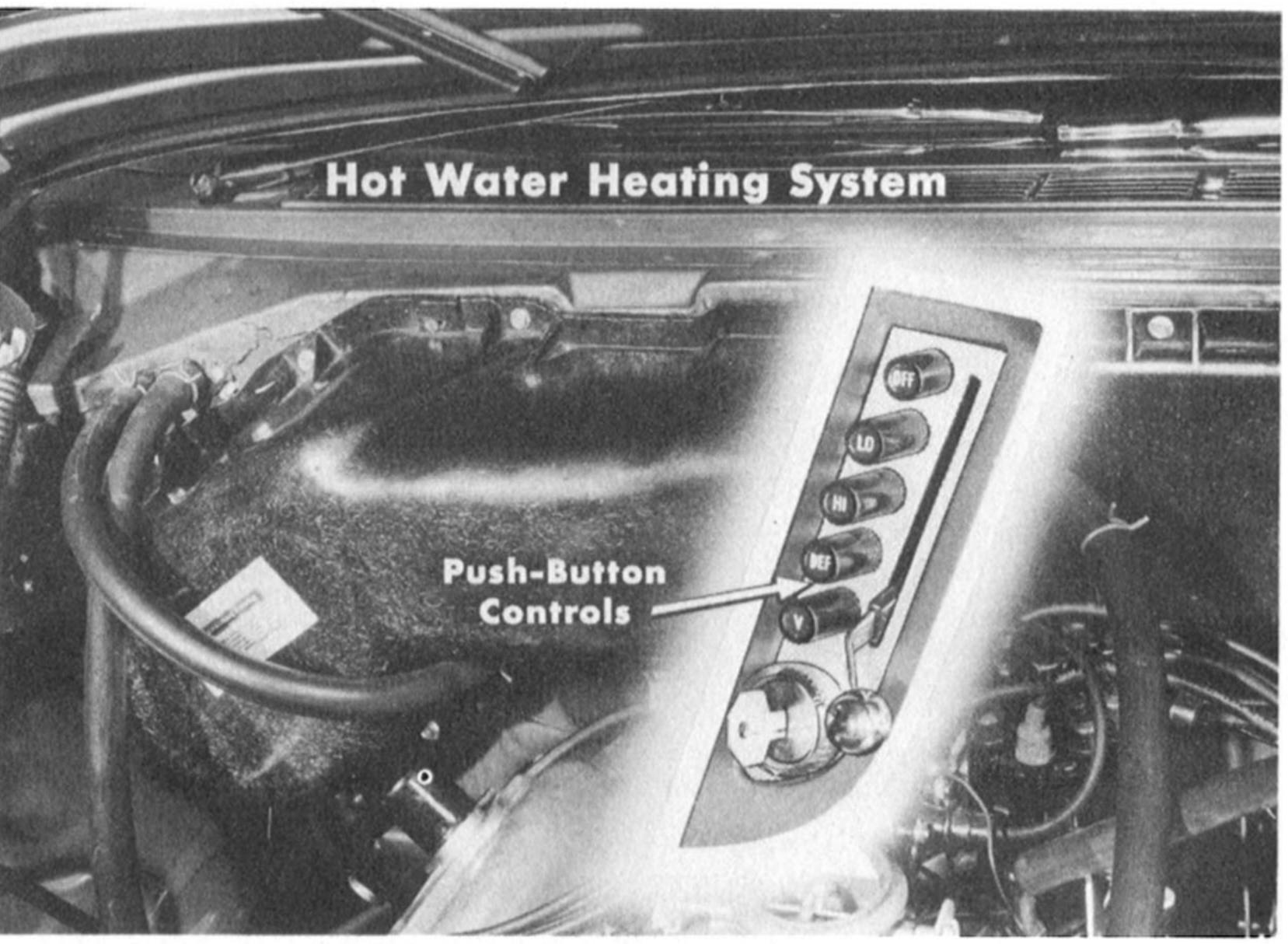
The system consists of a heater core mounted in a molded plastic housing on the engine side of the dash panel. A molded plastic distribution duct is mounted on the passenger side of the dash panel, and contains the single electric motor and the blower fan, as well as the shutoff door and the distribution duct damper. A water flow valve controls the flow of water through the heater core and thus controls
