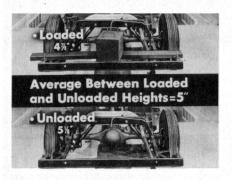
between loaded and unloaded heights. The average between 4%" and 51%" is exactly 5". Specifications call for 4%", plus or minus %" on all models but the Imperial. Imperials should be 4%" with the same tolerance. The average of 5" in this example is too high, so the valve would need adjustment. Here's how that's done.
