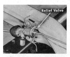
An air-sprung car, though, will take a load equal to the weight of nine average-size people. This is about 1200 to 1500 pounds, maximum. But overloading won't damage the system. It will trigger a relief device in the control valve, which is set to blow off at about 150 psi.
