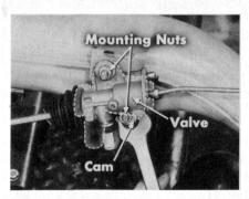
wise direction. This will enable the valve to reduce the controlled height. Hold the cam while you tighten both mounting nuts to exactly 100 inch-pounds. Do not get them any tighter. Then go through the complete loaded and unloaded checks to see if the valve is now controlling the springs at the proper height.
