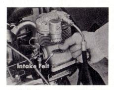
Check Intake Felt. About every 5,000 miles, check the air compressor intake felt. If it's dirty, replace it. This keeps the air clean and prevents clogging of compressor and control valve passages.
