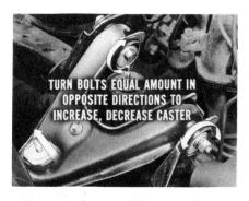
Turning each bolt an equal amount, but in opposite directions, moves the ball-joint end of the upper control arm fore or aft. This increases or decreases caster.
