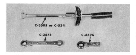
**Use Special Tools Available.** On most models it is impossible to put a torque wrench on the adjusting bolt nuts. So, you'll have to use the C-3005 or C-524 torque wrench, and this new C-3675 ratchet tool. With that combination, a torque reading of 45 foot-pounds on the wrench will be the same as the specified torque or 65 foot-pounds at the nut.
