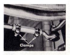
cause any interference. In addition, position the ends of the tie rods in the sockets so that both studs are against either the front or back sides of the sockets, then tighten the clabolits from 10 to 15 foctpounds. This provides sufficient angular rotation of the tie rod on the ball studs and prevents interference on extreme turns.
