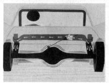
single spring of large capacity. Pressure in both air springs is always equal. If an owner tosses all his gear and heavy luggage on one side of the trunk or rear seat, such a severe one-sided load will not be leveled out. The system is just intended to keep the rear level with the front.
