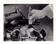
take a tip from the gas man who often traces leaks. Brush liquid soap over all seams, joints, connections, the drain valve, air springs and seats, and the height control valve mounting. When the engine runs and the system's full of air, any leak will show in the form of a bubble at the escape point.
