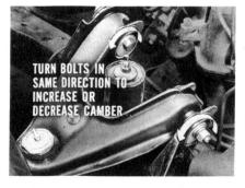
Turning both the front and rear adjusting bolts an equal amount in the *same* direction moves the upper control arm in or out. This increases or decreases *camber*.
