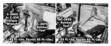
On some Chrysler cars equipped with several accessories, you'll have to use a shorter C-3696 ratchet tool. When you use this tool, you tighten the lock nut to a torque reading 55 foot-pounds on the wrench to get the specified 65 foot-pounds at the nut.
