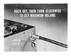
Again . . . be sure to make this adjustment on dual antenna installations. This is also important on touch-tuner radios where signal strength has a significant effect on over-all efficiency of the receiver.
