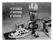
jar the instrument panel with the heel of your hand. If jarring causes more noise, there's probably a loose connection. To track it down, wiggle the power input plug, the speaker plug, and the antenna connector. Make sure the set doesn't have a loose mounting which would cause a poor ground.
