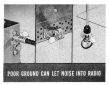
A poor radio ground can also let ignition noise interfere with reception. So check the connection between the antenna lead-in and receiver receptacle. Check the ground between the radio mounting and instrument panel. Also, make sure the anteena mounting nut is tight.
