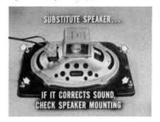
torn speaker cone, foreign material touching the cone, or a defective tube. If there are foreign particles (dust, metal chips) in the core, remove them with a vacuum cleaner. If none of these causes are found and the spare speaker doesn't improve the sould, substitute tubes.
