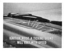
If you hear ignition noise, check the condenser connections at the ignition coil. They must be clean and tight. If connections are okay, substitute the spare, pre-tested coil condenser to see if the ticking disappears.
