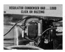
If the generator regulator condensor is bad, or has a poor connection, it may cause a loud "click", or a buzzing sound when the regulator operates. You can check this by substituting the good condenser from your test group.
