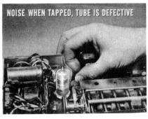
If none of those connections are loose, but you still get noise when you jar the set, remove it and hook it up on the bench. Then, with your finger tip, gently tap the tubes. Now, if you hear noise when any tube is tapped, it means the tube is
