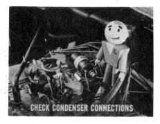
If the test condenser doesn't correct ignition noise, a loose hightension wire is the most common cause. Also, check connections at the distributor cap, coil, and at the spark plug terminals. If these are okay, check the secondary cables for continuity.
