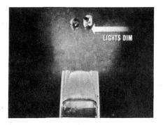
Mid-point between the two marks should be directly ahead of the scanner. If it isn't, ream the holes in the instrument panel with a 5/32" drill so the scanner unit can be relocated.
