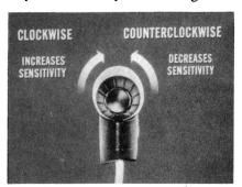
should, or dim when the approaching car is too far away, sensitivity is improperly adjusted. A knob at the rear of the scanner unit mounted on the instrument panel lets you adjust sensitivity. Turning the knob clockwise increases sensitivity — counterclockwise decreases sensitivity.
