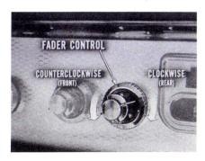
If you find the original antenna okay, suspect the speaker next. Radios with rear-seat speakers are easy to check. Just turn the fader control clockwise to check the rear speaker — counterclockwise to test the front speaker. If one works and the other doesn't, the set's okay, but one speaker is dead, so replace it.
