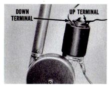
the motor runs freely, but the antenna doesn't extend or retract, replace the mast assembly. If the motor labors and the antenna moves very slowly, look for excessive dirt or bent mast rods. Clean and straighten rods that you find in this condition.
