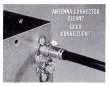
If the radio works, you'll know the difficulty was with the original antenna. However, make sure you don't throw away a good antenna assembly. See that the antenna connector is clean and makes a good connection. Corrosion there will make any antenna look bad.
