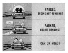
the condition. If not, find out when the noise takes place. In other words . . . determine whether the noise takes place when the car's parked and the engine isn't running. Then, see if the noise shows up when the car is parked and the engine is running. If not then, see if it shows up only when the car is out on the road.
