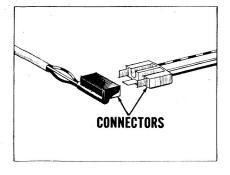
stepping on the foot switch will not change the headlight beam. Be sure to check these connections to see that they are tight. Tape the wires to the connectors, if necessary. You can use a trim panel retainer to keep the two connectors from working loose.
