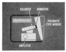
The solenoid attracts an armature attached to the prismatictype mirror, tipping it forward at the top. Glare is then directed overhead, leaving a dim, no-glare reflection for the driver. When glare behind the driver goes away, the mirror automatically repositions.
