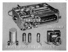
Only 12 volts are needed to operate tubes, resistors, and condensers of a transistor-powered radio. Operating at so low a voltage results in longer parts life. The transistor itself has an almost infinite service life. And, the transistor-powered radio requires less warm-up time.
