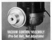
tion timing according to throttle opening at light load operation, and prevents too much advance under heavy load conditions. On the new distributor, the vacuum control assembly comes as a precision, pre-set unit. It is sealed when made, and is not adjustable.
