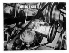
Run the engine until it warms up to normal operating temperature and set it at slow idle speed. Connect a timing light and check the ignition timing. The timing light should flash the instant the mark on the pulley is opposite the 10° BTDC mark on the timing chain case
