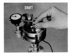
Move the shaft to and from the indicator with just enough pressure to measure movement. Too much pressure will spring the shaft and cause a false reading. If there's more than .008" total movement, replace the shaft and the bushings.
