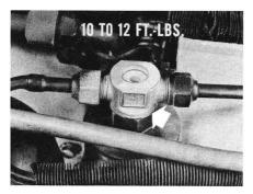
Always use new copper gaskets when you reconnect brass to steel, or steel to steel connections. And when you replace the receiver-drier, be sure to use the new gasket that comes with the drier. Torque the new drier-to-dry-eye connection 10 to 12 foot-pounds maximum.
