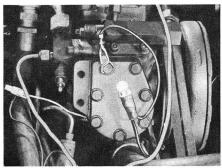
The compressor clutch should be engaged and the system should be working. If the clutch didn't engage, you'd have to use a test light to check out the compressor clutch circuit. Check contact of the brushes at the clutch, and replace worn brushes.
