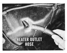
Temperature Control Valve Check. Even though the temperature control valve seems to be properly operated by the cable, it is well to check the valve itself. Momentarily, disconnect the heater outlet hose at the top of the heater housing. If there is just a small amount of water, but no con-
