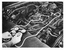
fold valves alternately. That will purge air from the hoses between the compressor and manifold. Next, read the pressures on the gauges. If the car has been parked inside long enough for all parts to reach room temperature, the pressures registered on the gauges will agree with those shown in the following table.
