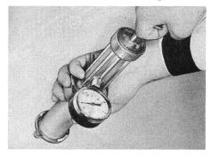
Then check the dry eye for color. If it is *blue*, the system is free from moisture. Pink, or an orchid color means moisture is present. This, of course, will call for purging the refrigerant, replacing the receiver-drier, and recharging the system.
