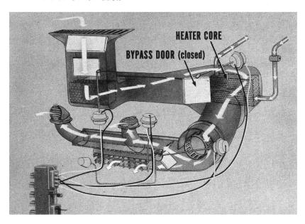
Air Flow—Defrosting. When defrosting operation is desired, you slide the control lever toward the "WARMER" end of the slot, and push the "DEF" (defrost) button in. This closes the heater bypass door. All outside air entering the opened fresh-air door is then directed through the heater core. Most of the heated air is discharged through the panel outlets to keep the windshield clear.
