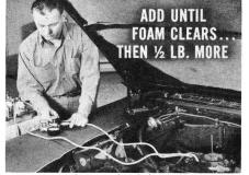
If you notice foam, it means the system is low on refrigerant. In this case, maintain discharge pressure at 225 to 250 psi and add refrigerant gas through the suction side until the foam clears. Then add exactly ½ pound more.
