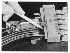
If a tighter fit on the hose connector plug doesn't bring vacuum drop within limits, remove the plug from the switch. Insert the test prod alternately in the connector block holes—first in the four holes in a row, and then in the two outer holes of the row of three. Watch the test gauge and if it comes back to 8 inches after each actuator operates, it proves the hose and actuators are okay, but the control switch is faulty and must be replaced.
