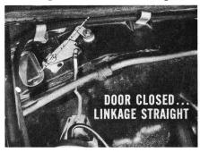
button, the bypass door should be closed, and the over-center lever and linkage (visible in the engine compartment) will be in a straight line. If the bypass door doesn't close completely, the linkage may need adjustment, or vacuum hose connections at the actuator may be reversed.
