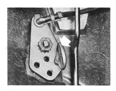
Cool-Down Test. With the car windows still open, move the temperature control lever to "OFF". Adjust the distribution duct damper control stop (or the cable, if the car is so equipped), so that it will direct 50% of the air through the panel outlets, and 50% through the floor outlets.
