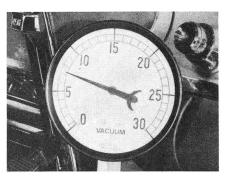
First push in the heat button. The vacuum gauge will read lower until the actuator works—and then it will build back up. Try all the buttons, and allow time for vacuum drop and build-up. You shouldn't get a vacuum drop of more than <sup>3</sup>4-inch of vacuum below 8 inches.
