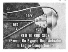
Inspect and correct any binding, misalignment, or maladjustment of the recirculating and fresh-air door connecting linkage.
