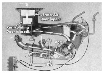
Air Flow—Fresh-Air Cooling. When the "FC" button is pushed in, the fresh-air door is opened, the recirculating door is closed. This pulls fresh air in, conditions it, and discharges it from the panel and floor outlets in the same 90%-10% amounts you get in the maximum cooling setting.
