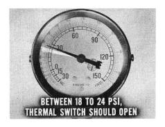
As the evaporator cools down, suction pressure should gradually lower. In fact, when suction pressure is between 18 and 24 psi, the thermal switch contacts should open and deenergize the clutch.
