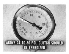
After the contacts open, suction pressure should rise rapidly. When it goes above 24 to 30 psi, the clutch should be energized again. Run the system several times to be sure that pressure changes and clutch engagements take place continuously.
