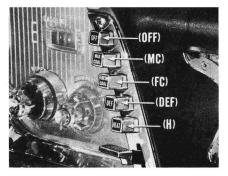
Push Buttons. As a reminder, the button marked "MC" is pushed when maximum cooling is desired. "FC" supplies fresh-air cooling. "DEF" provides defrosting, "H" is the heater button, and "OFF" turns the unit off.
