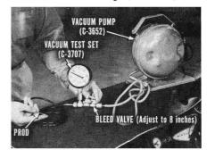
Release your finger on the hose prod a few times and reblock it. The bleed valve must be adjusted so the gauge needle returns to exactly 8 inches when your finger covers the prod.
