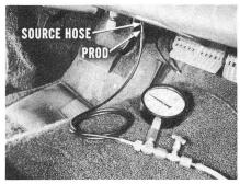
Disconnect the engine vacuum source hose at the plastic connection under the instrument panel. Insert the tester prod from the vacuum test set into the source hose that leads to the control switch.
