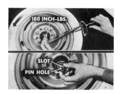
Under the new procedure, you should tighten the adjusting nut to 180 inch-pounds as you rotate the wheel. Put the nut lock over the adjusting nut so the cotter pin hole lines up with one set of slots.
