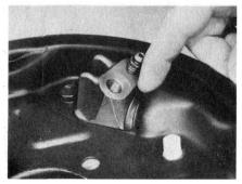
Rear Brake Cylinder. Rear brake cylinder have a more deeply machined surface at the bolting flange. In addition, there's a spot of white paint near the casting number to help you identify the new rear cylinder.
