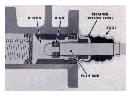
There's also a new rubber boot and boot retainer which serves as a piston stop. These new features help the master cylinder automatically maintain the proper push rod free-play. The piston stop does away with the need for any adjustment.
