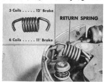
wide loop in the shoe and the spring link. The new springs have a load capacity that's 25% greater than the springs formerly used, to provide more positive shoe return. Five-coil springs are used on all 12" brakes. Six-coil springs are used on 11" brakes.
