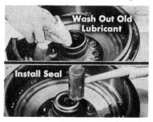
the old lubricant. Always remove the cone and roller assemblies and seals, and wash the old lubricant out of the hub. Wash the bearing, and then repack them with new lubricant. Add 1¾ oz. of lubricant to the inside of the hub. Install the bearings and the new inner seal.
