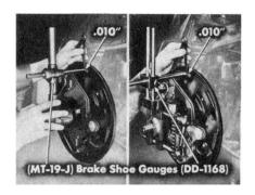
DD-1168) and a set of feelers to measure the platform height. With the dust shield installed, all platforms for one shoe should be in the same plane within .010". There should not be more than .020" width between the platform slots for one shoe and those of the opposite shoe.
