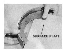
No clearance between the web and support plates can mean the shoe is bent so check web on a surface plate. Just hold the heal end of the plate, and swing the web across. Remember that the shoe cannot be straightened and will have to be replaced.
