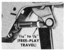
fective solid pedal of ½ to ¾ of the total pedal travel is considered satisfactory. But the brake *pedal free-play* travel should be ⅓ 16" to ⅓ 8". You can get this by lengthening or shortening the master cylinder push rod. This will provide the correct clearance of .015" to .030" between the push rod and piston.
