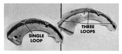
Another point . . . the new contact loops have outer edges that are *flush* with the edge of the shoe table. There is no lining overhang because the lining and table are ground at the time they're manufactured. Inner edges of the loops are formed to keep pressure from bending the loops inward.
