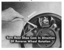
**Disassembly and Assembly.** Disassembling and assembling the platform brake are done the same way you've been handling former-type brakes. One exception, though, is removal and installation of the new shoe retainer.
