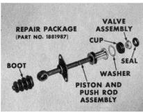
If the piston has to be replaced, install the complete Master Cylinder Reconditioning Kit (Part No. 1881987). It contains all internal parts including the piston and push rod assembly, needed for reconditioning the cylinder.
