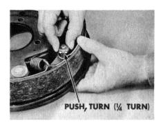
Installation is easy. Just insert the rod through the dust shield and web of the shoe. Place the inner retainer, spring and outer retainer over the rod. Apply finger pressure against the rod head. Press the outer retainer down over the rod, turn it \(^1/4\)-turn, and release.
