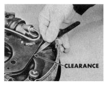
the web for signs of interference with the support plate. Any web that's flatter than specifications should align itself between the support plates. Even a web slot center will be okay because there is clearance between the web and the support plate.
