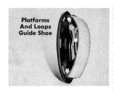
The big basic change involves the dust shield and brake shoes. Three platforms, pressed in the shields, and three loops formed on the sides of the shoes are key factors in operation. The loops guide the shoe on the platforms, and keep it in accurate alignment with the contact surface of the drum.
