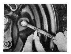
On front wheel brakes, turn the adjusting cams in direction of forward wheel rotation as you turn the wheel forward. You turn the cams to move the shoes against the drum until the wheel locks in place. Then scribe a mark in the dust shield at the leading edge of the wrench
