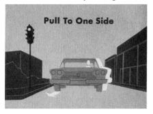
brake pull. In addition, low or uneven tire pressure can lead to brake pull. So can improper front suspension alignment, or improper front wheel bearing adjustment. All of these possible conditions can cause uneven braking and lead to pull.
