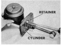
The piston, push rod, push rod ring, and boot retainer are furnished as an assembly. So they're not to be taken apart. If you have to remove this assembly, just take out the screws that hold the retainer to the master cylinder.
