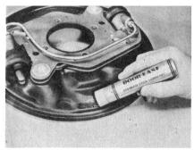
stick lubricant on the platforms, and at the heel at the ends of the shoe. It's far better to use too little lubricant than too much. At extremely high brake temperatures, loosing any lubricant is apt to turn into liquid that could contaminate the linings.
