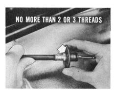
Installing the Control Cable. To install the control cable, first make sure the adjustment wheel is turned back on the control cable guide (away from the "O" ring) until only two or three threads are showing. The guide must be free from dirt or burrs so the wheel
