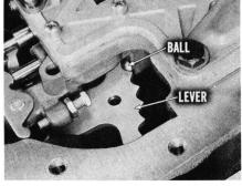
Finally, have the assistant hold the "R" button in, rock the manual valve lever back and forth. If the ball rides higher on one side of the
