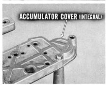
Here's something else. The accumulator cover is now integral with the transfer plate. (Incidentally, on cars using dual four-barrel carburetors, no accumulator spring is used.)
