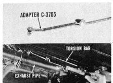
pan and the oil strainer. After that, adjust the bands. A new 6" adapter (Tool C-3705) will help simplify the kickdown band adjustment. This adapter is handy on models where the torsion bar and exhaust pipe get in the way of the standard torque wrench C-3380, and extension C-3583.
