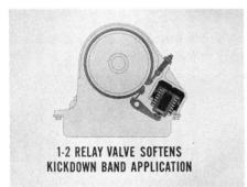
assembly, suppose we take a look at the improvement in transmission operation. As an example, let's consider the new 1-2 relay valve. This valve helps soften application and release of the servos and clutches on the upshift and downshift — particularly the kickdown band application on the 1-2 upshift.
