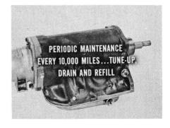
After you drain the fluid, always remove the oil pan. Clean the
