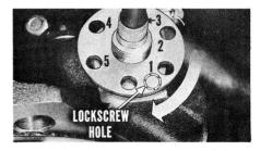
**NOTE:** If an adjustment hole doesn't line up with the lockscrew hole in the case, the next clockwise adjustment hole should be considered the "Number 1" hole. Count four more holes, making a total of five, and you will have turned the wheel the proper amount. Install and tighten the lockscrew.
