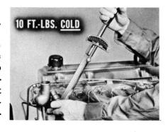
After the manifolds have been tightened to the cylinder head, make sure that the intake-to-exhaust manifold bolts are tightened to a torque of 200 inch-pounds.
