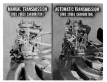
manual transmission cars a BBS-2985S carburetor is used. On cars with an automatic transmission, the BBS-2986S carburetor is used. Both carburetors use a well-type automatic choke that is connected to the choke valve by an inclined rod.
