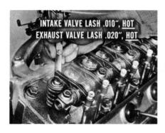
Now, with the transmission in neutral, adjust engine idle to 550 r.p.m. for cars with manual transmissions, and 500 r.p.m. for cars with automatic transmissions. Remove the cylinder head cover. With the engine hot and running, *readjust* intake rocker arms to have
