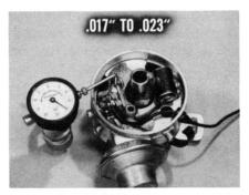
Correct ignition timing, again, is  $2\frac{1}{2}^{\circ}$  BTC. Remember to disconnect the vacuum line and plug it when you make this inspection so there won't be any advance.
