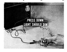
From the hinge side of the armature, insert a .048" wire gauge between the armature and the core. Push the gauge up against the nylon stops. Press the armature down against the wire core, pressing on the armature and not the stainless-steel reed which carries the contact point. The light should dim slightly.
