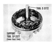
Positive rectifiers are identified by red paint; negative rectifiers by black paint. Start the new rectifier into the mounting squarely, and press it into position with tool C-3772. Solder the wire lead. Hold the wire lead with pliers while soldering it. This will help to dissipate heat, protecting the rectifier.
