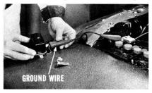
lator must have a good ground. It is better to test the regulator when it is mounted on the car. However, if a ground wire is installed between the regulator base and a good ground, it is possible to get accurate voltage readings.
