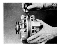
The two end frames are held together by three throughbolts. When these bolts are removed, carefully pry the drive end (the pulley end) from the stator frame, leaving the stator frame resting in the other (rectifier) end frame.
