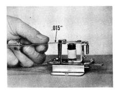
With the air gap adjusted properly, measure the clearance between the movable contact and the lower contact. It should be .015". If it isn't, adjust to this clearance by bending the lower contact bracket. Again, be careful to maintain contact alignment.
