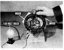
each stator winding in turn, and the other prod to the stator frame. If the lamp lights, the winding is grounded, and the stator assembly will have to be replaced.
