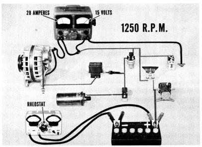
The output test is made at a specified engine speed, so connect a reliable tachometer. Also, since current output is stated at a specific voltage value, it is necessary to hold the voltage at a certain figure. Therefore, install a carbon pile rheostat across the battery terminals. If you do not have a carbon pile rheostat, use the battery-starter tester, and adjust the variable resistor in that piece of test equipment.
