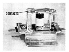
This leaves the voltage regulator as the only external conrol needed for the alternator. The voltage regulator controls the voltage output of the alternator by regulating the current supplied to the field coil of the rotor.
