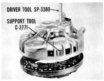
Replacing A Rectifier. If it becomes necessary to replace a rectifier, cut the lead at the point of the crimp. Support the end frame on tool C-3771, and press the rectifier out of the mounting by using tool SP-3380.
