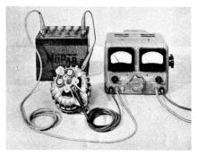
Rotor Test. An amperage draw test of the rotor field circuit can be made on the bench, before the alternator is disassembled. Simply connect one lead of a test ammeter to one terminal of a fully charged battery. Connect a jumper to the other terminal of the battery, and ground it to the
