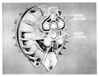
The other three rectifiers are negative—that is, they permit current flow from the battery ground terminal, through the grounded alternator end frame, through the rectifier base to the lead wire and into the stator winding, thereby completing the circuit. The negative rectifiers are pressed into the alternator end frame.
