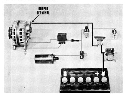
There's a connection from the field terminal of the alternator to the field terminal of the regulator. The connection from the ignition terminal of the regulator goes to the ignition side of the ignition switch. There's a 7.5-amp fuse in that lead to protect the circuit from an accidental short. The lead from the alternator output terminal disappears in a wiring harness, but it completes the circuit from the alternator to the battery positive terminal.
