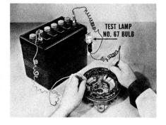
If the test lamp lights during one test, but not the other, the rectifier is good because it is allowing current to flow in one direction but not the other. If the test lamp doesn't light in either test, the rectifier has an open circuit and will have to be replaced.
