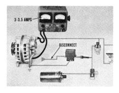
Voltage Regulator Test. This is a test to determine how well the regulator controls the alternator output. It is made after the circuit resistance test has indicated there is no more than normal resistance in the circuit, and after the current output test has indicated the alternator output is up to specifications.
