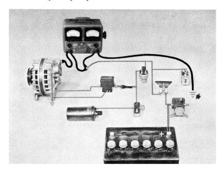
Connect the test ammeter between the alternator output terminal and the wire removed from that terminal. Connect the voltmeter between the wire removed from the output terminal, and ground. Connect the tachometer. Run the engine long enough (about 15 minutes) to be sure the charging system has become temperature-normalized. This is necessary because the voltage regulator is temperature-compensated, so the voltage reading must take temperature into consideration.
