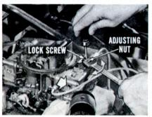
screw. Increase the engine speed to 1400 r.p.m. and note the fuel flow from the sight hole. If there is more than a trickle, the level should be reduced. If there is no flow, raise the level until a trickle is noted. Secure the lock screw. Then, install the sight plug and tighten it securely.
