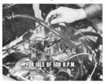
**NOTE:** On cars with air conditioning, turn on the compressor to put a load on the engine. Then adjust the idle air-speed screw for an engine speed of 550 r.p.m.
