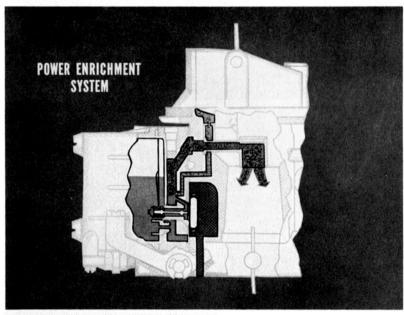
Manifold vacuum is sensitive to engine power demands. At idle, when the throttle valves are closed, vacuum is strongest. As engine load is increased, the throttle valves must open wider to maintain a given speed. That reduces vacuum because the opened throttle valves offer less restriction to the air entering the intake manifold.
