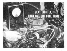
Idle Air-Speed Adjustment. Use a narrow-blade screwdriver to reach the idle air-speed screw at the bottom of the air cleaner anchor stud hole. Turn the screw in *lightly* against its seat, then back out one full turn. Readjust the screw as needed to get an idle speed of 500 r.p.m.
