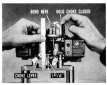
Choke Unloader Adjustment. Use your finger to hold the choke valve lightly closed. Then, open the throttle valves to wide-open position.
