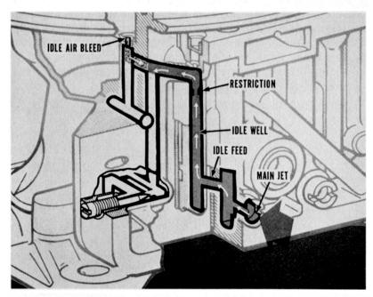
Because both sides of the carburetor work very much alike, flow of fuel on only one side will be described. At engine idle speed, normal air pressure causes fuel to flow from the bowl through the main jet, and into a small angular passage called an "idle feed". The main jet and idle feed are both in the primary metering body.
