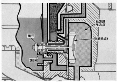
Accelerating Pump System. On acceleration, air flow through the carburetor increases quickly as the throttle valves are suddenly opened. To maintain proper balance of fuel and air, an accelerating pump supplies an extra charge of fuel until the main metering system can step up an increased flow.
