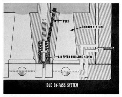
As we mentioned before, fuel enters the throttle bores below the throttle valves. Even though no air flows past the throttle valves which are closed completely during curb idle, air does enter the idle bypass through a port between the primary venturis. It then flows past the curb idle air speed adjusting screw. From there, it goes down through a cross groove at the bottom of the carburetor where it mixes with the fuel going to the combustion chambers.
