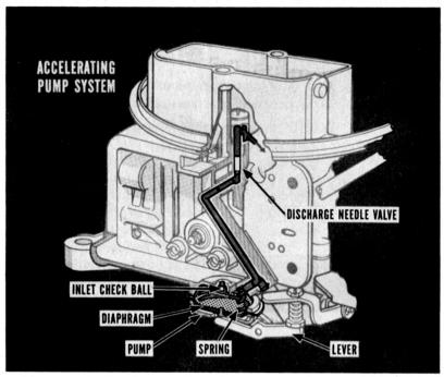
The accelerating pump used on this carburetor is a diaphragm-type, located on the bottom of the primary fuel bowl. It goes to work when the pump operating lever is actuated by the throttle opening. As the throttle opens, pump linkage, actuated by a nylon cam on the primary throttle shaft, forces the pump diaphragm up against spring pressure. Diaphragm pressure forces a pump inlet check ball onto its seat to keep fuel from going back to the bowl.
