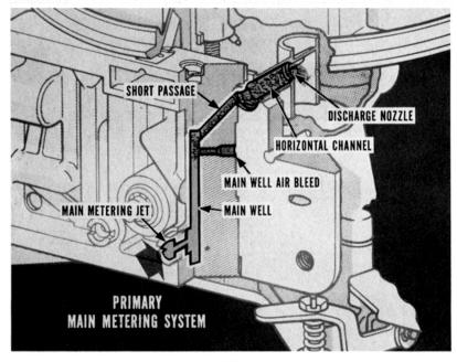
Fuel from the bowl flows through the main metering jet and into the bottom of the main well. It then moves up the well and past the main well air bleed. Filtered air from the bleed mixes with the fuel.
