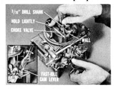
Fast-Idle Adjustment. Proper fast-idle adjustment is necessary to keep the engine running during pre-warm-up. So, invert the carburetor and close the choke and throttle valves completely. Place the fast-idle screw in contact with the high step of the fast-idle cam. Turn the
