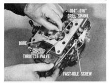
screw in or out until you can insert a .014" to .016" drill shank between the primary throttle valve and side of the bore toward the center of the carburetor. Turn the screw in until the drill shank is held tightly. Then, back it off until you can feel a slight drag as you remove the drill.
