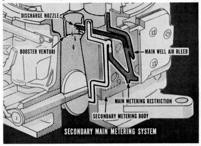
Fuel in this system enters the secondary metering body through the main metering restriction. It moves up a vertical passage where it mixes with air from the main well air bleed. From there it moves into the discharge nozzle. It is then discharged into the booster venturi and air stream.
