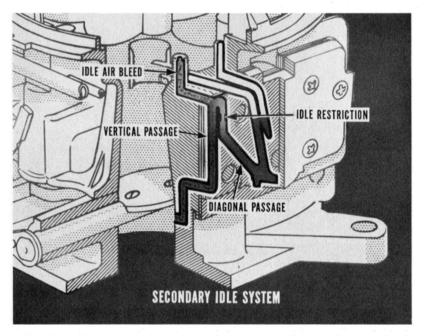
Fuel, in this system, flows through main metering restrictions which are used in place of jets. The fuel goes up a diagonal passage and through an idle restriction in the secondary metering body. It flows past the idle air bleed, picks up air, and flows down a vertical passage in the main body.
