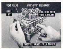
if you can insert a .050" to .070" drill shank between the center of the vent valve and the float bowl. If not, use Tool T-109-213 to bend the air vent valve rod at its right-angle turn to change the arc of contact with the throttle lever until bowl vent clearance is correct.
