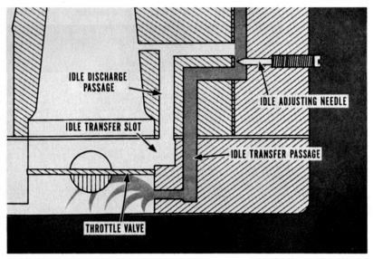
As the throttle valve opens slightly, fuel flows through the idle transfer passage from the metering body into the main body and throttle passages. Then, as the throttle is opened wider and more of the idle transfer slot is exposed to vacuum, fuel-air mixture is discharged into the throttle bore. Vacuum in the throttle body increases as the throttle opens still wider. This brings the main metering system into action to smooth out the change from idle to cruising speeds.
