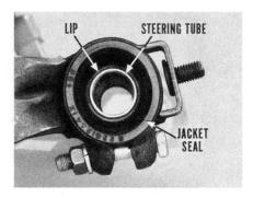
It is important that the steering tube be centered in the jacket seal, and that the lip of the seal which contacts the tube be well lubricated with wheel bearing lubricant to avoid squeaks.
