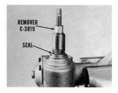
Thread the Seal Remover into the seal until it engages the metal portion of the seal. Then, turn the puller center screw to withdraw the seal from the housing.
