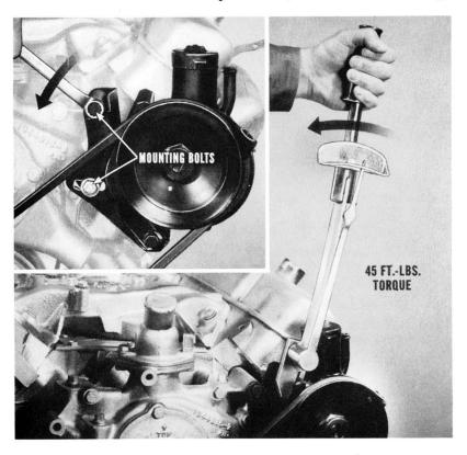
of the pump mounting bracket as close as possible to the outer edge of the bracket. Next, tighten the belt until you obtain a reading of forty-five foot-pounds on the torque wrench. Hold that tension while you tighten the bracket mounting bolt nuts to hold the adjustment.
