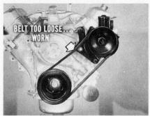
If the belt tension was originally adjusted too loosely, or the belt was stretched after a lot of service, there may be a squealing noise from the belt, or a slight knocking noise caused by the bracket vibrating against the rubber stop.
