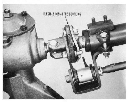
You'll notice the coupling, which looks and acts very much like a certain type of universal joint, is located just above the chuck. The coupling is made up of a flexible disc sandwiched between two steel hubs. The lower hub of the coupling is attached to the worm shaft by a serrated connection and clamp bolt. This shaft, which extends from the chuck, has a master serration which lines up with an index mark on the outside of the lower hub.
