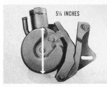
While the new pump is the same basic slipper-design as used formerly, the pump is of larger capacity and the individual parts are not interchangeable with the former pump. For example, the diameters of the reservoir and the mounting flange are increased from 45%" to 51%".
