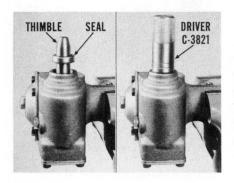
To install the seal, first place the Thimble over the serrations on the worm shaft to protect the lip of the seal. Then, carefully drive the seal into the housing until it stops against the counterbore.
