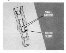
truck models. The replacement pump is furnished with the orifice sleeve positioned so the *small* orifices are in line with the flow of fluid from the rotor—as required for passenger car installation. The upper set of orifices is blocked off because of the position of the sleeve.
