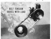
creased automatically to prevent belt slippage. Since most belt slippage and consequent wear takes place when the pump is under heavy load, the automatic tension take-up reduces the slippage, thus increasing belt life and resulting in fewer belt adjustments.
