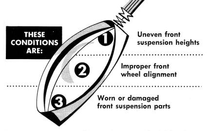
**Front Suspension Heights.** Incorrect front suspension heights, due to improper torsion-bar adjustment, can impose an extra load on one side of the front suspension. This would have a definite effect on steering control, and might lead the technician to blame the steering gear adjustment.
