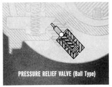
Pressure Relief Valve. The new pressure relief valve is a ball-type valve instead of the disc-type valve formerly used, and is serviced as an assembly. The valve is supplied in three different capacities, and each valve is marked on the hexagon section for easy identification.
