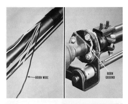
Steering Column Bracket. A new steering column bracket is used at the lower end of the jacket to secure the jacket to the dash panel. There are two different types used—one for cars using standard brakes and another for cars using power brakes.
