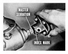
Position the clamp bolt hole in the coupling hub in line with the radial groove on the worm shaft, and install the bolt and lock washer. Tighten the clamp bolt to 30 to 35 foot-pounds.
