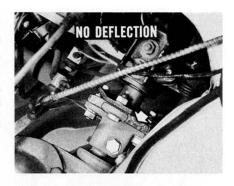
While holding the jacket in position, tighten the column bracket stud nuts at the dash panel and the column clamp to 100 inch-pounds torque.
