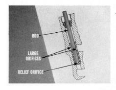
The sleeve may be positioned deeper in the passage by using a length of ½-inch round steel rod to drive it down to the bottom of the counterbore. Be sure there is a slight chamfer on the end of the rod so you don't damage the relief orifice in the lower end of the sleeve.
