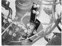
Jacket Clamp. In addition, cars equipped with manual transmission use a new stamped jacket clamp in place of the die casting type formerly used at the lower end of the gearshift tube. This clamp offsets the lower end of the gearshift tube from the jacket, toward the engine. This arrangement provides the necessary clearance between
