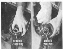
separator, in the jacket with the radius on the inside diameter of the bearing facing downward. See that the bearing seats squarely on the three supporting lugs in the jacket. Then, press it firmly into place. Next, place the washer, part number 2201299, on top of the bearing.
