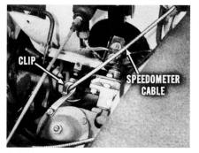
see that the end of the clip is properly bent over to secure the cables. On early models without the clip, it might be advisable to install one to assure the proper clearance. You can make a clip that will do the job—just be sure to wrap it with tape so it won't chafe the cables.
