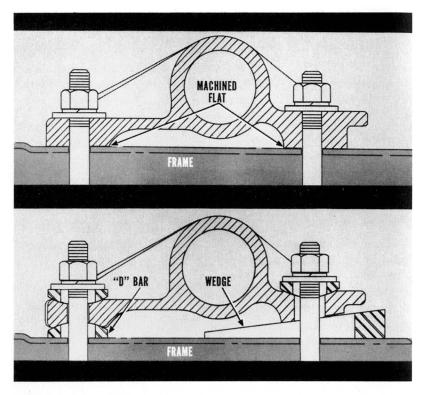
The new steering gear provides several benefits for both the car owner and the service technicians. First, the flexible coupling reduces the transmission of road shock and noises into the car. Service technicians like the new gear because the new mounting and the flexible coupling make the job of aligning the gear and steering column much easier and more positive than with the former unit.
