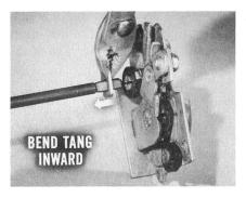
To guard against control rod disengagement, bend the tangs on both latch mechanisms inward (toward the tailgate center). Then, check control rod operation to see that rod ends will stay in place.
