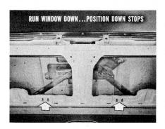
Loosen the lower stop screws near the bottom of the gate. Lower the glass until the top of the frame is even with, or slightly lower than the top of the tailgate outer panel. Hold the stops against the glass frame, and tighten the screws to limit the downward travel of the glass.
