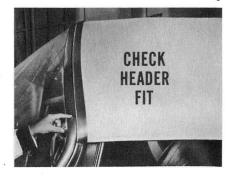
If it is necessary to re-position either side of the folding top header, remove the door glass weatherstrip and retainer from the roof rail to
