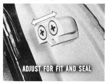
each time it is closed, and releases easily when operating the latch handle. You may need to move the strikers more than once. If necessary, you can add or remove shims behind the strikers to improve rotor engagement.
