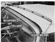
Apply cement to the top fabric and to the top surface of the weatherstrip. Then install the 1½" x 62" strip of waterproof tape. Be sure to cover all the staples and tabs so there is a waterproof bridge from top material to header weatherstrip, to provide a good seal.
