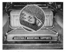
Third Seat Adjustment. On three-seat suburbans, the third seat back and cushion also have adjustable mountings and supports. By loosening the bolts, you can move the mountings to get a more level cargo-carrying surface whenever required.
