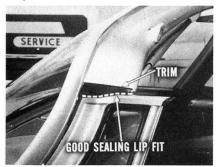
remove all the old sealer. Also, clean the seal to remove any powder on the exterior. Apply cement to the body pillar and the seal. Let it dry until tacky, then press the seal into place. In some cases you may have to install a new seal to stop a leak at the upper edge of the vent wing frame.
