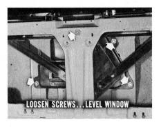
Run Channel Adjustment. The easiest way to align the tailgate run channels with the body run channels is to use the glass as an alignment fixture. So, loosen the run channel attaching screws at the top and bottom. Close the tailgate. Raise the glass to within about a half-inch of the top, and this will align the
