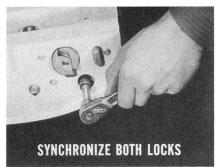
action of both locks to see that both rotors release at the same time. This can be adjusted, if necessary, by an adjusting screw reached by removing a rubber plug in the end of the tailgate. Adjust the action to take up the lost motion in the lock levers so both rotors will release at the same time.
