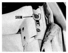
NOTE: In some cases it may be necessary to rotate the leading edge of the top header downward to improve sealing... particularly at the outer ends of the header. The top header can be rotated by inserting a spacer approximately ½" thick between the side rail and the windshield
