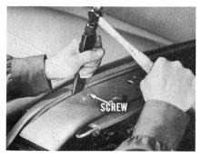
the outside side molding and upper windshield header molding. If necessary, rework the end of the side molding to reduce the step-off by reforming the fillet after installing the additional metal screw. After the lap joint gap is eliminated, wipe sealer into the joint.
