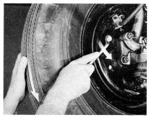
Starting at the right front wheel, turn the adjusting cam on the front shoe in the direction of the front wheel rotation when the car is moving forward, and rotate the wheel slowly. Turn the cam until the shoe lining is solidly against the drum, and the wheel is locked.
