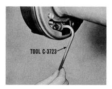
Next, expand the shoes outward against the drum until a slight drag is felt. Because of the limited access to the adjusting screw, use of Adjusting Tool C-3723 will make the job easier. Then, back off the adjustment one notch, or until the drum is free.
