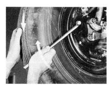
Then, back off the cam until only a *very slight drag* is felt, as you turn the wheel in forward direction.
