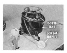
A recommended procedure to overcome this possibility is to always use Brake Bleeder Tank C-3496 and Adapter C-3494A, or their equivalent, whenever bleeding the hydraulic system. A bleeder tank will always give the right amount of bleed pressure and the proper steady flow of brake fluid through all the lines to force out all air bubbles.
