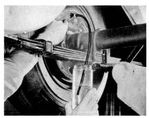
brake fluid. Use a *clean* glass jar. Pour in enough Chrysler-approved brake fluid to be sure the opposite end of the bleeder hose will be covered by the fluid. This will enable you to detect any trace of contaminants, such as mineral oil or water, as the fluid is expelled.
