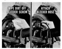
at that location. The reason for starting at this location is that the long lines to the rear cylinders generally contain about three times as much air as the short lines, and it is essential to remove these bubbles first to obtain a firm brake pedal.
