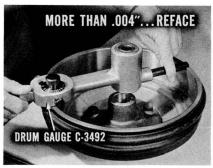
out of round should be refaced. If removing more than .030 inch on one side, or .060 inch on the diameter is necessary to true up the drum, it should be replaced. If too much metal is removed from a drum it will tend to distort under load, particularly on hard brake applications, when high temperatures are developed.
