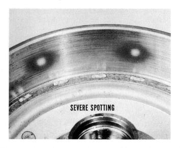
This type of spotting cannot be removed by turning on a drum lathe because the metal is too hard. Grinding is required. However, grinding should be limited to .030 inch on a side or .060 inch on the diameter. If the removal of more than this amount of metal is required, the drums should be replaced.
