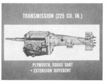
tion it carries the parking brake. The Plymouth and Dodge Dart transmission also has the low gear ratio of 2.71 to 1, and the second gear ratio of 1.83 to 1. These ratios, higher than these models had last year, provide excellent breakaway acceleration.
