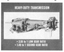
This heavy-duty transmission is also used on Dodge Trucks, and is optional on taxicabs and fleet cars. When it is used on Dodge Trucks and heavy-duty passenger cars, gear ratios are 3.02 to 1 in low, and 1.76 to 1 in second.
