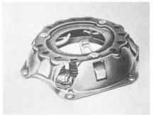
Then there is a special application of a  $10\frac{1}{2}$ " semi-centrifugal clutch. This is used when the heavy-duty transmission is coupled to the 361 cubic inch engine with a two-barrel carburetor for Dodge Polara, De Soto, and Chrysler Newport models. Clutch size goes up to 11" when the heavy-duty transmission is used on a four-barrel 361 cubic inch engine. For all 1961 clutch model applications, refer to the chart on Page 24.
