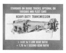
Heavy-duty features of this transmission consist of heavy-duty ball bearings at the main drive gear and mainshaft. There's also a ball bearing at the rear end of the mainshaft. The countershaft has two sets of double-row roller bearings. The reverse idler gear also has roller bearings. Heavy-duty straddle-type shift forks are used.
