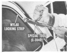
on Valiant windshields and rear windows is continued, and is extended to the Dodge Lancer models. It is also found at the stationary rear quarter glass on some models. A new special tool (C3840) is available to simplify installation of the Mylar locking strip.
