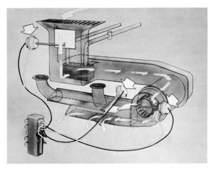
If coolant circulation is satisfactory, yet the heat delivered to the interior of the car is not, the air circulation system should be inspected. Be sure the little vacuum actuators which control the movement of the doors and damper are working properly.
