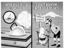
ideal engine operating temperature and the boiling point of the coolant. Water boils at a temperature of 212° at sea level. Up on a 10,000-foot mountain water will boil at about 194° because atmospheric pressure is lower at that altitude.
