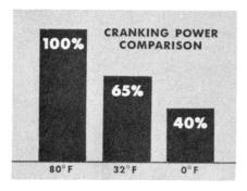
Therefore, when the battery has less than its full cranking ability, and there are undoubtedly other electrical losses along the line, it is easy to understand why there's just not enough voltage left to jump the gap at the spark plugs—and the engine won't start
