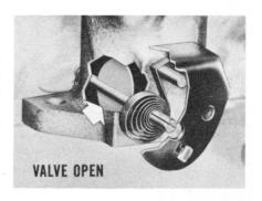
If the valve sticks in its closed position, too much heat will be directed to the carburetor hot spot. This overheats the mixture and
