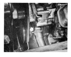
Since each of these conditions results in bubbles in the coolant, they are relatively easy to detect. Simply remove the radiator cap and watch for bubbles circulating in the coolant while the engine is running. If they are present, remove the fan belt which drives the water pump, and run the engine without the pump. If the bubbles keep coming it is evident they are produced by a compression leak.
