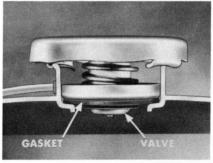
Under ordinary driving conditions there is no pressure buildup in the system. But, driving in heavy traffic, extremely hot weather, up
