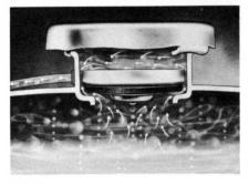
system to atmospheric pressure. Pressure immediately starts to build up in the system, and the boiling point of the coolant is raised. If pressure increases to the point where it overcomes the spring pressure against the cap pressure valve, the valve will be lifted off its seat. Pressure is then relieved through the overflow tube.
