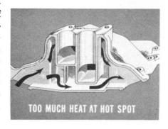
The manifold heat control valve should be lubricated regularly with solvent (Part No. 1879318) every 1000 miles.
