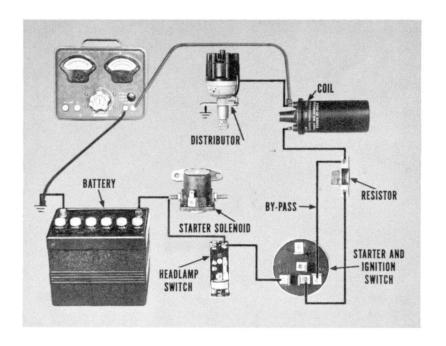
Next, remove the jumper wire and test the voltage drop between the distributor side of the coil, and ground. If there is more than .1 volt drop, look for a poor connection between the coil and the distributor points, examine the points themselves, and inspect for a good ground between the distributor housing and the engine. It might be necessary to inspect the engine ground strap to be sure it is clean and tight.
