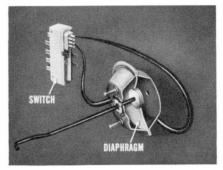
nected, split or cracked. This would cause a vacuum leak, making the actuator inoperative. The vacuum switch at the pushbutton panel could be leaking, or the vacuum actuator could have a cracked diaphragm. If the diaphragm is cracked, replace the actuator.
