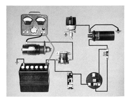
Connect the voltmeter positive lead to the battery positive terminal, and the voltmeter negative lead to the starter motor terminal.
