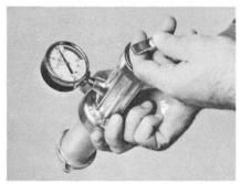
cooling system for leaks. Plug the overflow tube and attach the tester (without the cap adapter) to the radiator filler neck. The system should be tested at three pounds higher pressure than the cap. Failure to hold pressure indicates a leak in the cooling system.
