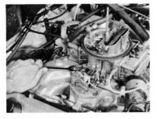
One cause of hard starting that is often overlooked is loose carburetor air horn screws or mounting stud nuts, or both. They cause air leaks which lean out the fuel mixture by the time it reaches the combustion chamber. Always tighten these screws and mounting nuts on each job.
