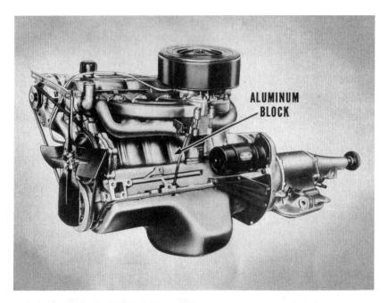
In general, the new aluminum engine is similar in design to the cast-iron engine. It can be easily identified by visual inspection, and by the engine code identification AR-22 followed by the engine serial number stamped on a machined boss next to the number one spark plug on the right side of the block.
