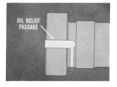
In order to test for this type of hydraulic knock, first attach an oil pressure gauge. Run the engine to bring in the knock. Then, reduce oil pressure a noticeable amount by backing off on the oil pump
