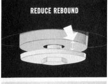
Remove the stud and turn it on a lathe to reduce shoulder height an amount equal to the measured space between the stud washer and stop.
