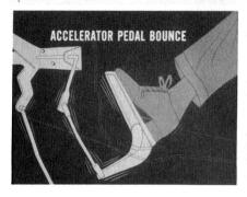
Under certain driving conditions, engine movement may cause an accelerator pedal bounce that the owner can feel through the sole of his shoe. If this pedal movement is objectionable after the engine has been properly tuned, the amount of rebound at the rear engine mount can be reduced.
