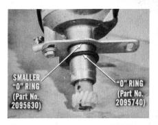
If the distributor already has a large "O" ring and is leaking, remove and discard this "O" ring. Slide a smaller "O" ring (Part No. 2095630) into the small undercut under the retainer plate. Then, install a new, large-size "O" ring (Part No. 2095740). Reinstall the distributor and set ignition timing to specifications.
