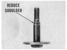
**NOTE:** Don't replace the stud with a plain bolt. This can compress the spring fully and cause misalignment between the engine and drive line.
