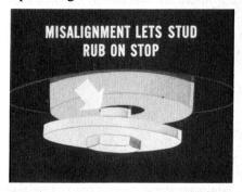
on a hoist. Then, grasp the propeller shaft near the transmission and move it up and down to see if it will bring in the noise. A squawk of this type is generally caused by misalignment of the engine mounts that lets the rear mount stud rub on the rubber stop.
