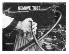
A quick test for a sticking flow valve is to remove the flexible connecting hose from the flow valve and hold your thumb over the end of the hose. If engine idle smooths out, the flow valve is probably dirty and needs cleaning. The flow valve should be serviced regularly, of course. This is particularly important on cars that are operated under short-trip driving conditions during cold weather.
