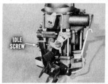
engines is occasionally a problem. That's because the carburetor has only one screw for setting both the fast and curb idle. With this setup, fast idle may be too fast when curb idle is okay. And, when fast idle is okay, the curb idle may be too slow and cause a rough idle or stalling.
