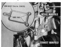
the six-cylinder engine cools. It's caused by relative movement of the manifolds at the intake-to-exhaust-manifold gasket, when the exhaust manifold contracts. This movement might even cause the gasket to creep. To prevent this noise, apply MoPar "Led-Plate" (Part No. 2275437) to each side of the gasket.
