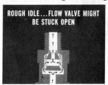
On an engine equipped with the closed crankcase ventilation system, engine idle will be rough and the engine will have a tendency to stall if the flow valve sticks in its open position. This would let excess air bleed in at idle, and lean out the fuel mixture.
