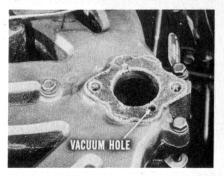
choke piston and the step-up piston vacuum ports. And if the vacuum hole in the gasket is not positioned at the hole in the manifold, there will be a rough engine idle. The vacuum hole must line up with the manifold hole provided, or an air leak will result.
