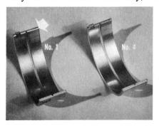
bearing insert has a greater chamfer on the inside edge at the locating tab end to provide lubrication to the timing chain and sprockets. Putting this chamfered insert in the number four position will direct more oil against the rear main seal than it can handle.
