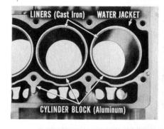
The top of the block is cast open. This permits visual inspection and access for cleaning the water jackets.
