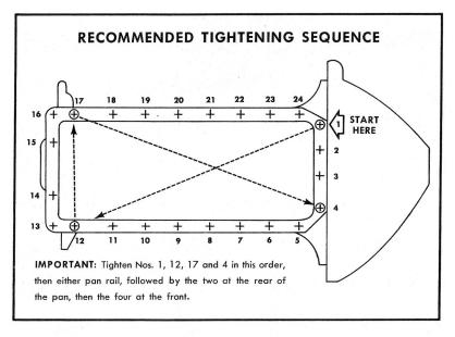
The recommended tightening sequence for oil pan retaining cap screws is shown in the accompanying illustration.
