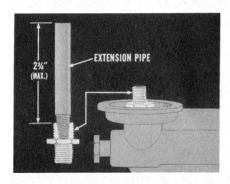
In a case like this, make an oil filter extension pipe out of ½" pipe. Install this extension to provide an oil reservoir for an added oil supply during initial engine starting. Here are the detailed steps to follow for this operation:
