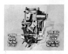
In a case of this kind, install a curb-idle adjusting screw (Carter Part No. 100-16) and spring (Carter Part No. 61-291) in the tapped hole provided. This will permit accurate curb-idle setting independently of fast-idle setting, and result in improved engine performance.
