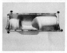
Unless the engine is jacked up and blocked that way, you won't have the working room needed — and you're apt to bend the oil pan corners. Bent corners on the pan won't seal properly and may cause an oil leak.
