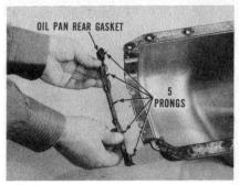
installing the new gasket on an earlier-type pan, don't be tempted to snip off any of the prongs to make the new gasket fit. Cutting off a rubber prong can cause the gasket to shift and spoil its sealing efficiency. Instead, adapt the pan to fit the new gasket.
