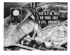
**NOTE:** When setting idle speed of engines equipped with an alternator, the bright lights should be turned on. This will impose a load on the engine comparable to that normally imposed by the heater, radio and other accessories.
