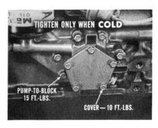
**CAUTION:** Remember . . . tighten oil pump cap screws only when cold! The aluminum and steel mating parts expand and contract at different rates.
