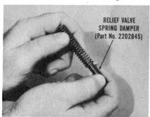
equipped with the 361-, 383-, or 413-cubic-inch engines. It's a growling, grinding or buzzing sound heard most clearly at the oil pan. You can eliminate this particular noise by installing the new-type oil pump relief valve spring damper (Part No. 2202845).
