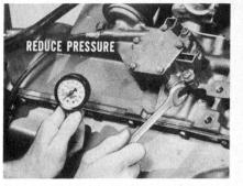
relief valve nut—or temporarily remove the relief valve spring.
