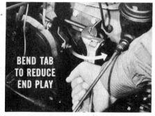
**CAUTION:** Don't bend the support bracket too much, or it will cause the linkage to bind. A slight amount of end play should remain.
