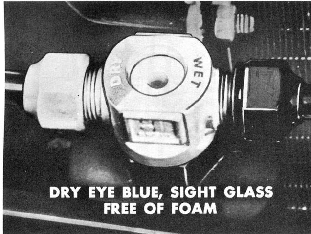
Fig. 10—Foam means low refrigerant supply
