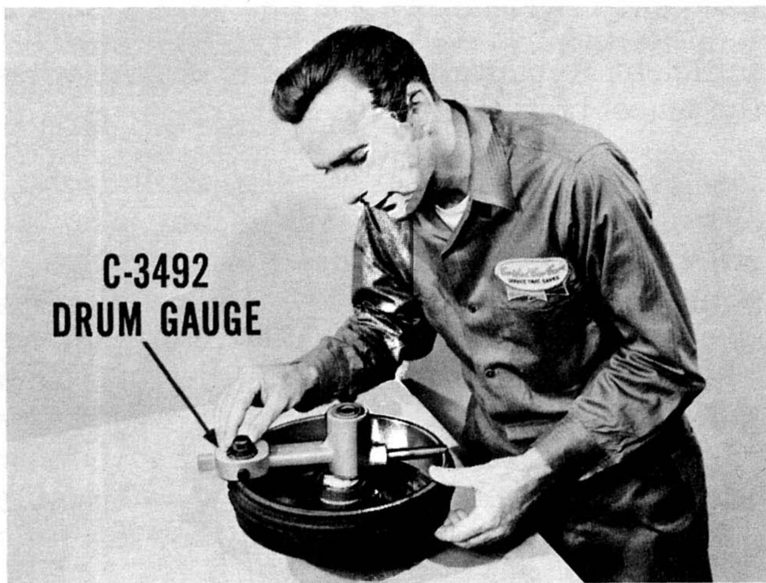
Figure 19—Measure drum with gauge C-3492
