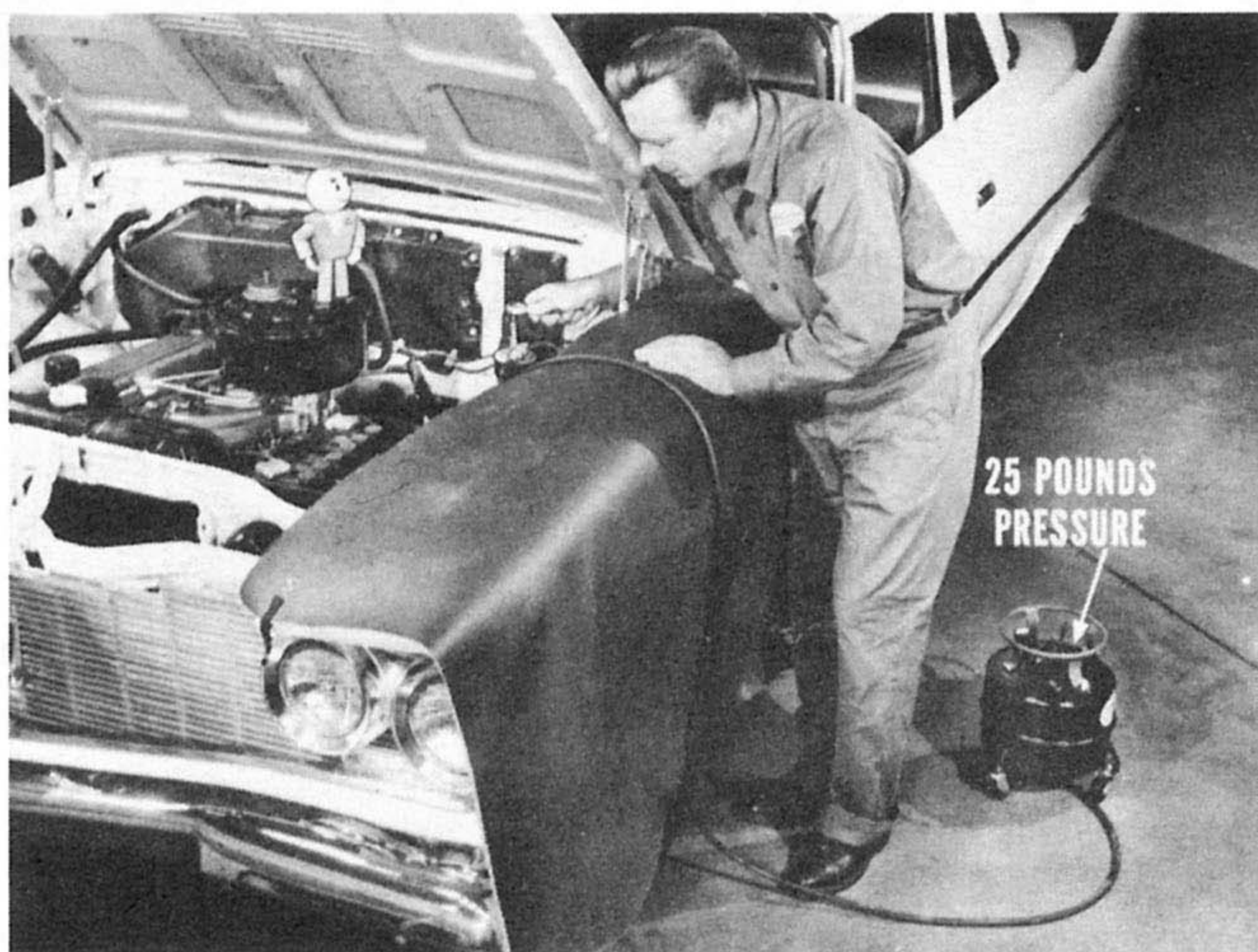
Figure 1—Use pressure tank to bleed brakes
