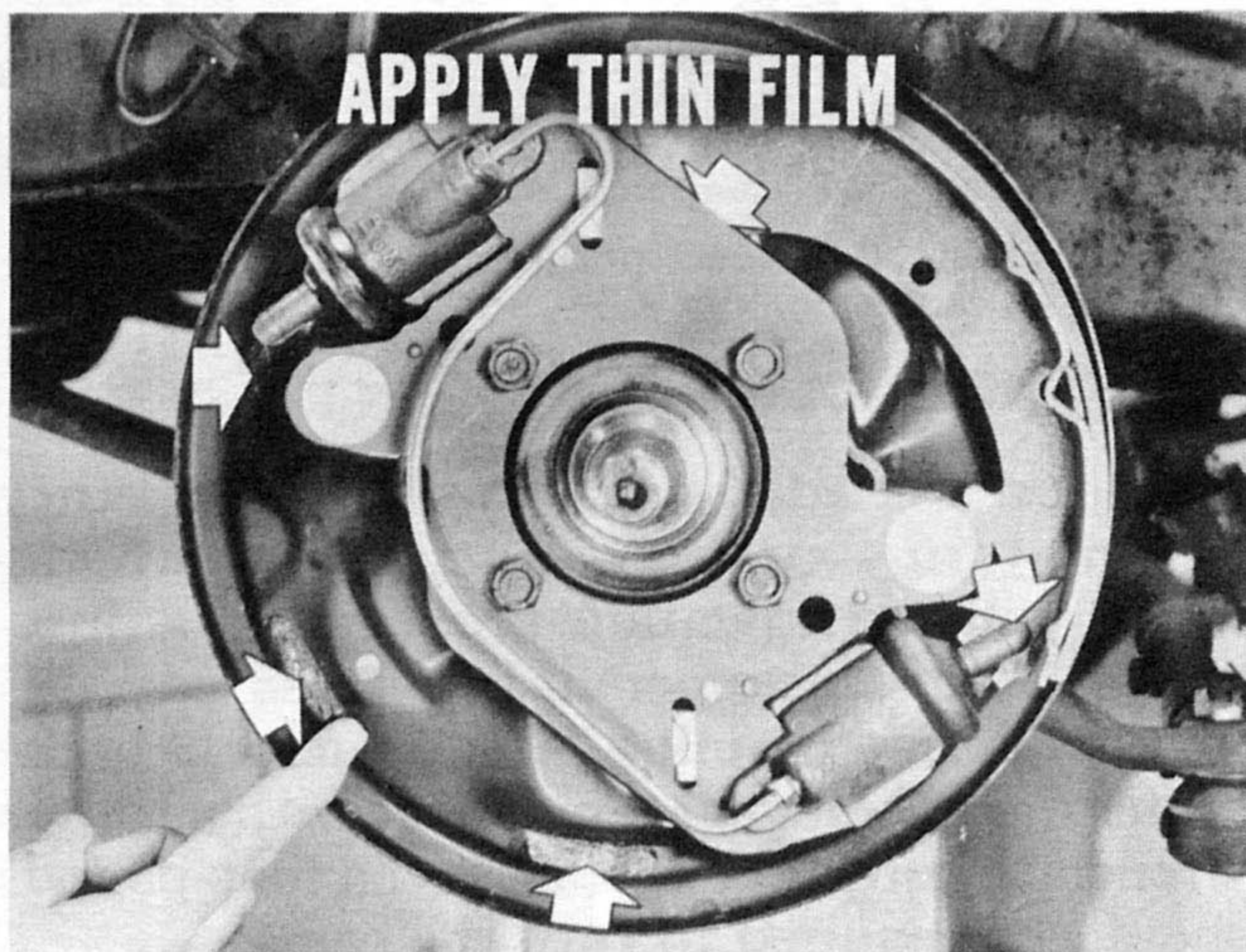
Figure 12—Lubricate shoe contact points
