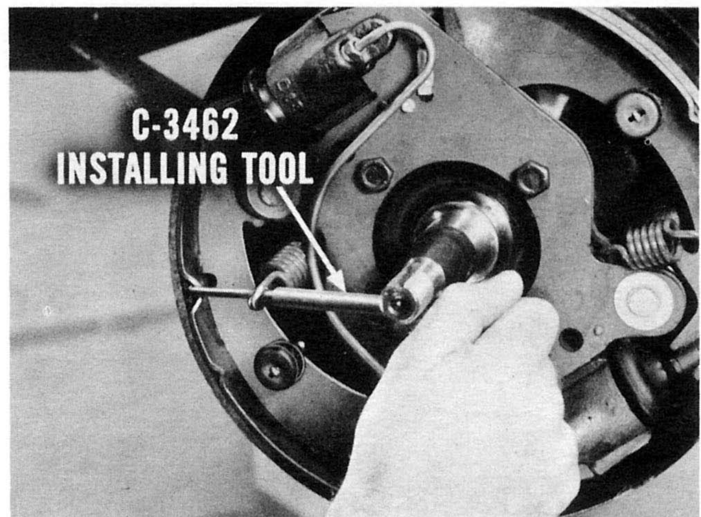
Figure 13—Use return spring installing tool C-3462
