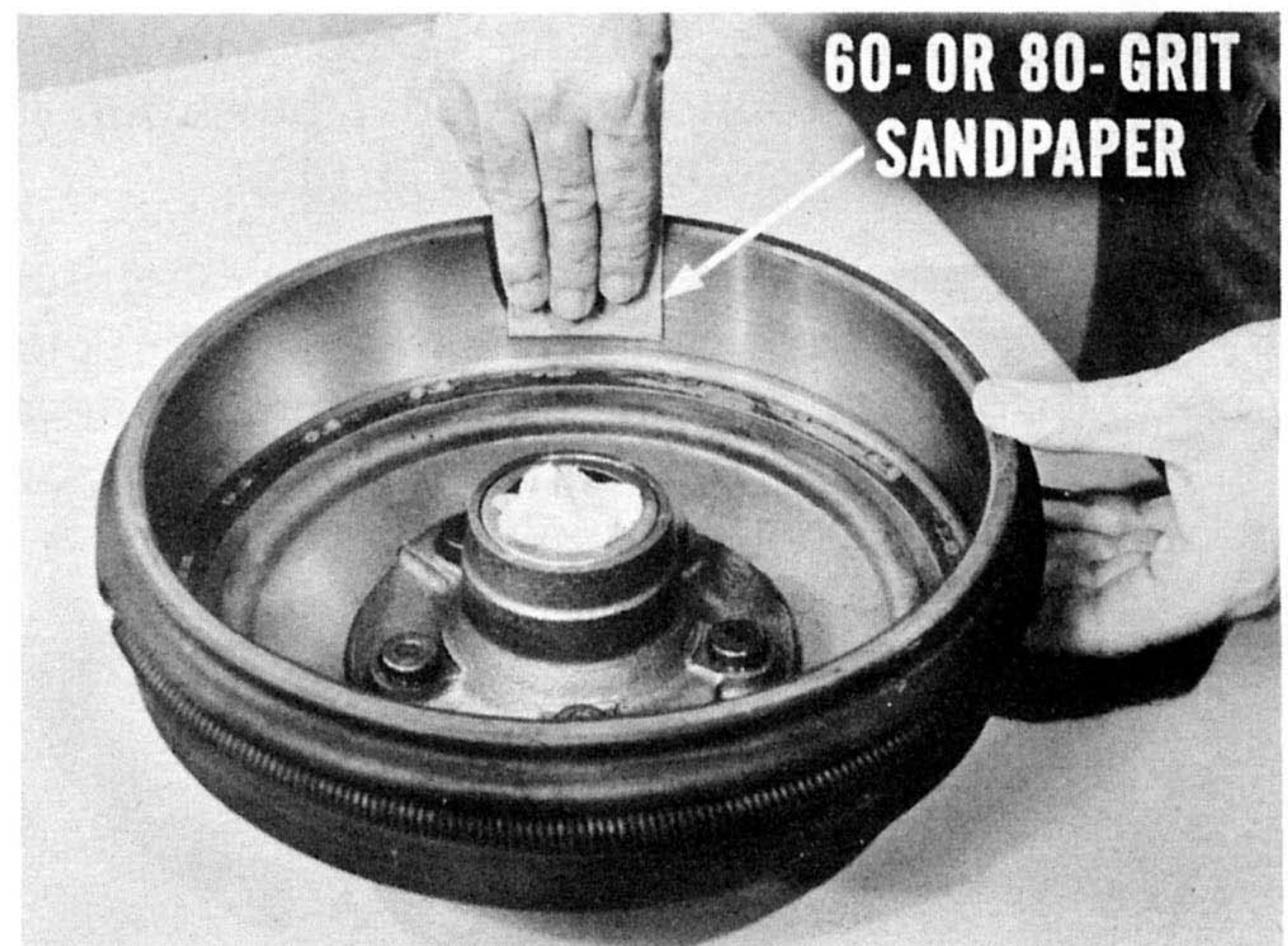
Figure 20—Rough up drum surface
