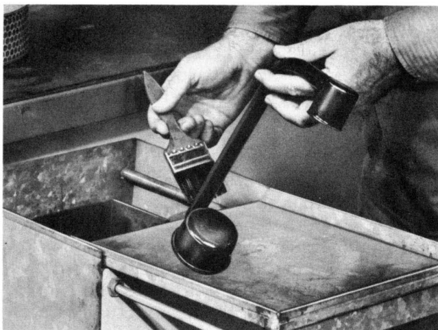
Figure 2—Clean crankcase breather pipe
