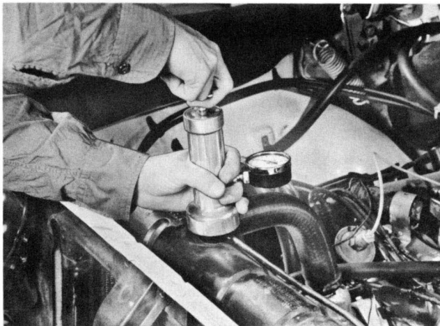
Figure 5—Pressure-testing the cooling system
